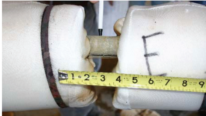
Figure 5-14. Post-test Photo of Hemyc ERFBS Showing Shrinkage at Junction
