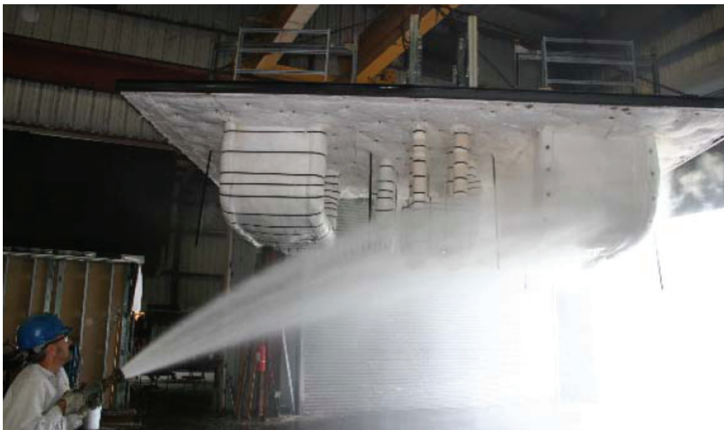
Figure G-6. Post-Fire Exposure – Hose Stream Test
