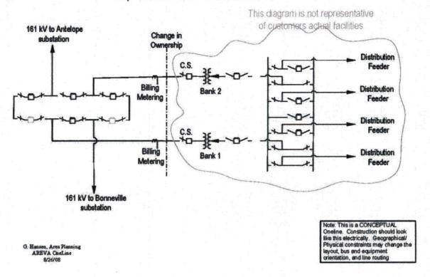
Figure 2: One-line diagram showing the proposed transmission system from Bonneville to Antelope and the new interconnect to AREVA substation.
