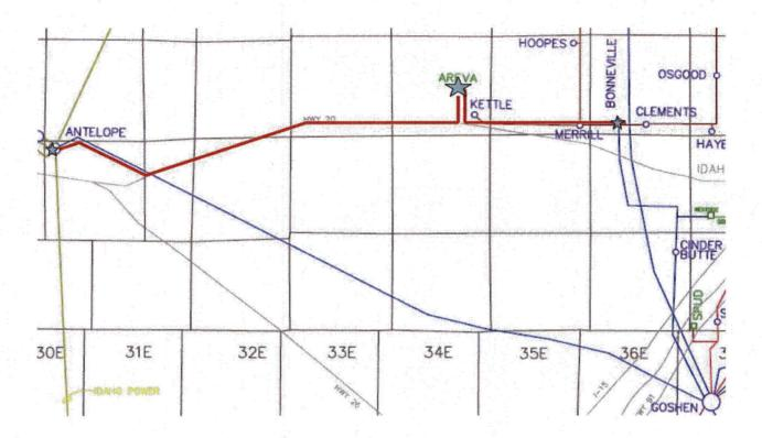
Figure 1 is a one-line diagram showing the proposed 161 kV transmission system from Bonneville to Antelope and the delivery point of the new AREVA substation.
