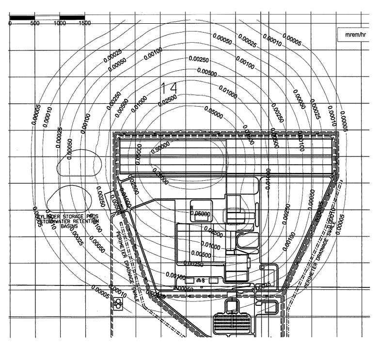
Figure 2: Dose Contours from Full Tails, Full Feed, and Empty Cylinder and Product Pads (mrem/hour) at the End of Plant Construction
