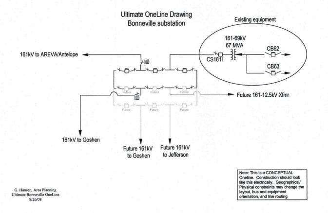
Figure 3: One-line diagram showing the ultimate layout of Bonneville substation.
