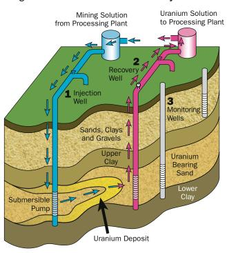
Figure 36. The In Situ Uranium Recovery Process
