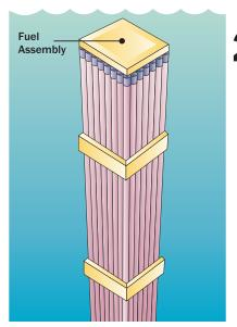
After about 6 years, spent fuel assemblies—typically 14 feet (4.3 meters) long and containing nearly 200 fuel rods for PWRs and 80–100 fuel rods for BWRs—are removed from the reactor and allowed to cool in storage pools for a few years. At this point, the 900-pound (40.8 kilograms) assemblies contain only about one-fifth the original amount of uranium-235.
