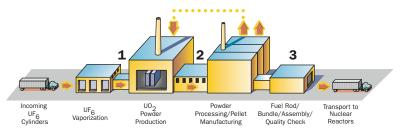
Fabrication is the final step in the process used to produce uranium fuel. Fuel fabrication facilities mechanically and chemically process the enriched uranium into nuclear reactor fuel.
