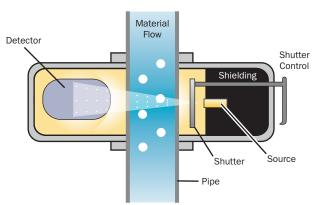
Figure 33. Cross-Section of Fixed Fluid Gauge
