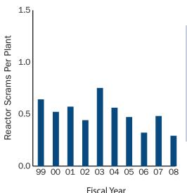
A reactor is said to be "critical" when it achieves a self-sustaining nuclear chain reaction, as when the reactor is operating. The sudden shutting down of a nuclear reactor by rapid insertion of control rods, either automatically or manually by the reactor operator, is referred to as a "scram." This indicator measures the number of unplanned automatic scrams that occurred while the reactor was critical.
