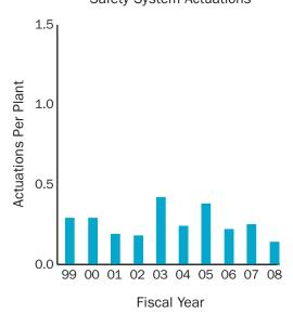
Safety system actuations are certain manual or automatic engagements of the logic or equipment of the emergency core cooling systems or emergency power systems. These systems are specifically designed to either remove heat from the reactor fuel rods if the normal core cooling system fails or provide emergency electrical power if the normal electrical systems fail.
