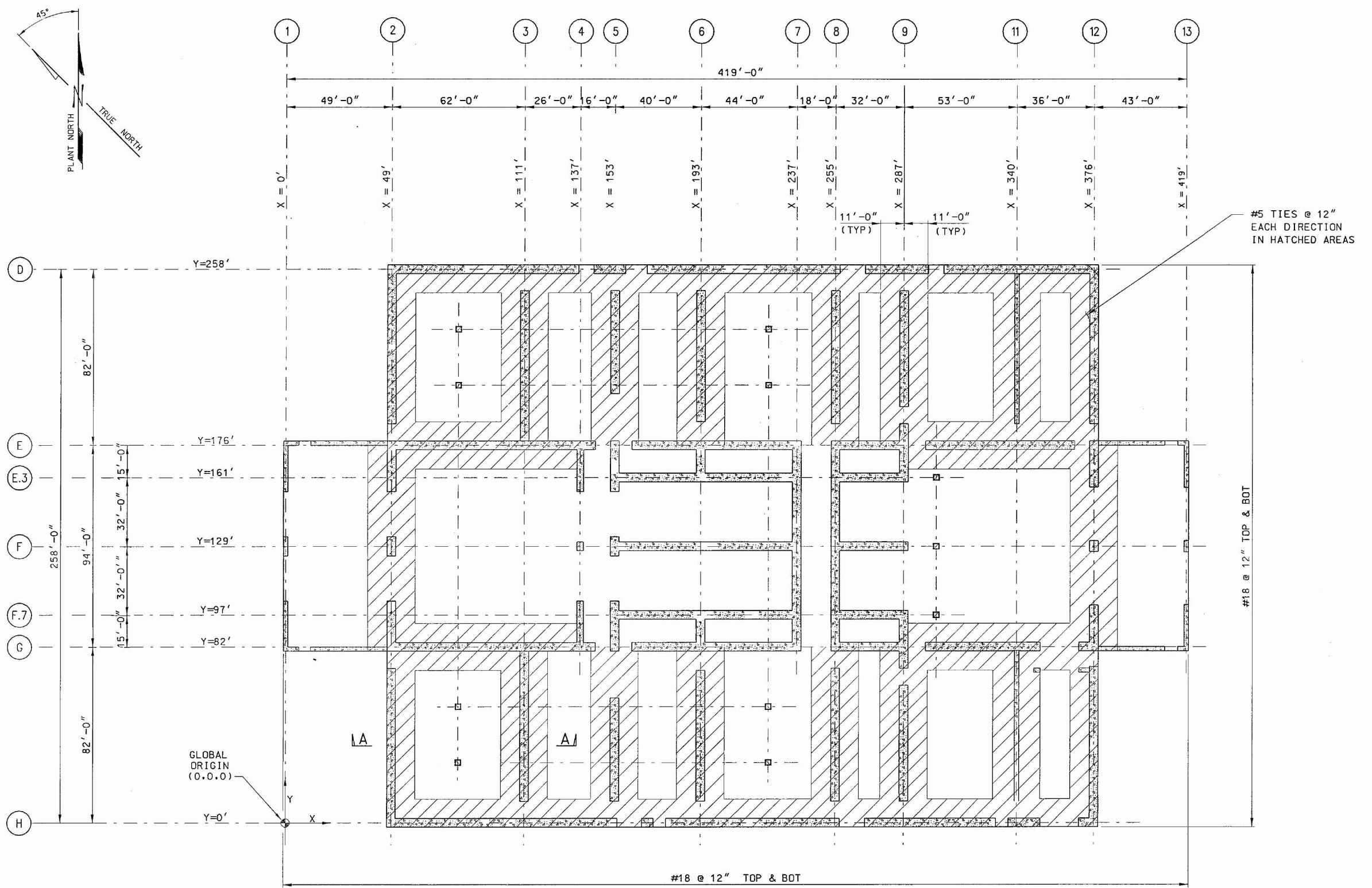
FIGURE 6.5.1 FOUNDATION MAT REINFORCEMENT (6'-0" THICK CONCRETE MAT)
