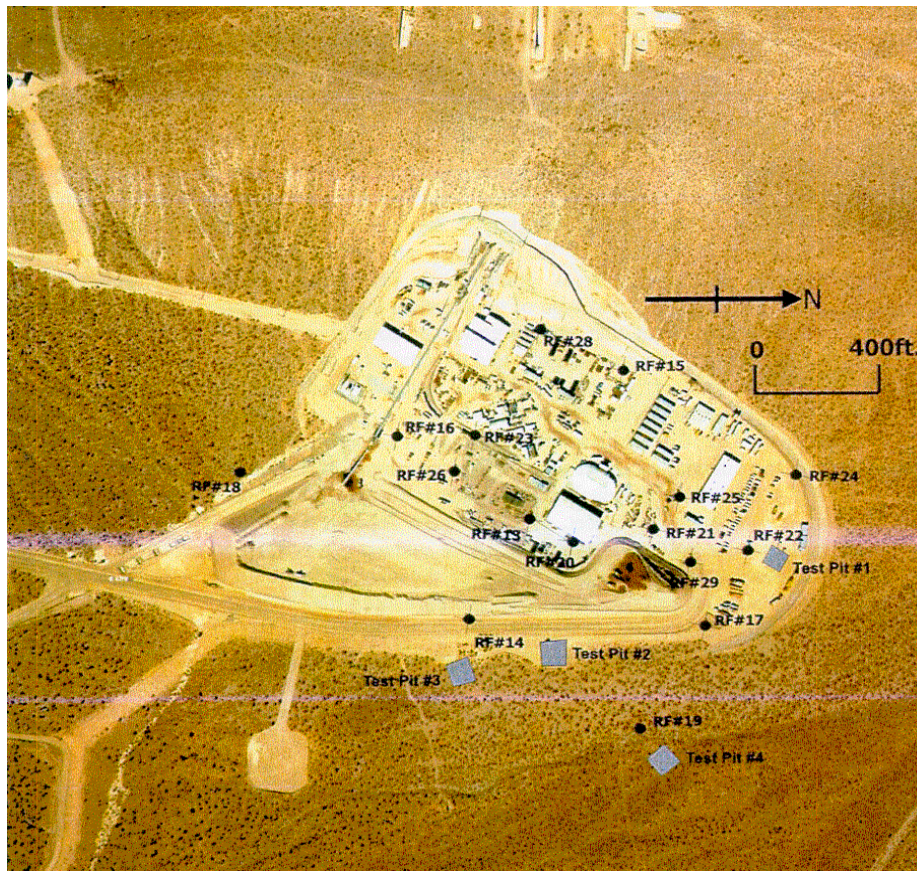
Figure A3-1. Locations of borings where downhole and suspension seismic surveys were conducted (Figure 2 of BSC 2002a, DTN:GS020383114233.001).
