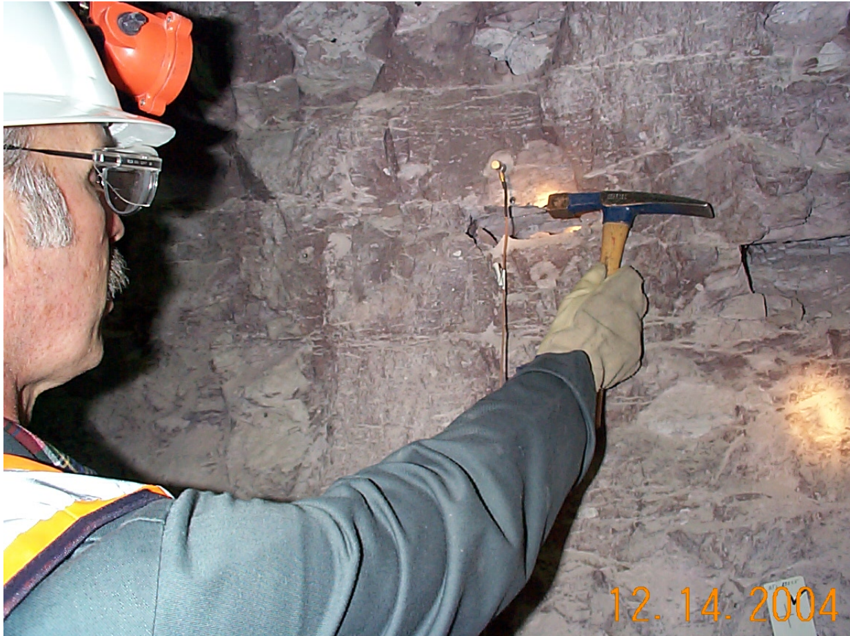
Figure 6.4-1. Typical Accelerometer Installation and Signal Source Hammer
