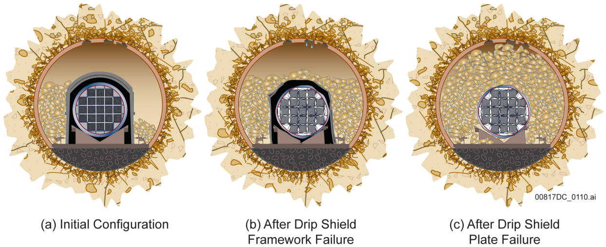
Figure 6.6-5. Schematic Representation of Future Configurations of EBS Components for Seismic Damage Abstraction
