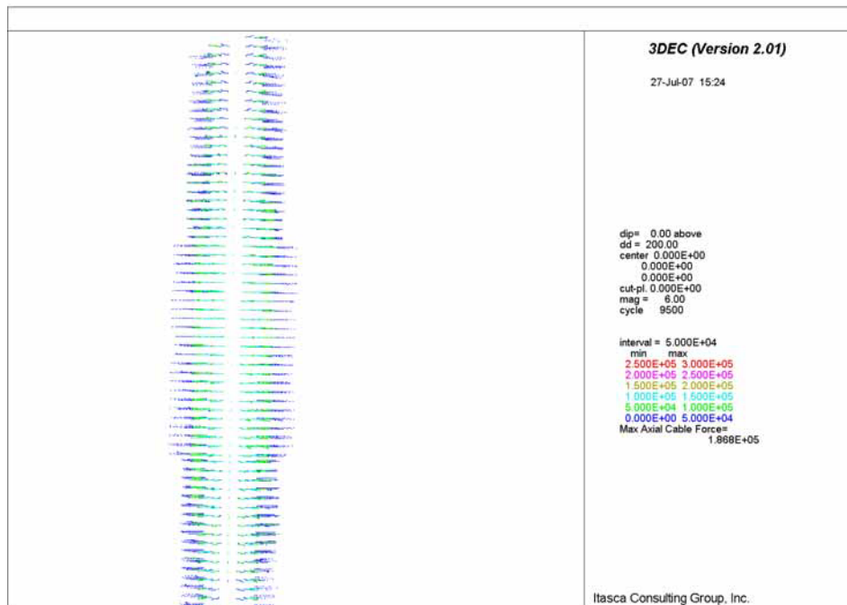
Figure 6-177 Axial Forces (N) in Bolts along Exhaust Main after Excavation
