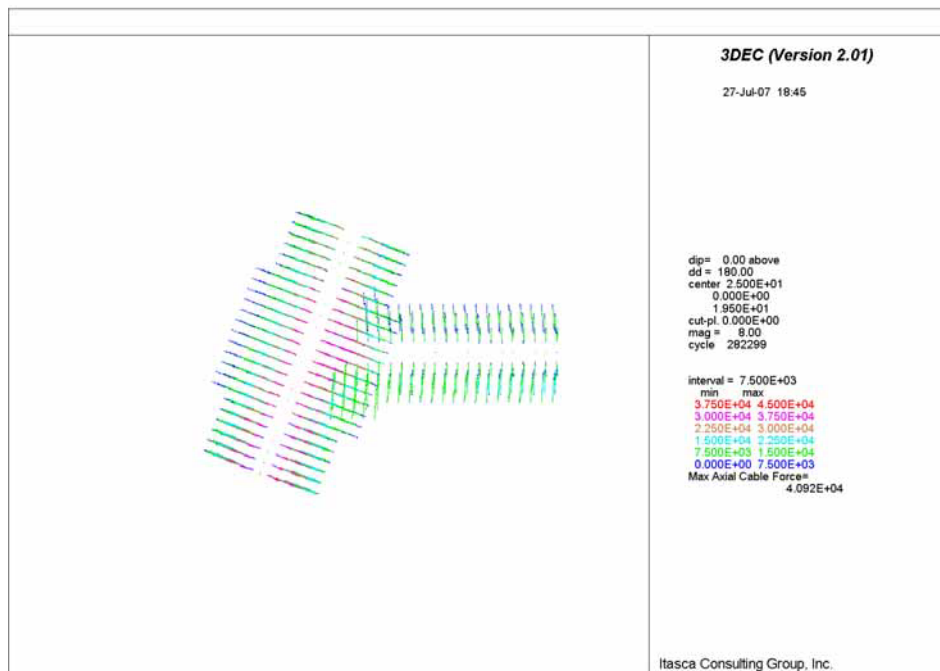
Figure 6-205 Plan View of Bolt Forces (N) in Intersection between Observation Drift and Exhaust Main after 15 Seconds of Seismic Shaking
