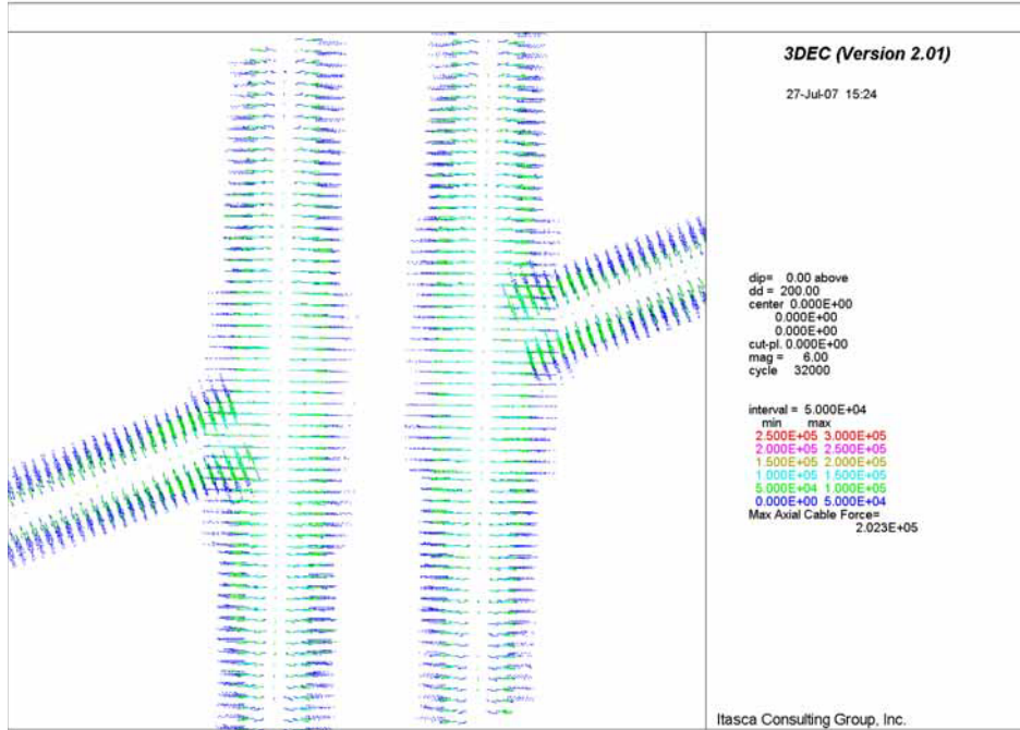
Figure 6-181 Plan View of Axial Forces (N) in Bolts along Exhaust Main after Excavation of Exhaust Main and Emplacement Drift
