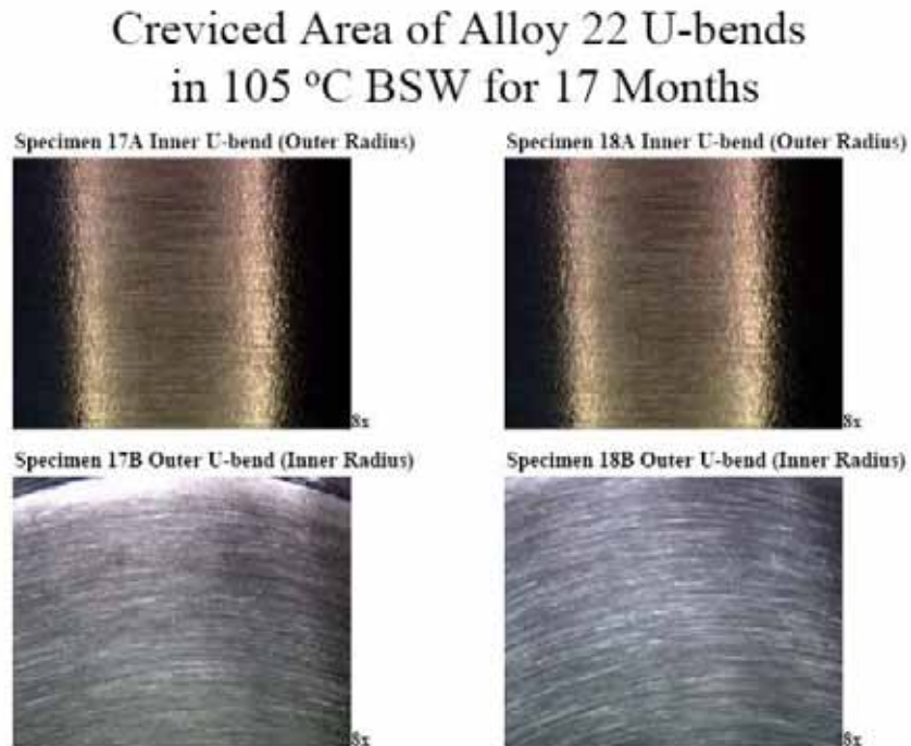
Figure 6-3. Alloy 22 Double U-Bend Specimens Exposed for 17 Months in 105°C BSW at LTCTF
