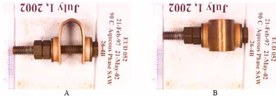
Figure 6-70. Welded Titanium Grade 12 U-bend Specimen after Five Years Exposure at LTCTF, (A) Side View Top and (B) Apex View
