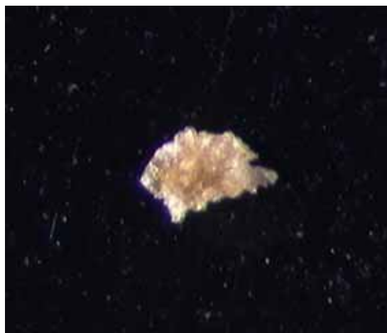
Figure 6-3[a]. Optical (50×) Photo of the Insoluble Particle That Formed from Four-Salt Mixture after 50 Days at 180°C
