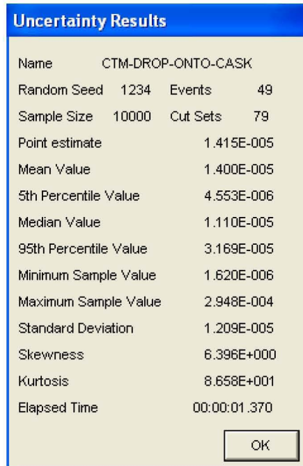
Figure B4.4-21. Uncertainty Results of the CTM Drop onto Canister Fault Tree
