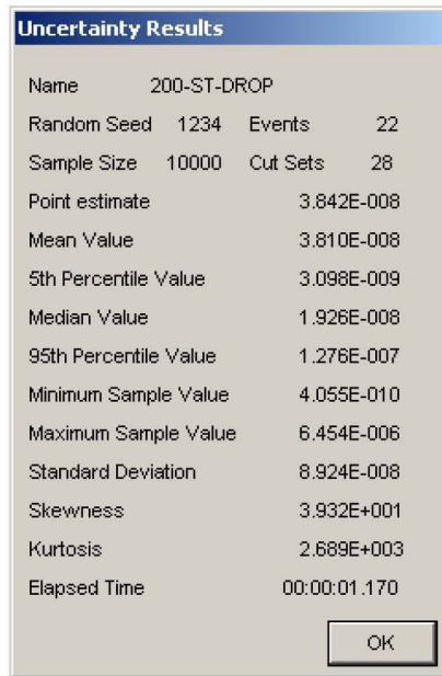
Figure B6.4-6. Uncertainty Results for the Site Transporter Load Drop during Lift and Movement Fault Tree
