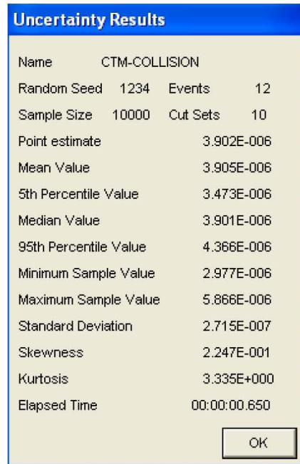
Figure B4.4-35. Uncertainty Results of the CTM Collision Fault Tree
