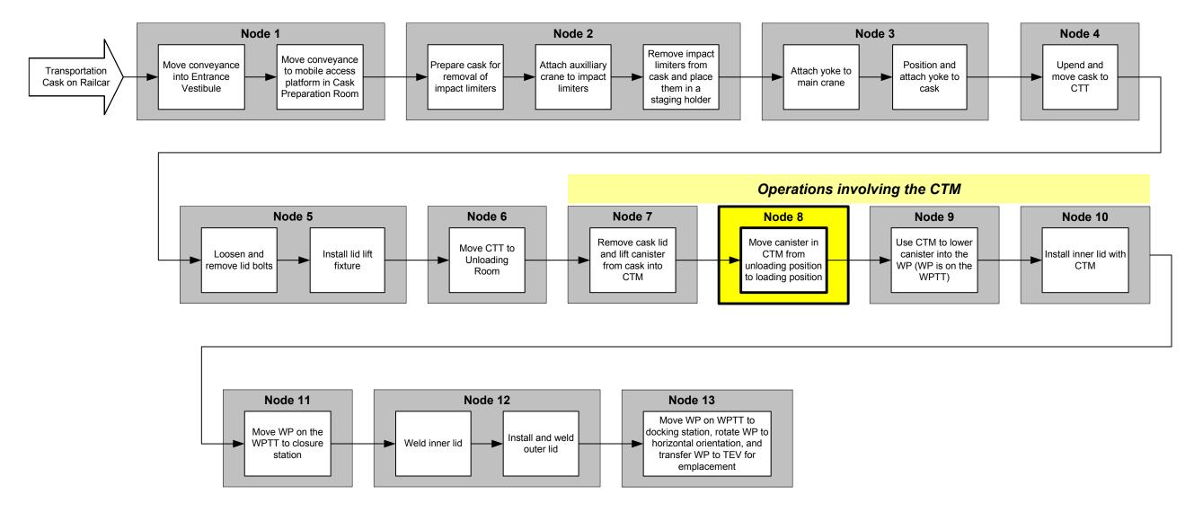
NOTE: CTT = cask transfer trolley; CTM = canister transfer machine; TEV = transport and emplacement vehicle; WP = waste package; WPTT = waste package transfer trolley.
