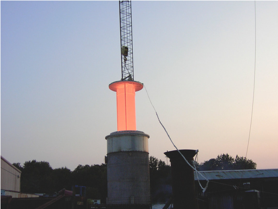
Figure C-1. Prototype Waste Package Outer Corrosion Barrier Entering Quench Tank
