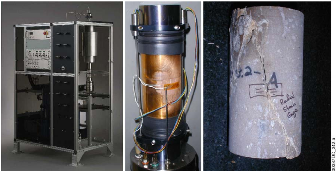
Figure 6-48. Triaxial Static Fatigue Experimental Setup and Posttest Sample for Heated, Saturated, 50.8 mm Diameter Samples of Tptpmn
