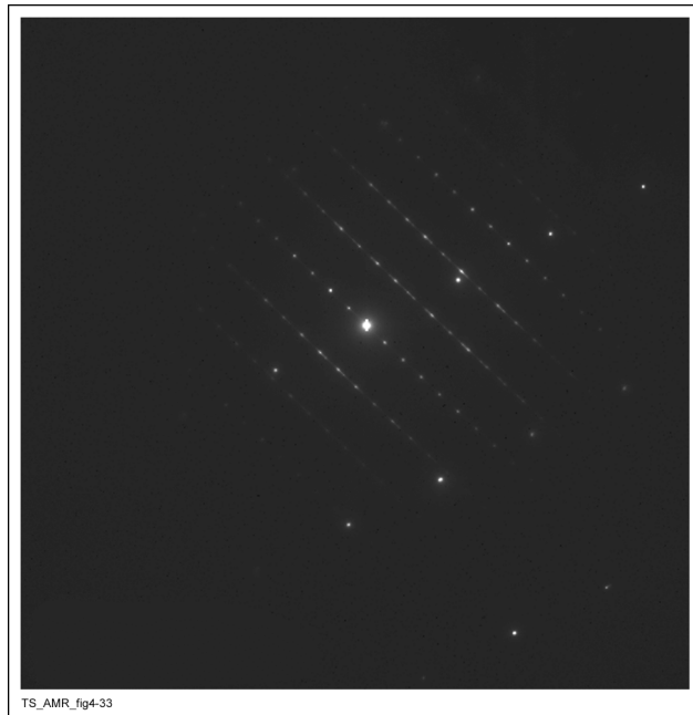
Figure 12. Precipitation (Possibly \mu Phase) in Alloy 22 Aged for 16,000 Hours at 760°C
