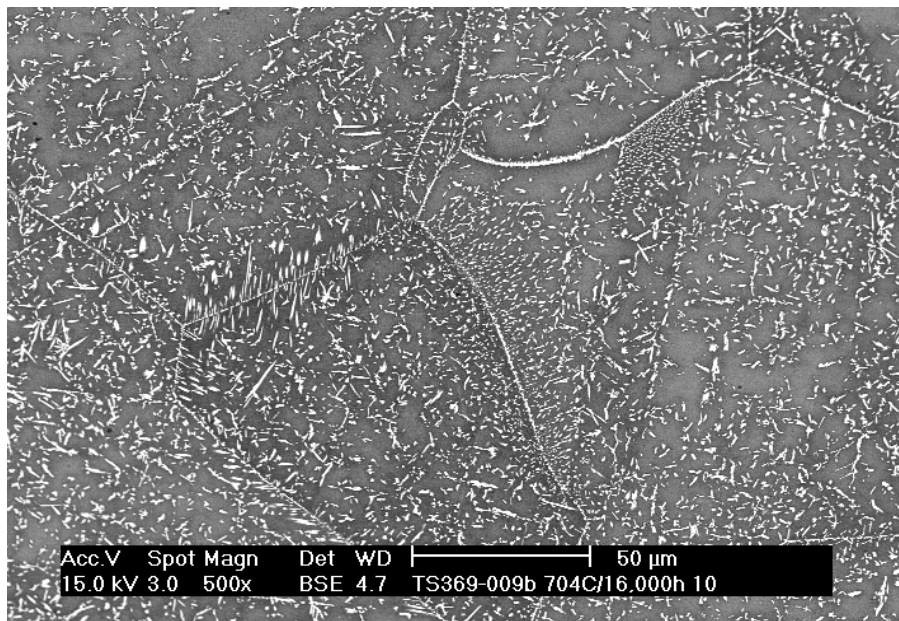
Figure 58. Base Metal aged at 649°C for 16,000 Hours
