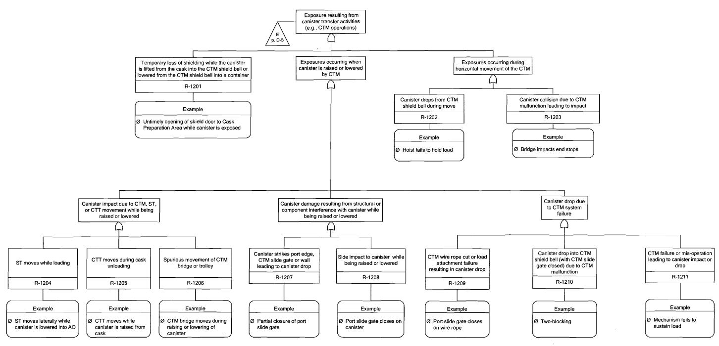
NOTES: Unplanned exposure of individuals to radiation or radioactive materials is referred to as "exposure."
