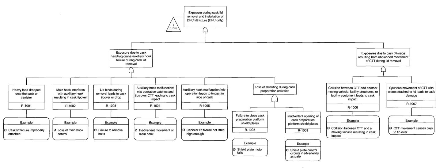
NOTES: Unplanned exposure of individuals to radiation or radioactive materials is referred to as "exposure." CTT = cask transfer trolley; DPC = dual-purpose canister.
