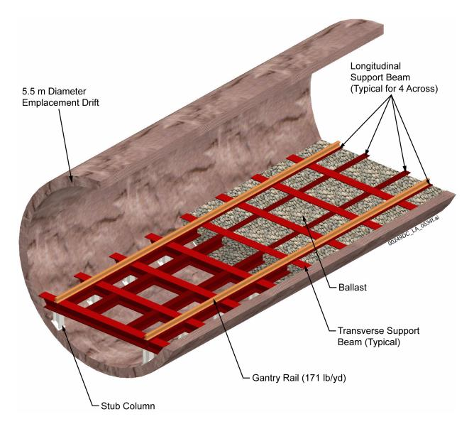
Figure 1.3.4-5. Emplacement Drift Steel Invert
