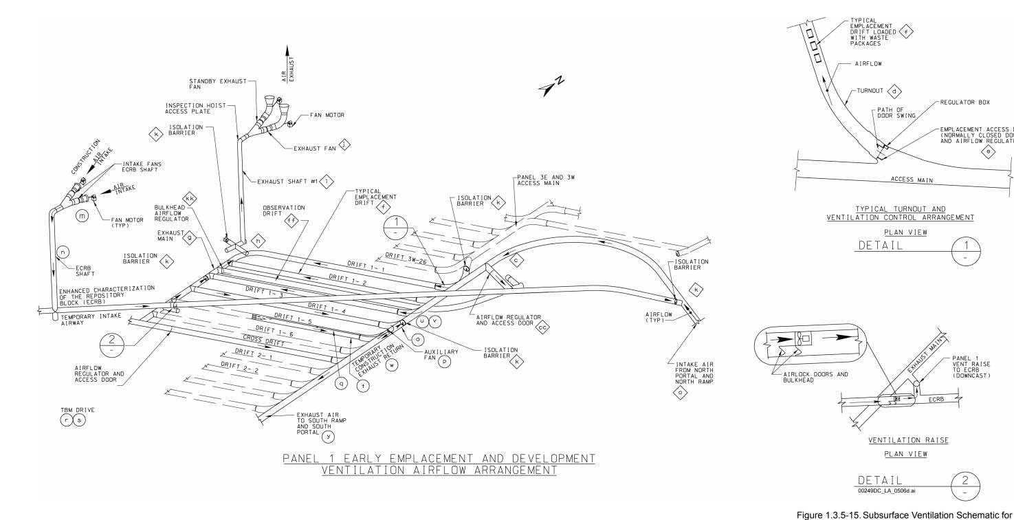
Panel 1 Development and Emplacement NOTE: TBM = Tunnel boring machine. Sides
