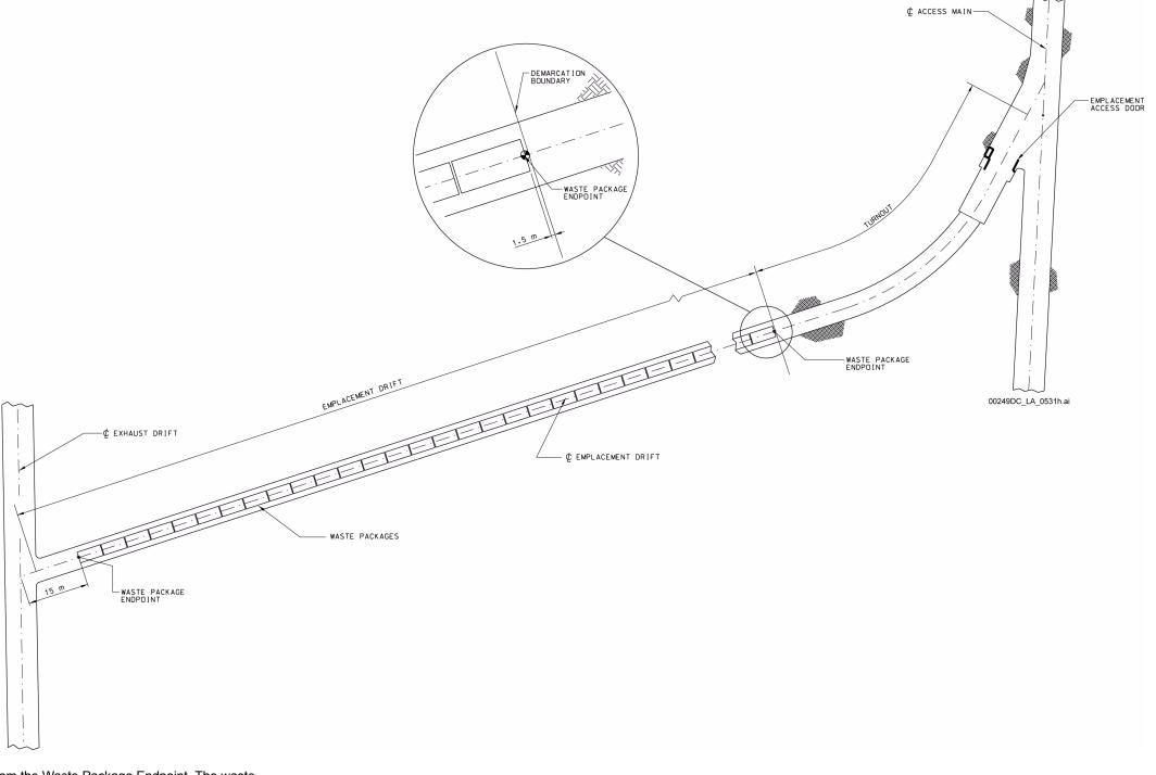
NOTE: Emplacement drift—turnout demarcation boundary is 5.0 ft (1.5 m) from the Waste Package Endpoint. The waste package standoff distance to the centerline of the exhaust main is 49 ft (15 m).
