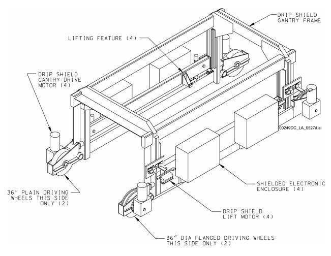
Figure 1.3.4-17. Drip Shield Emplacement Gantry
