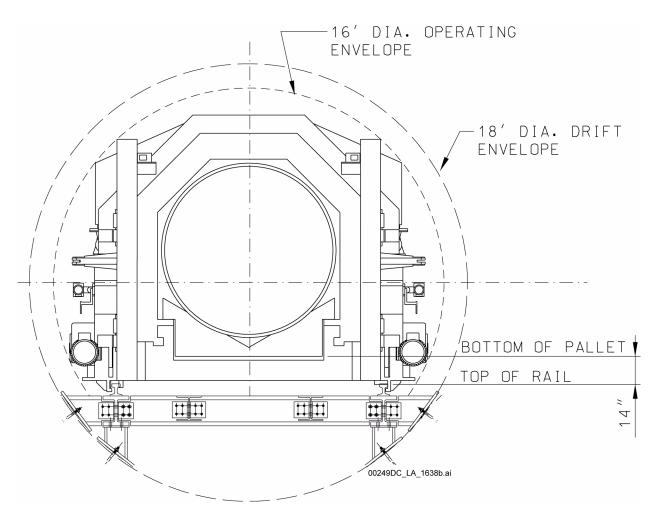
Figure 1.3.4-20. Transport and Emplacement Vehicle with Waste Package in the Emplacement Drift
