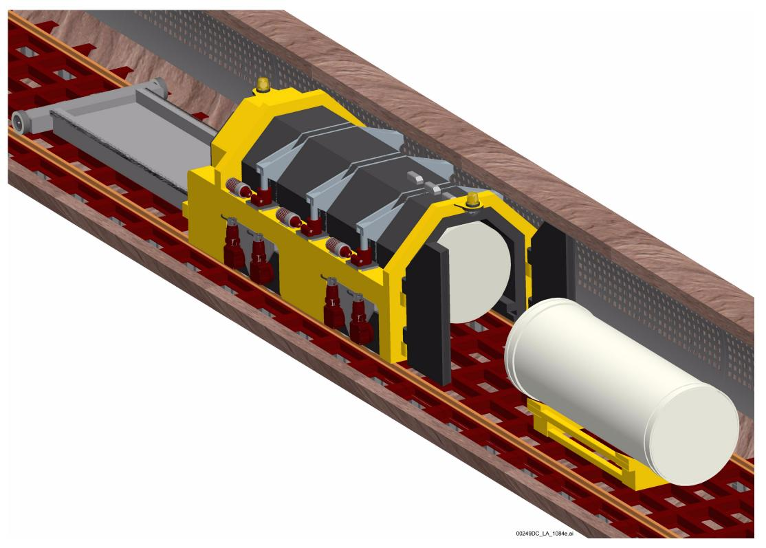
NOTE: A more specific presentation of the Transport and Emplacement Vehicle configuration is provided in Figures 1.3.3-39 and 1.3.3-40. Third rail is not shown.
