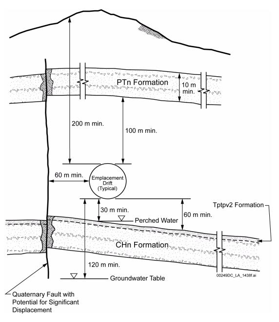
Figure 1.3.4-1. Simplified Representation of the Subsurface Facility Standoffs as Applicable to an Emplacement Drift
