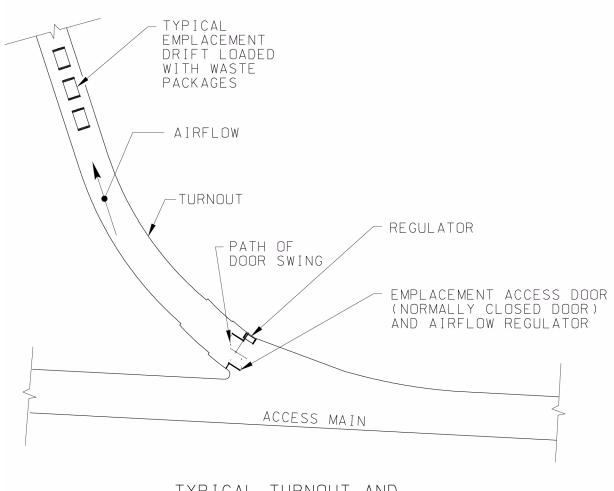
TYPICAL TURNOUT AND VENTILATION CONTROL ARRANGEMENT
