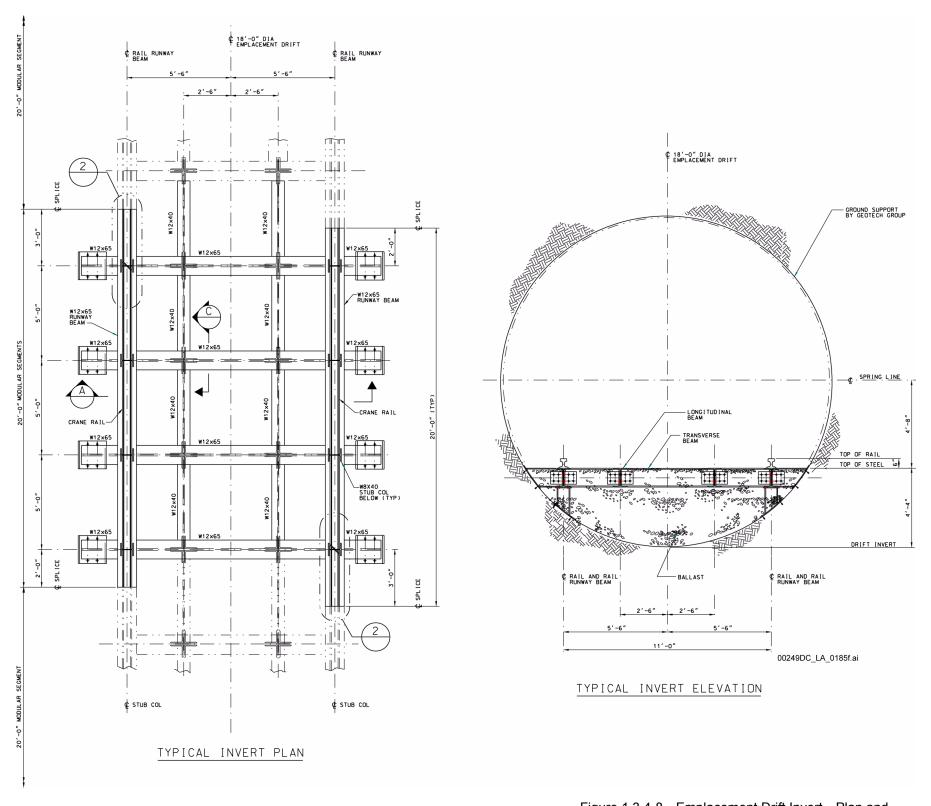
Figure 1.3.4-8. Emplacement Drift Invert—Plan and Elevation
