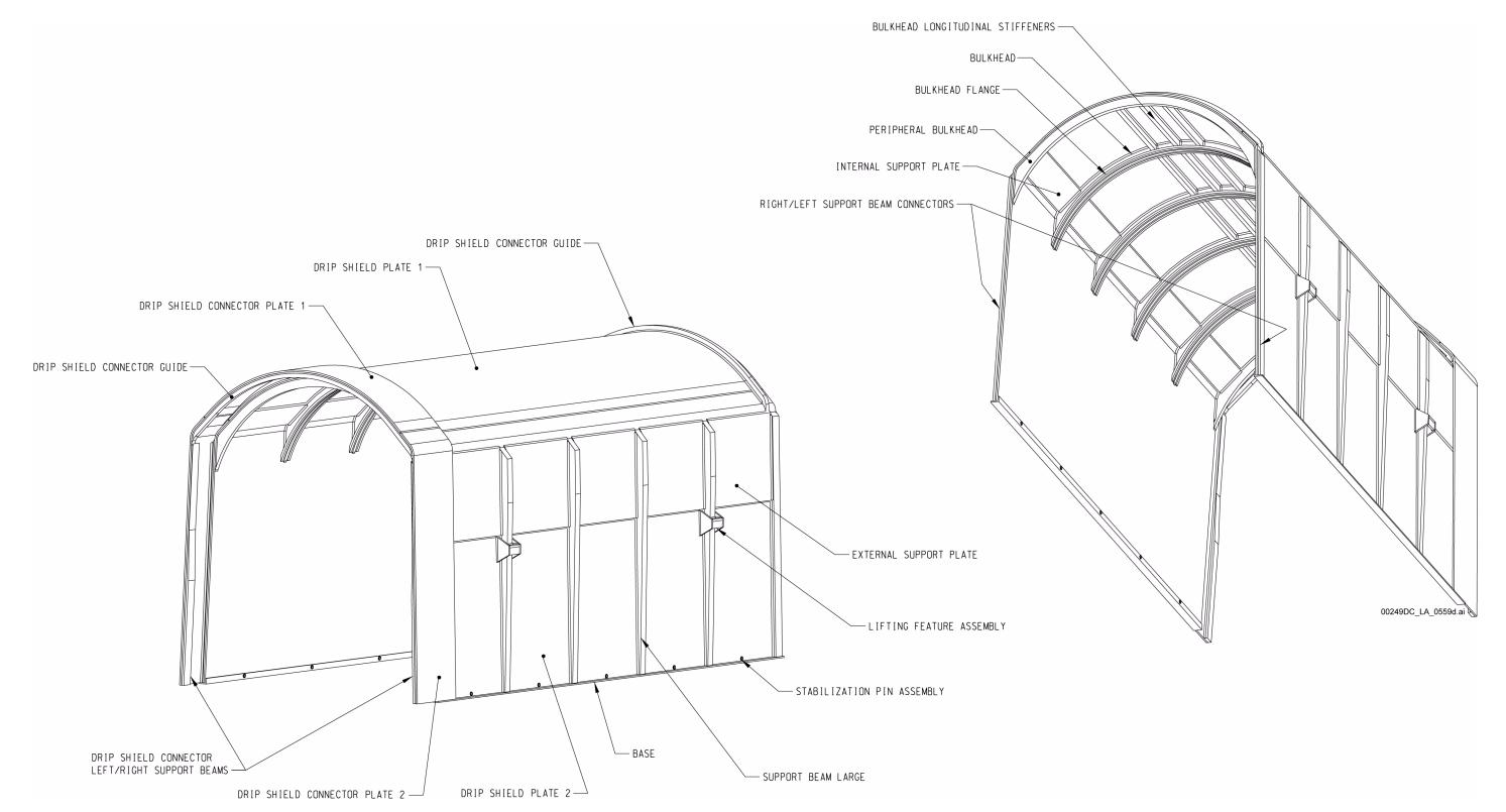
Figure 1.3.4-14. Interlocking Drip Shield
