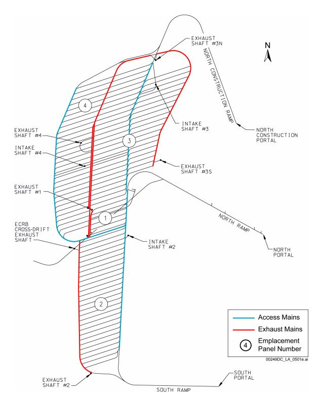
Figure 1.3.5-2. Underground Layout and Location of Ramps and Shafts
