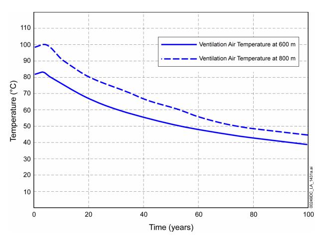
Figure 1.3.4-16. Emplacement Drift Exhaust Air Temperatures as a Function of Time and Distance from the Drift Inlet (Full Drift) for Drifts Loaded with a Thermal Line Load of 2.0 kW/m
