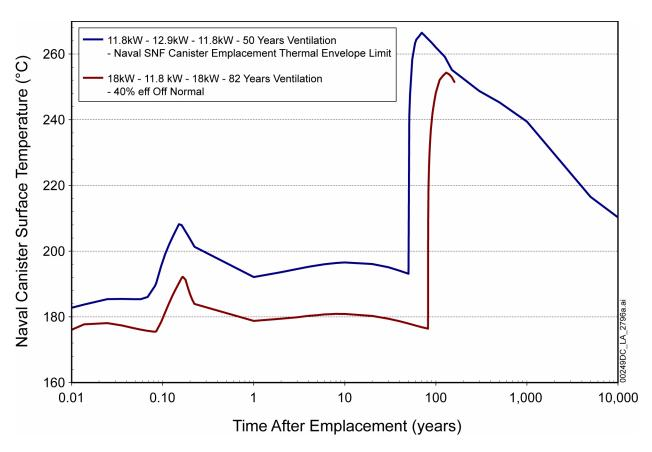
Figure 1.3.5-20. Naval SNF Canister Surface Temperature Comparison—Misplacement of an 11.8-kW Naval SNF Waste Package in a 2.0-kW/m Commercial SNF Drift Segment with 40% Natural Ventilation Efficiency During Preclosure and with Occurrence of an Off-Normal Condition
