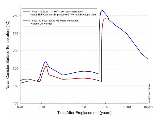
Figure 1.3.5-19. Naval SNF Canister Surface Temperature Comparison—Misplacement of a 22.0-kW Commercial SNF Waste Package in a 1.45-kW/m Naval Drift Segment Loaded with One 12.9-kW Naval SNF Waste Package, with 40% Natural Ventilation Efficiency During Preclosure and with Occurrence of an Off-Normal Condition
