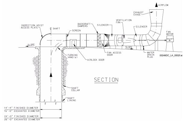
Figure 1.3.5-3. Typical Exhaust Fan Installation Configuration, Section and Plan View
