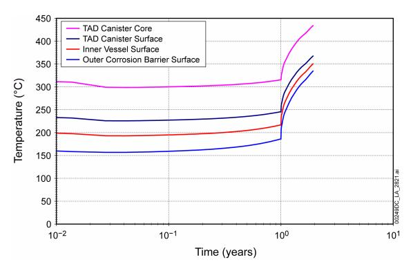
Figure 1.3.5-18. Temperature Histories for an 18.0-kW TAD Waste Package, Case 4v\_1y Boundary Conditions
