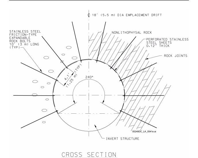
Figure 1.3.4-7. Schematic of Typical Emplacement Drift Permanent Ground Support
