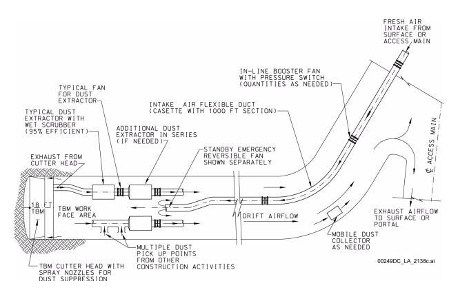
Figure 1.3.5-16. Typical Local Ventilation Arrangement for the Tunnel Boring Machine Excavation
