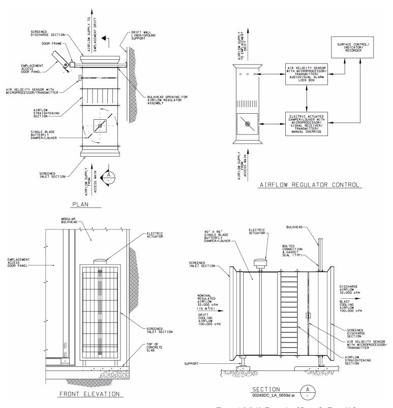
Figure 1.3.5-13. Example of Butterfly-Type Airflow Regulator
