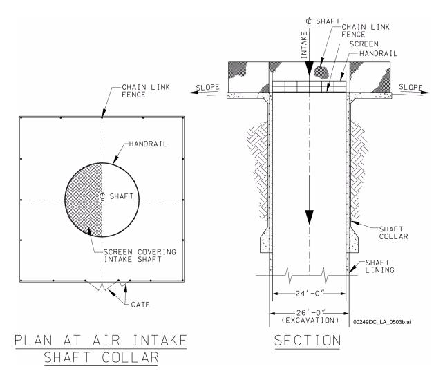
Figure 1.3.5-4. Typical Intake Shaft Configuration, Section and Plan View
