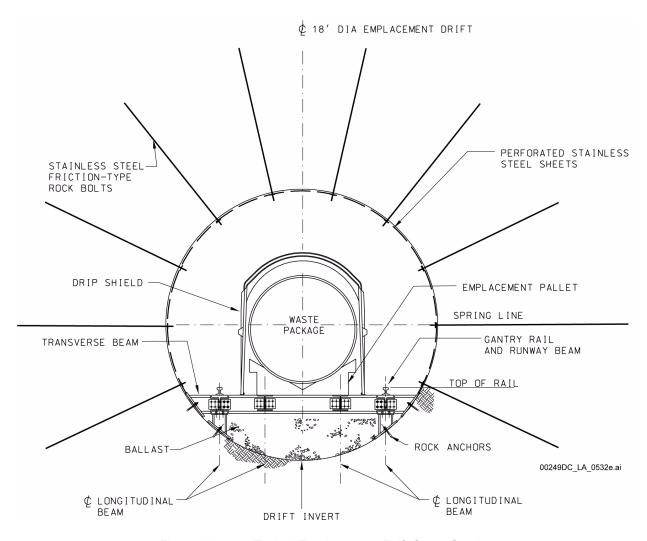
Figure 1.3.4-4. Typical Emplacement Drift Cross Section
