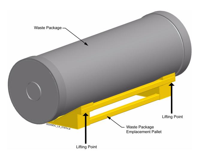
Figure 1.3.4-13. Emplacement Pallet Loaded with Waste Package
