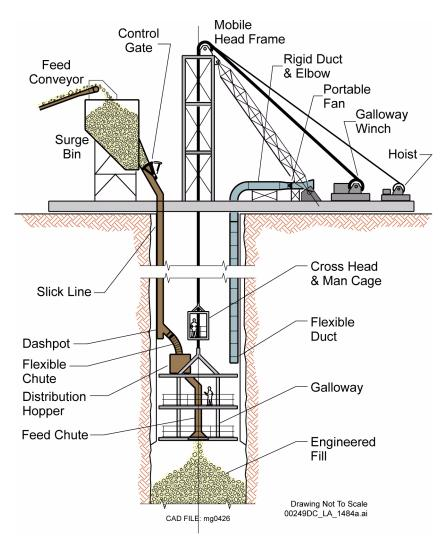
Figure 1.3.6-3. Conceptual Arrangement for Placement of Backfill in Shafts
