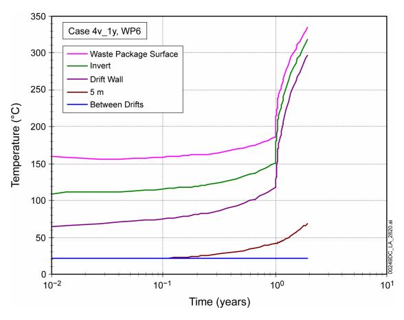
Figure 1.3.5-17. Peak Temperature Histories for Emplacement Drift Wall and EBS Components
