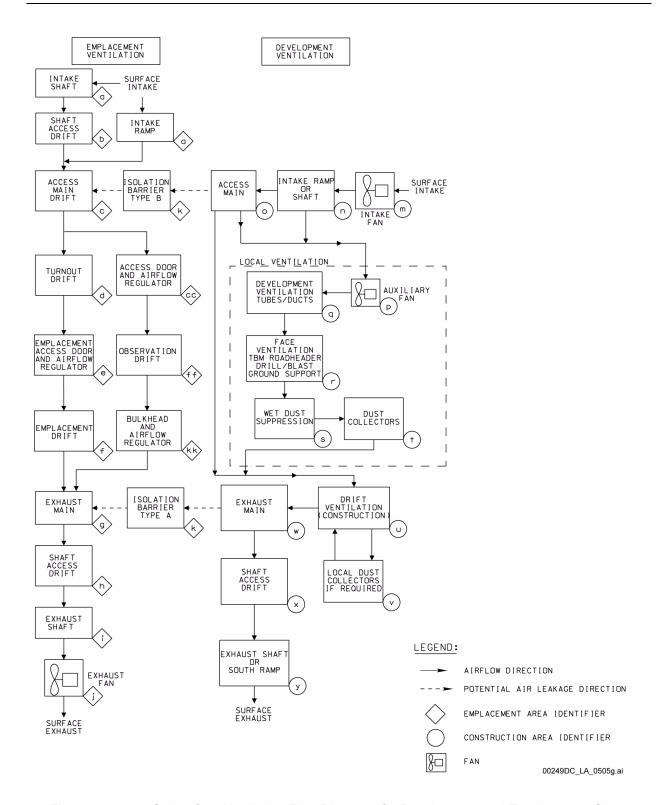
Figure 1.3.5-14. Subsurface Ventilation Flow Diagrams for Development and Emplacement Sides
