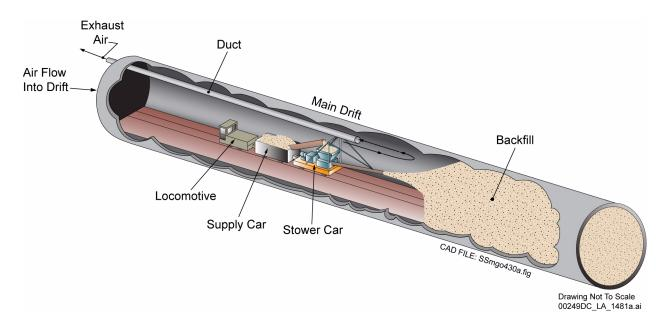
Figure 1.3.6-2. Conceptual Arrangement for Placement of Backfill in Ramps
