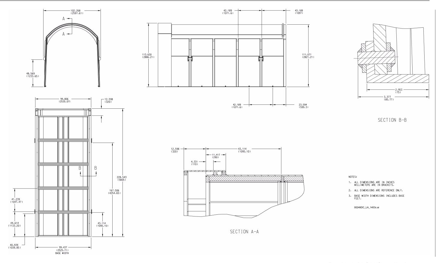
Figure 1.3.4-15. Drip Shield Structural Details
