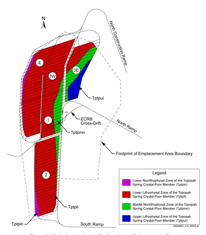
Figure 1.3.4-2. Underground Layout Configuration and Geologic Units by Panel
