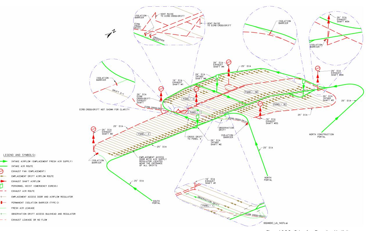
Figure 1.3.5-5. Subsurface Repository Ventilation System at Full Emplacement
