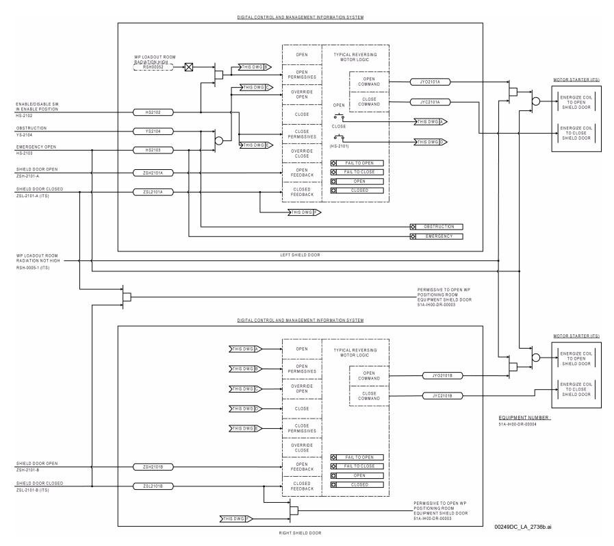
NOTE: Important to safety controls are identified by the letters "ITS" after the instrumentation tag number or control device identifier. The DCMIS is non-ITS and non-ITWI. Instrumentation tag numbers are prefixed by "51A-HL00-" and software tag numbers are prefixed by "51AHL00." WP = waste package.
