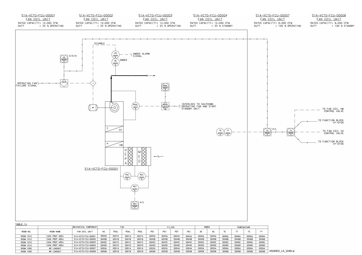
NOTE: This figure includes no SSCs that are either ITS or ITWI. An interlock is provided to shut down the operating fan and start the standby unit upon detection of low differential pressure across the operation fan coil unit. CH = chilled water; HW = hot water; WP = waste package.
