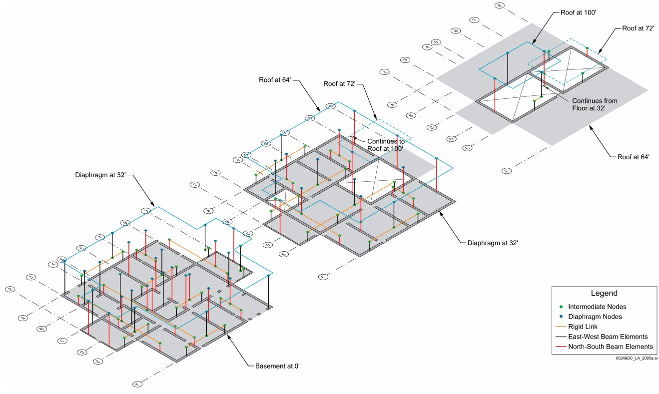
Figure 1.2.2-16. Receipt Facility Lumped-Mass, Multiple-Stick Model
