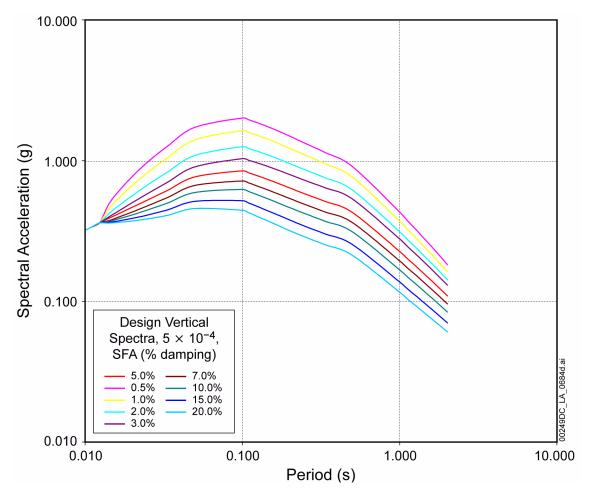
Figure 1.2.2-11. Vertical Ground Response Spectra at Multiple Dampings for a Mean Annual Exceedance Probability of  $5 \times 10^{-4}$
