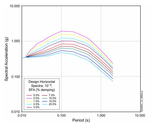
Figure 1.2.2-8. Horizontal Ground Response Spectra at Multiple Dampings for a Mean Annual Exceedance Probability of 10<sup>-3</sup>
