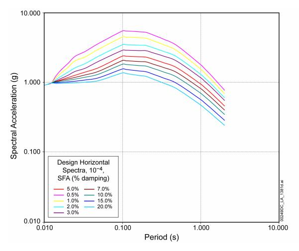
Figure 1.2.2-12. Horizontal Ground Response Spectra at Multiple Dampings for a Mean Annual Exceedance Probability of 10<sup>-4</sup>
