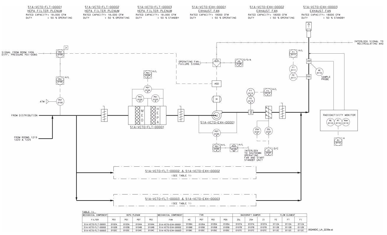
NOTE: This figure includes no SSCs that are either ITS or ITWI. An operating fan failure signal starts this unit (if it is in auto). An interlock is provided to shut down the operating fan and start the standby unit upon detection of high or low differential pressure across the operating fan. AHU = air handling unit.
