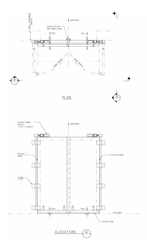
Equipment Number: 51A-IH00-DR-00003, waste package positioning room equipment shield door.
