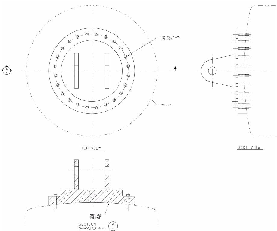
Equipment Number: 51A-HMC0-HEQ-00005, naval cask lift plate.
