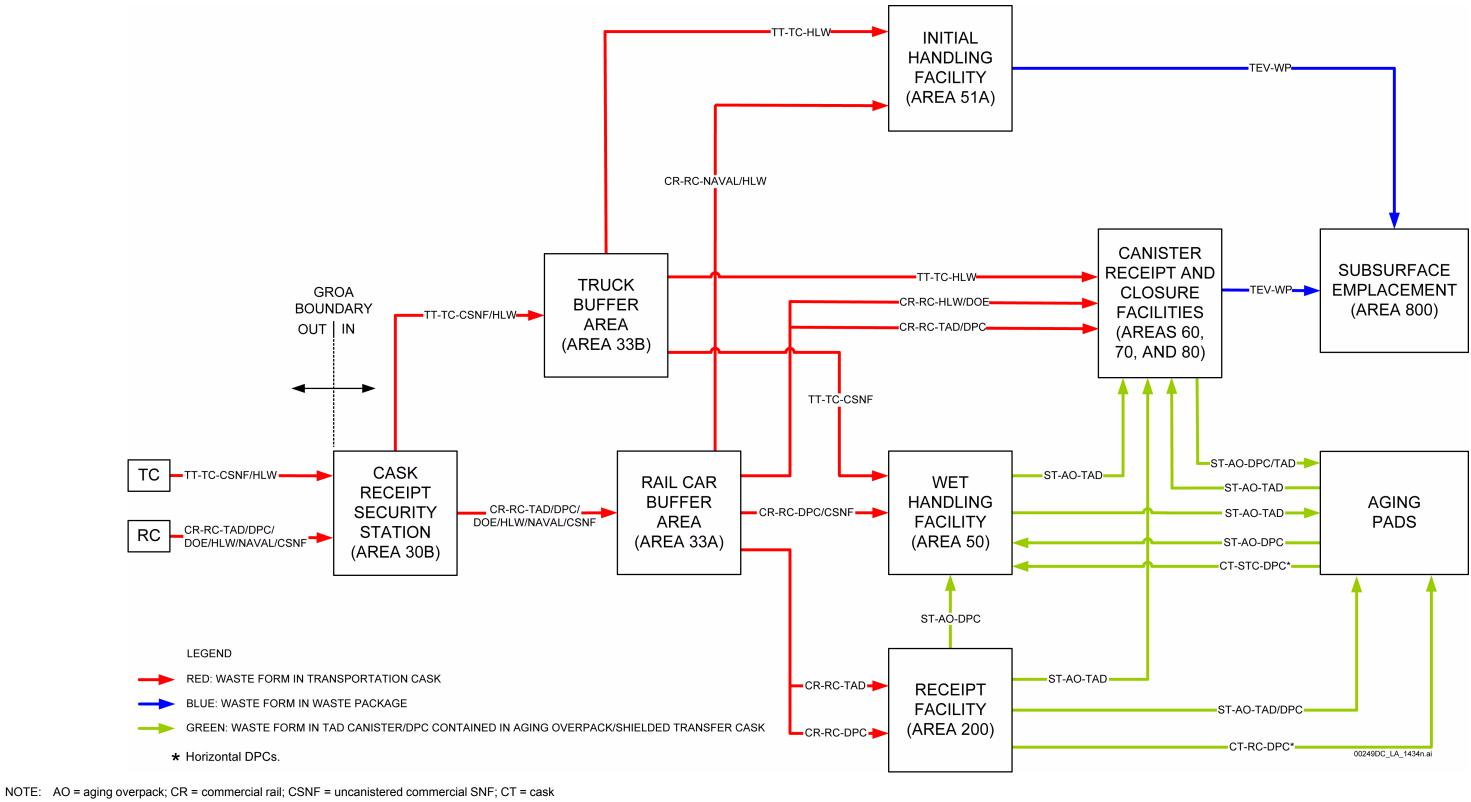
tractor and cask transfer trailer; DOE = DOE SNF canister; HLW = HLW canister; Naval = naval SNF canister; RC = rail cask/overpack; ST = site transporter; STC = shielded transfer cask; TC = truck cask/overpack; TT = truck trailer; WP = waste package.
