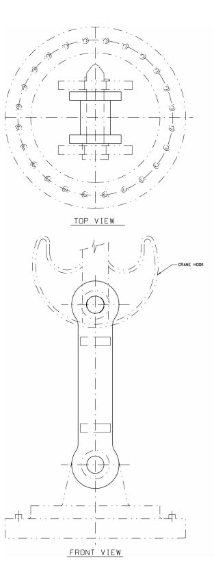
Equipment Number: 51A-HMC0-BEAM-00001, naval cask lift bail.
