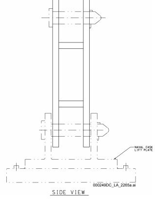
Figure 1.2.3-24. Naval Cask Lift Bail Mechanical Equipment Envelope
