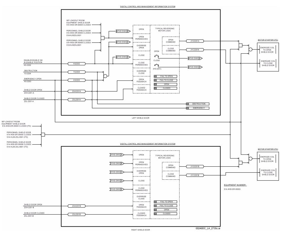
NOTE: Important to safety controls are identified by the letters "ITS" after the instrumentation tag number or control device identifier. The DCMIS is non-ITS and non-ITWI. Instrumentation tag numbers are prefixed by "51A-HW00-" and software tag numbers are prefixed by "51AHW00."
