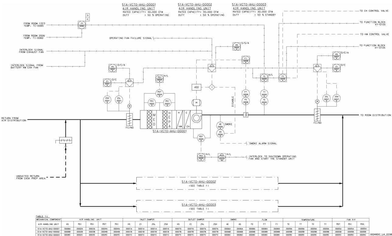
NOTE: This figure includes no SSCs that are either ITS or ITWI. If a smoke alarm signal is detected, the signal is directed to fire alarm panel. An interlock is provided to shut down the operating fan and start the standby unit upon detection of high or low differential pressure across the operating fan. An operating fan failure signal starts this unit (if it is in auto). CH = chilled water; HW = hot water.
