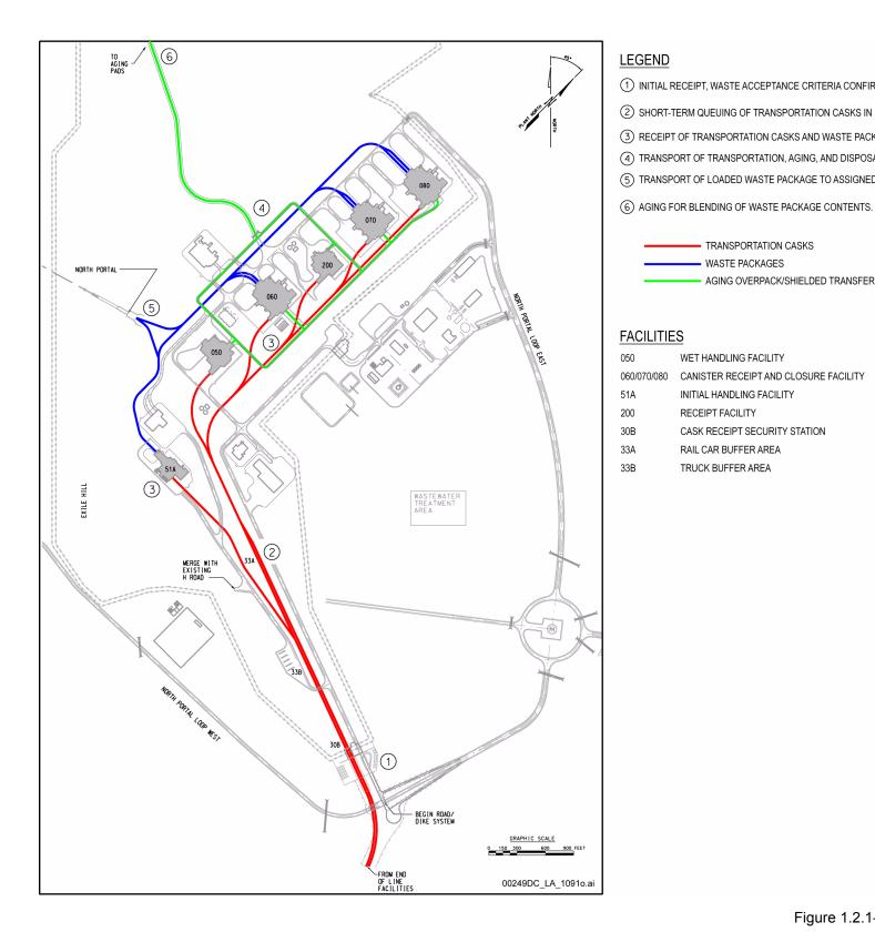
(1) INITIAL RECEIPT, WASTE ACCEPTANCE CRITERIA CONFIRMATION, SECURITY ENTRY INSPECTION, AND RADIOLOGICAL SURVEY.
