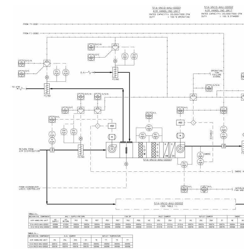
NOTE: This figure includes no SSCs that are either ITS or ITWI. If a smoke alarm signal detected, it is directed to the fire alarm panel. An interlock is provided to shut down the operating fan and start the standby unit upon detection of high or low differential pressure across the operating fan. CH = chilled water; HW = hot water; OA = outside air.
