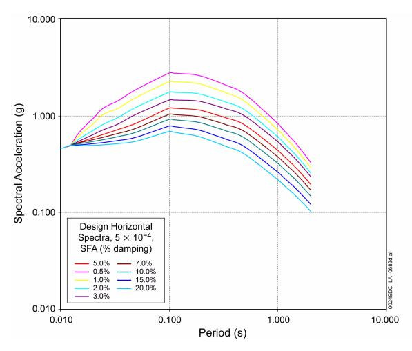
Figure 1.2.2-10. Horizontal Ground Response Spectra at Multiple Dampings for a Mean Annual Exceedance Probability of  $5 \times 10^{-4}$
