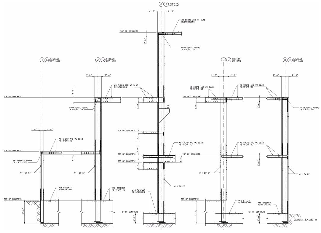
Figure 1.2.2-1. Typical Canister Receipt and Closure Facility Reinforcing Sections
