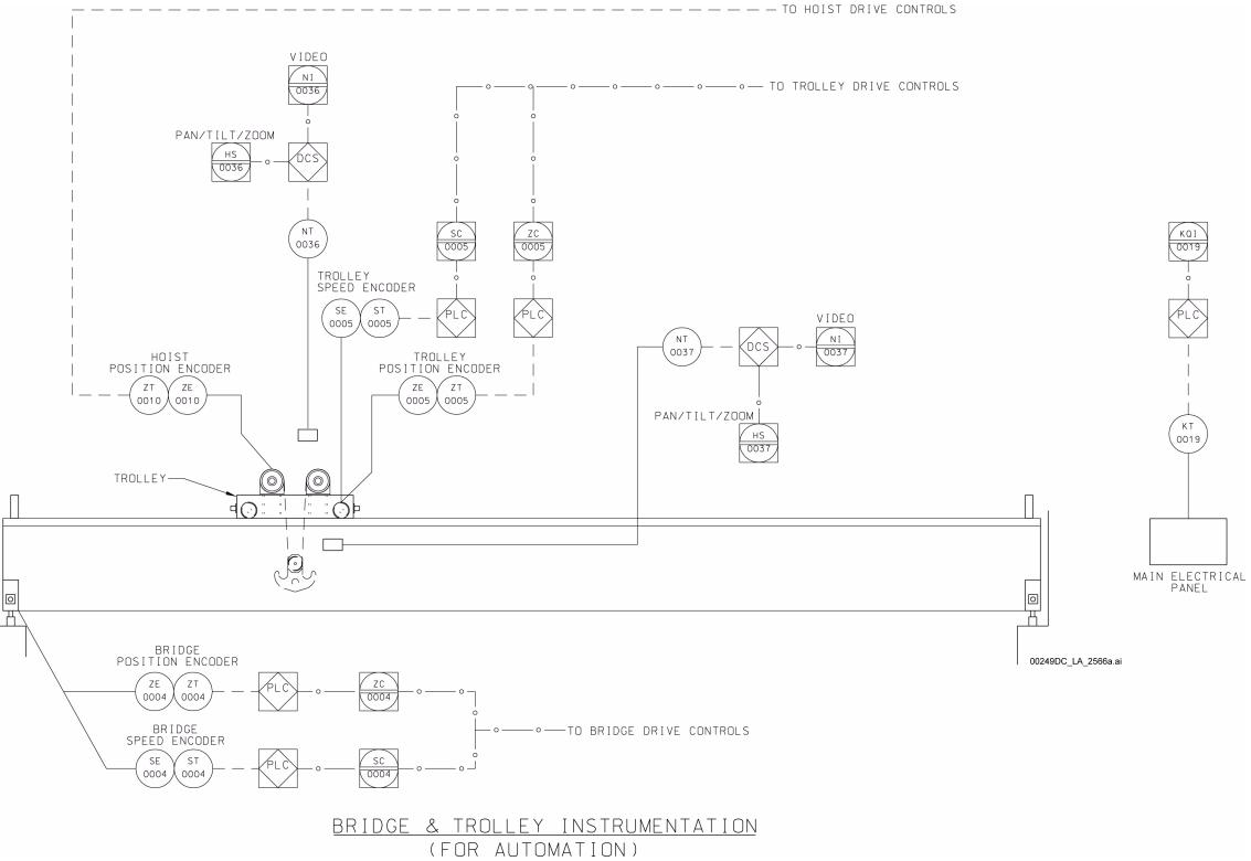
Figure 1.2.3-22. Cask Preparation Crane Process and Instrumentation Diagram (Sheet 3 of 3)
