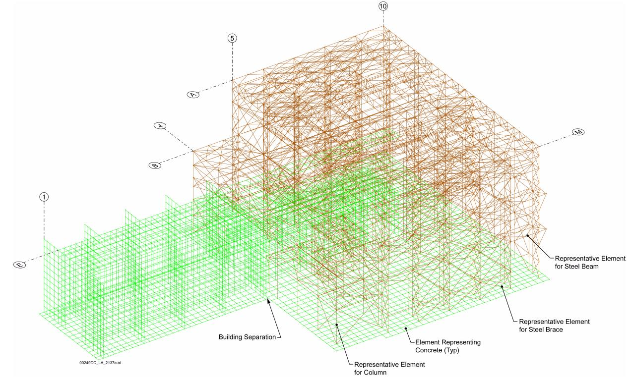
Figure 1.2.2-18. Initial Handling Facility Model
