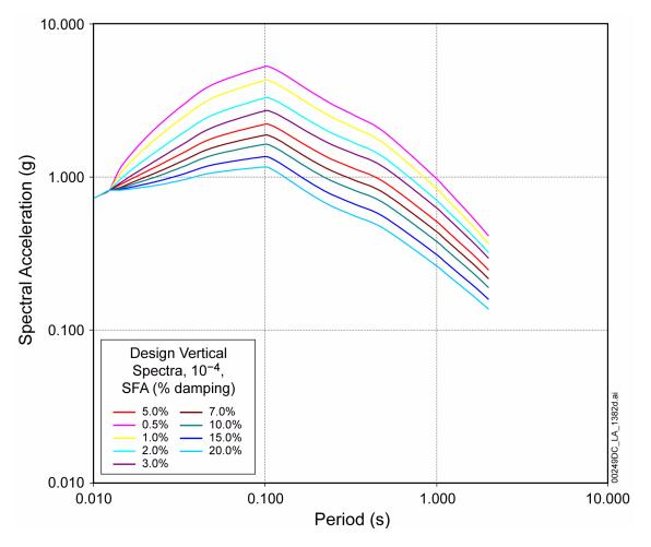
Figure 1.2.2-13. Vertical Ground Response Spectra at Multiple Dampings for a Mean Annual Exceedance Probability of  $10^{-4}$
