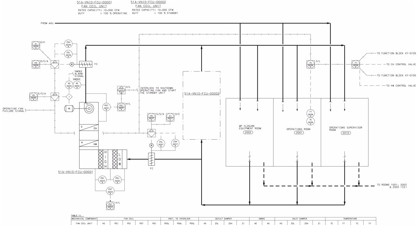
NOTE: This figure includes no SSCs that are either ITS or ITWI. An interlock is provided to shut down operating fan and start the standby unit upon detection of high or low differential pressure across the operation fan coil unit. CH = chilled water; HW = hot water; WP = waste package.
