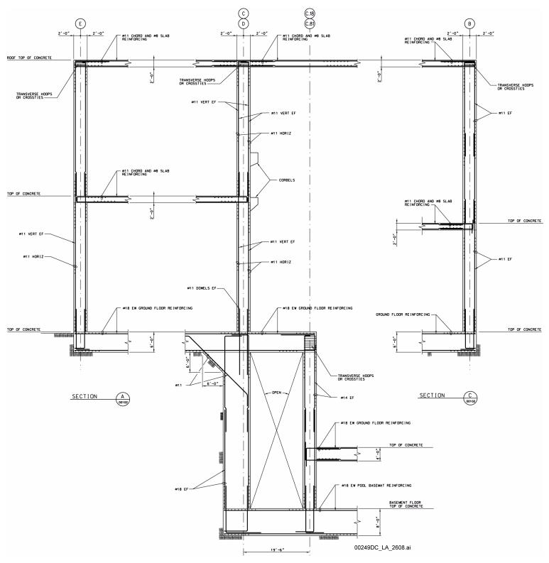
Figure 1.2.2-2. Typical Wet Handling Facility Reinforcing Sections
