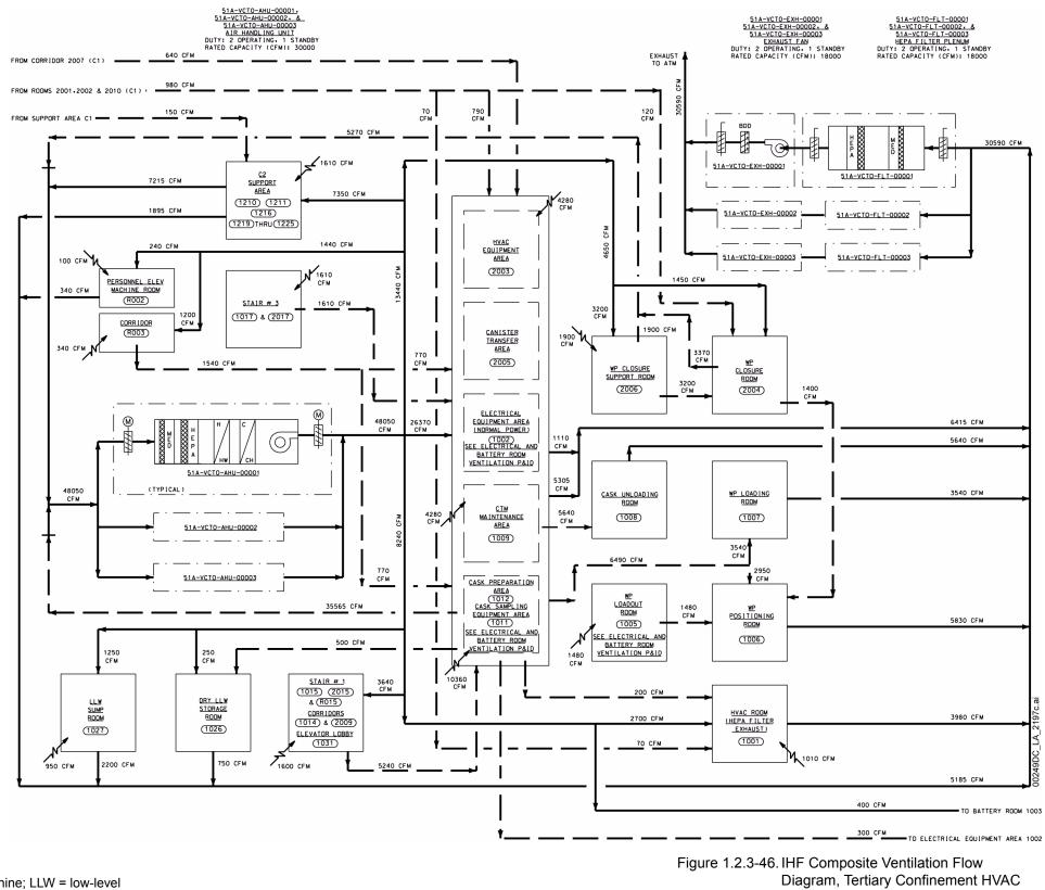
NOTE: This figure includes no SSCs that are either ITS or ITWI. CTM = canister transfer machine; LLW = low-level radioactive waste; WP = waste package.
