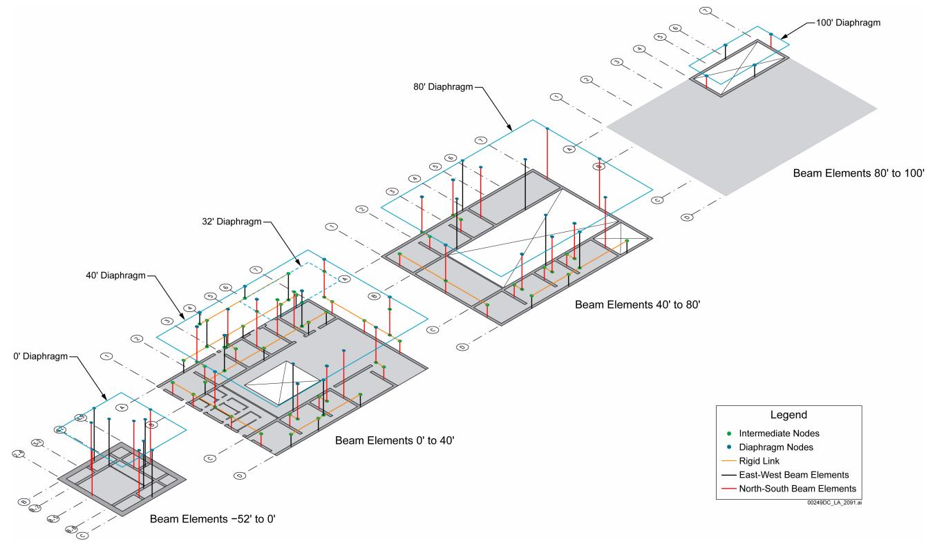
Figure 1.2.2-15. Wet Handling Facility Lumped-Mass, Multiple-Stick Model
