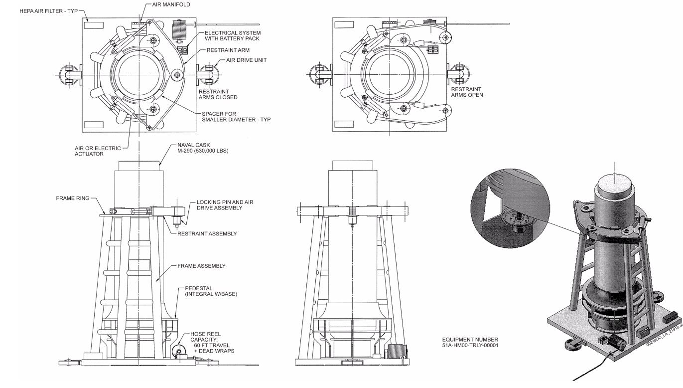
Figure 1.2.3-20. Cask Transfer Trolley Mechanical Equipment Envelope
