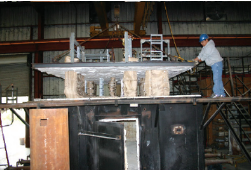
Assembly of insulated electrical cables being lowered into a furnace that reaches 1700° F for a 1-hour test
