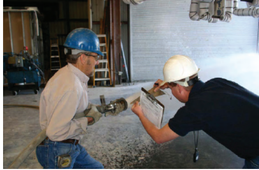
Simulation of water flow from a fire hose that may be used to extinguish a cable insulation fire
