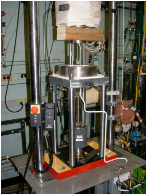
Figure 9. Photograph of the specimen load train for the 2-liter autoclave.
