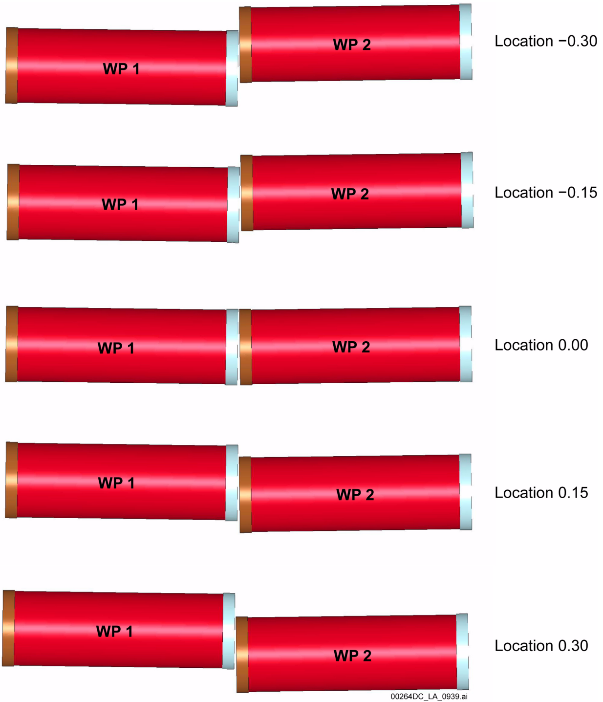
Figure 2.3.4-65. Example of Impact Location Configurations for TAD-Bearing Waste Package-to-TAD-Bearing Waste Package Damage Lookup Table Analyses. All Analyses Were Performed with an Impact Angle of 1.5 Degrees.
