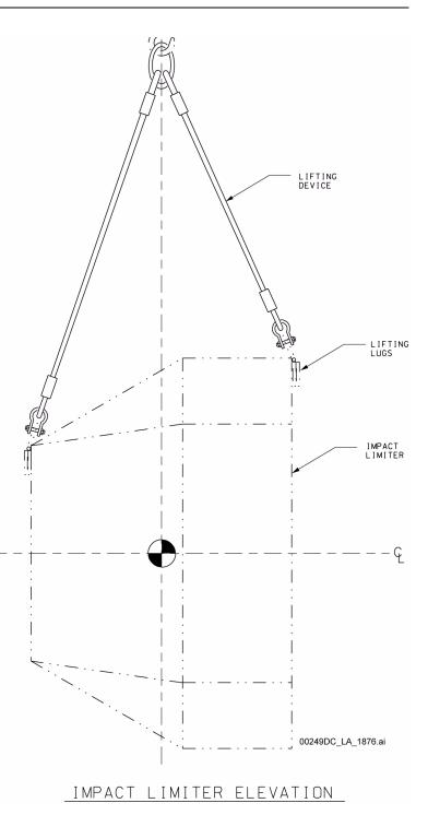
Figure 1.2.4-42. Impact Limiter Lifting Device Mechanical Equipment Envelope
