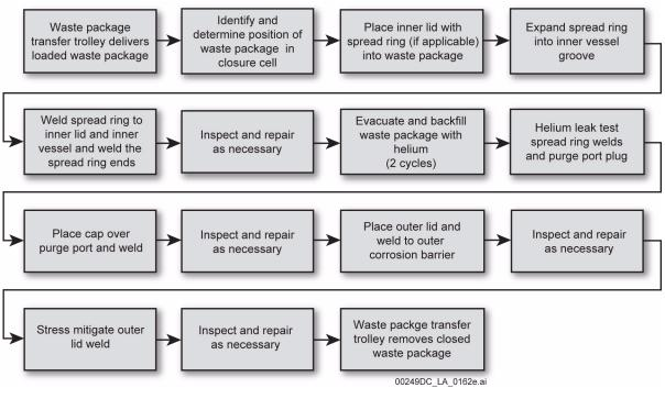
Figure 1.2.4-71. Waste Package Closure System Flow Diagram
