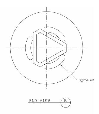
Figure 1.2.4-47. Canister Transfer Machine Canister Grapple
