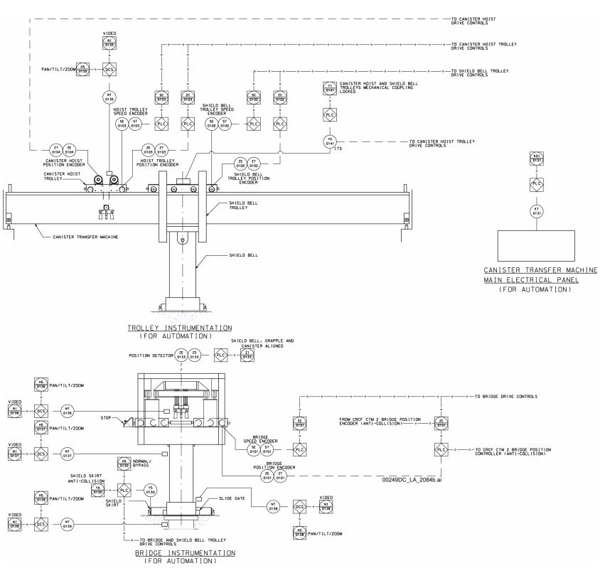
NOTE: This equipment is used in the CRCF, RF, WHF, and IHF. CTM = canister transfer machine.
