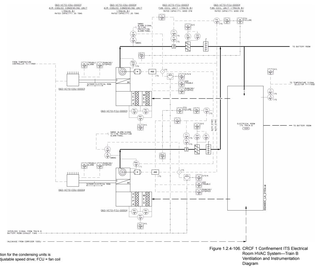
NOTE: All HVAC equipment, ductwork, and dampers are ITS. The compressor operation for the condensing units is controlled by either the battery room or electrical room temperature. ASD = adjustable speed drive; FCU = fan coil unit.
