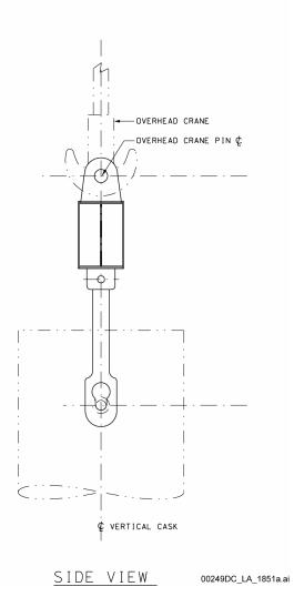
Figure 1.2.4-28. Cask Handling Yoke Mechanical Equipment Envelope
