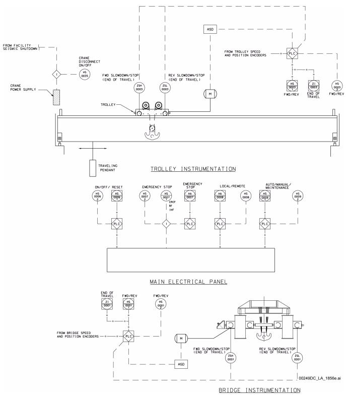
NOTE: This equipment is used in the CRCF, IHF, and RF. ASD = adjustable speed drive.
