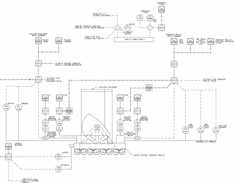
NOTE: This equipment is used in the CRCF and IHF. "A" drive motor is shown; figure is typical for "B" drive motors. PLC = programmable logic controller; WP = waste package.
