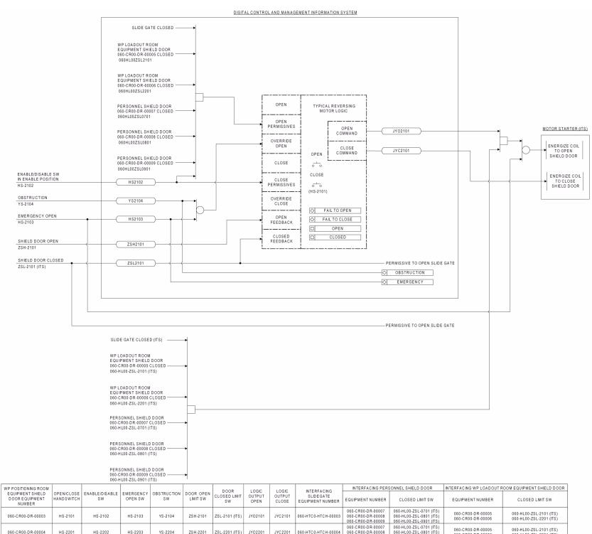
NOTE: ITS controls are identified by the letters "ITS" after the instrumentation tag number or control device identifier. The DCMIS is non-ITS and non-ITWI. Instrumentation tag numbers are prefixed by "060-HW00-" and software tag numbers are prefixed by "060HW00." WP = waste package.
