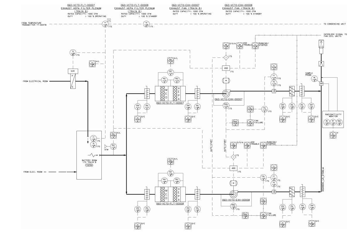
NOTE: HVAC equipment, ductwork, and all duct-mounted HVAC devices are ITS. The silicon controlled rectifier is integral to the electric heating coil and modulates heating in response to the temperature controller signal. ASD = adjustable speed drive. Figure 1.2.4-108. CRCF 1 Confinement ITS Battery Room Exhaust System—Train B Ventilation and Instrumentation Diagram
