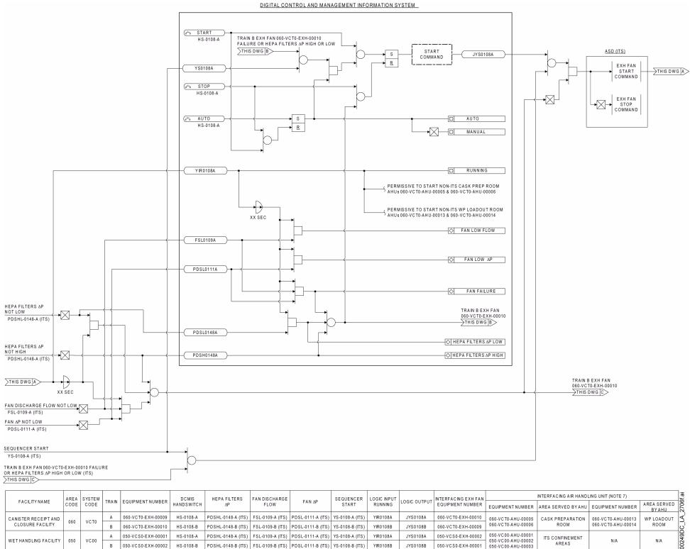
NOTE: ITS controls are identified by the letters "ITS" after the instrumentation tag number or control device identifier. The DCMIS is non-ITS and non-ITWI. Instrumentation tag numbers are prefixed by "XXX-YYYY-" and software tag numbers are prefixed by "XXXYYYY," where XXX is the area code and YYYY is the system code. AHU = air handling unit; ASD = adjustable speed drive;  $\Delta P$  = differential pressure; WP = waste package.
