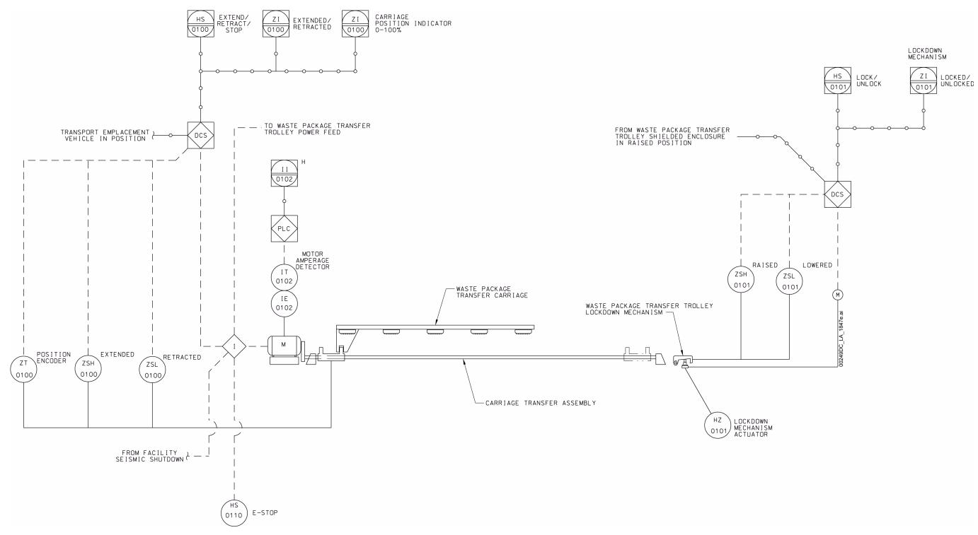
NOTE: This figure includes no SSCs that are ITS or ITWI. This equipment is used in the CRCF and IHF. A carriage transfer drive motor running signal is interlocked with the waste package transfer trolley power feed to prevent it from moving while a waste package is being transferred.
