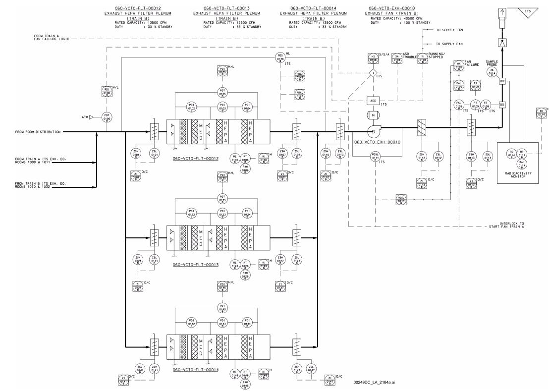
NOTE: An interlock is provided to shut down the operating fan and start the standby unit upon detection of low differential pressure across the fan coincident with low flow, a high HEPA filter train differential pressure, or a low HEPA filter train differential pressure. The HVAC equipment, ductwork, and dampers shown on this drawing are ITS. ASD = adjustable speed drive.
