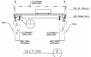
Figure 1.2.4-78. Waste Package Closure Room Crane Mechanical Equipment Envelope
