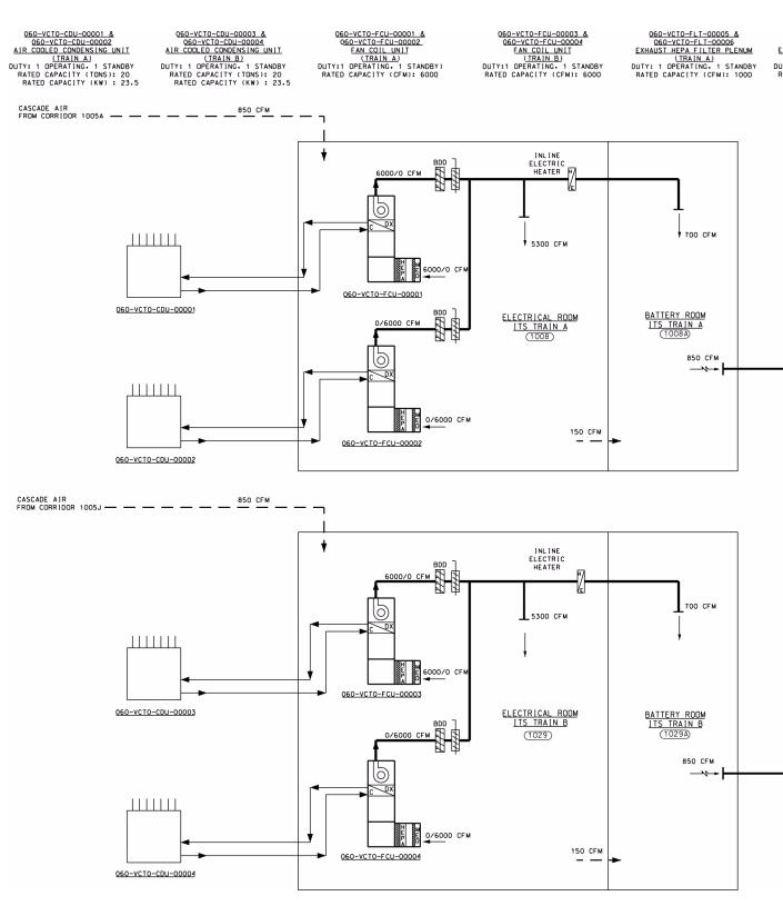
NOTE: Backup units are provided in case the operating units are down for maintenance or servicing. However, both units may be operated simultaneously as needed to maintain required room conditions during off-normal mode.
