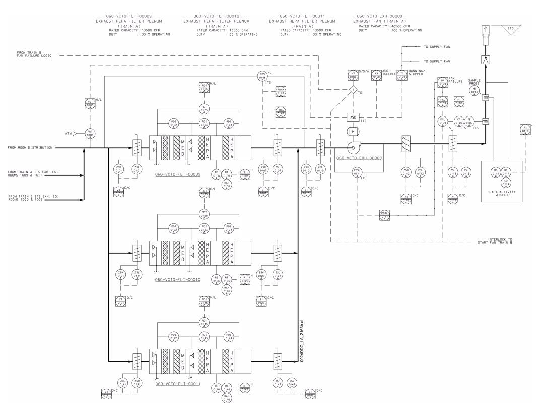
NOTE: An interlock is provided to shut down the operating fan and start the standby unit upon detection of low differential pressure across the fan coincident with low flow, a high HEPA filter train differential pressure, or a low HEPA filter train differential pressure. The HVAC equipment, ductwork, and dampers shown on this drawing are ITS. ASD = adjustable speed drive.
