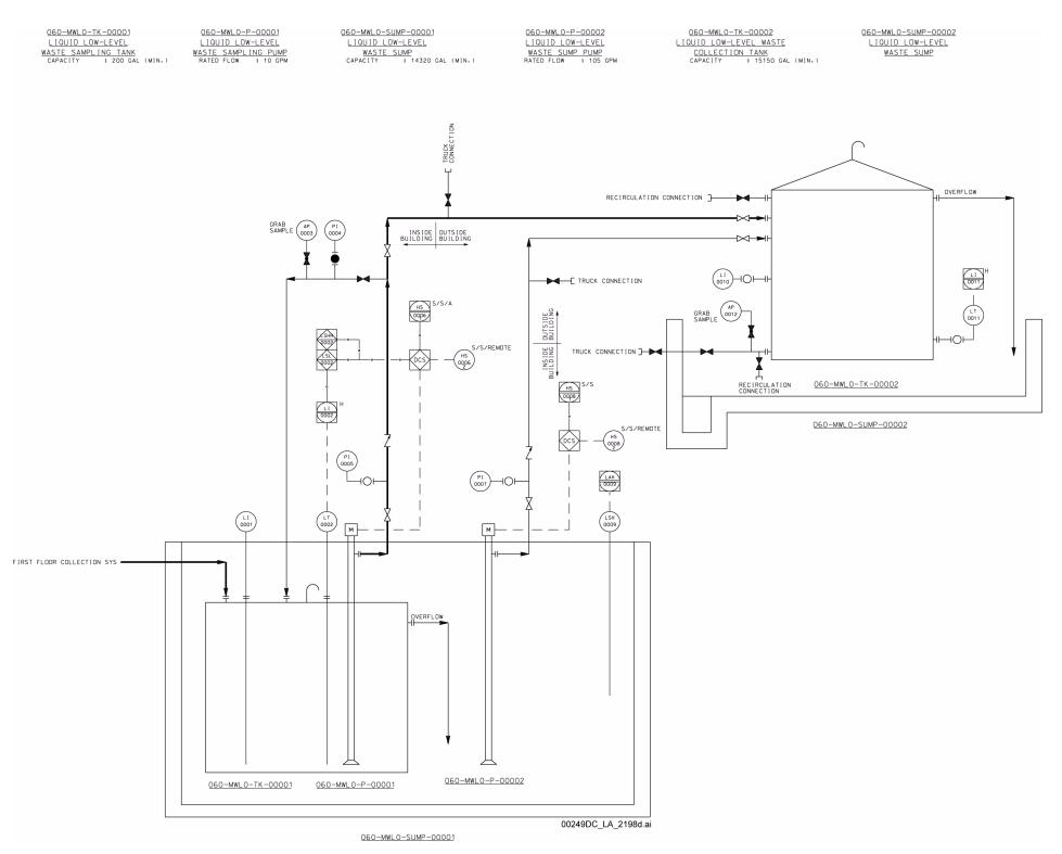
Figure 1.2.4-95. CRCF Liquid Low-Level Waste Sampling and Sump Piping and Instrumentation Diagram
