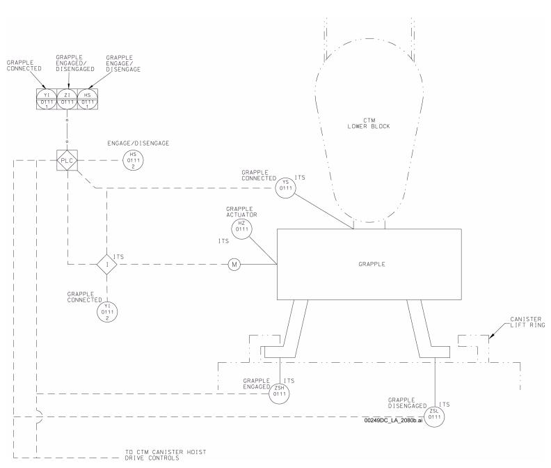
NOTE: The grapple with a suspended canister is prevented mechanically from inadvertent canister disengagement. This equipment is used in the CRCF, RF, WHF, and IHF. CTM = canister transfer machine.
