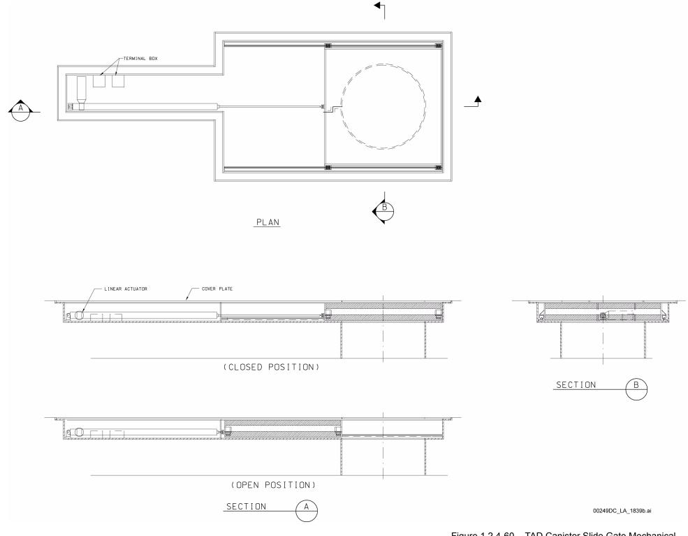
Equipment Number: 060-HTC0-HTCH-00010/00011, CRCF TAD canister slide gate.
