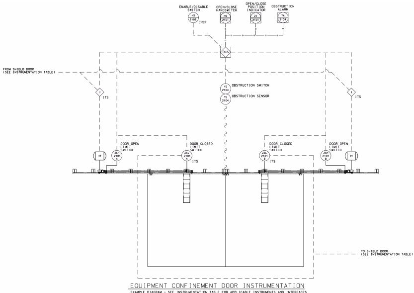
EQUIPMENT CONFINEMENT DOOR INSTRUMENTATION EXAMPLE DIAGRAM - SEE INSTRUMENTATION TABLE FOR APPLICABLE INSTRUMENTS AND INTERFACES DOUBLE DOOR SYSTEM AS SHOWN SINGLE DOOR SYSTEM SIMILAR
