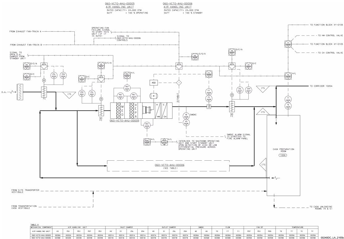
NOTE: Supply and return ductwork within the flags, including the air handling unit housing, is ITS for pressure boundary only; the air handling unit and isolation dampers do not have any ITS functions. Instrument and control devices are non-ITS.
