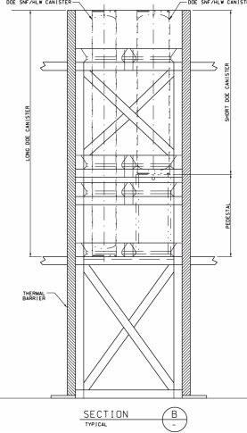
NOTE: The DOE canister staging rack assembly is configured to handle six canisters in Room 1021 and four canisters in Room 1025.
