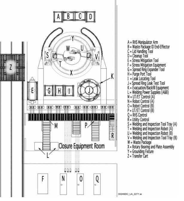
NOTE: ID = identification; RHS = remote handling system; UT/ET = ultrasonic testing/eddy current testing.
