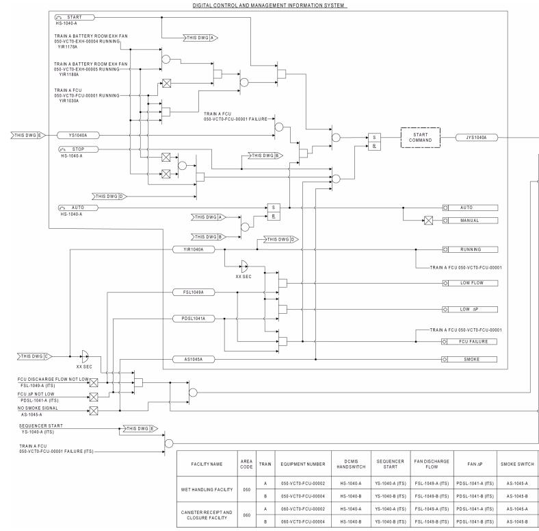
NOTE: This figure shows the logic diagram for the standby fan coil units in either Train A or Train B. ITS controls are identified by the letters "ITS" after the instrumentation tag number or control device identifier. The DCMIS is non-ITS and non-ITWI. Instrumentation tag numbers are prefixed by "XXX-VCT0-" and software tag numbers are prefixed by "XXXVCT0," where XXX is the area code. ASD = adjustable speed drive;  $\Delta P$  = differential pressure; FCU = fan coil unit.
