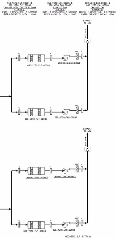
Figure 1.2.4-104. CRCF 1 Composite Ventilation Flow Diagram, Tertiary Confinement ITS HVAC Systems, Electrical and Battery Rooms
