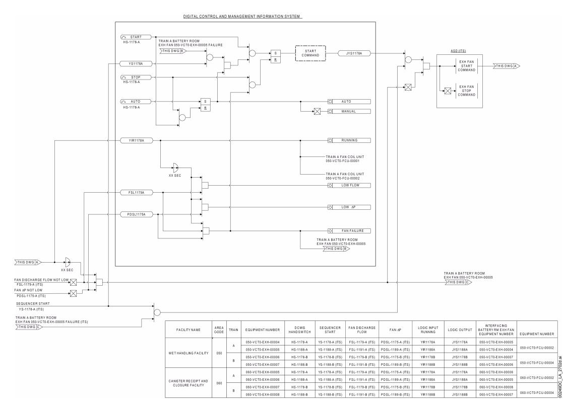
NOTE: ITS controls are identified by the letters "ITS" after the instrumentation tag number or control device identifier. The DCMIS is non-ITS and non-ITWI. Instrumentation tag numbers are prefixed by "XXX-VCT0-" and software tag numbers are prefixed by "XXXVCT0," where XXX is the area code. ASD = adjustable speed drive; ΔP = differential pressure.
