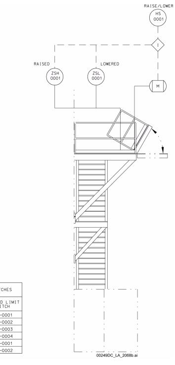
Figure 1.2.4-140. Loadout Platform Process and Instrumentation Diagram
