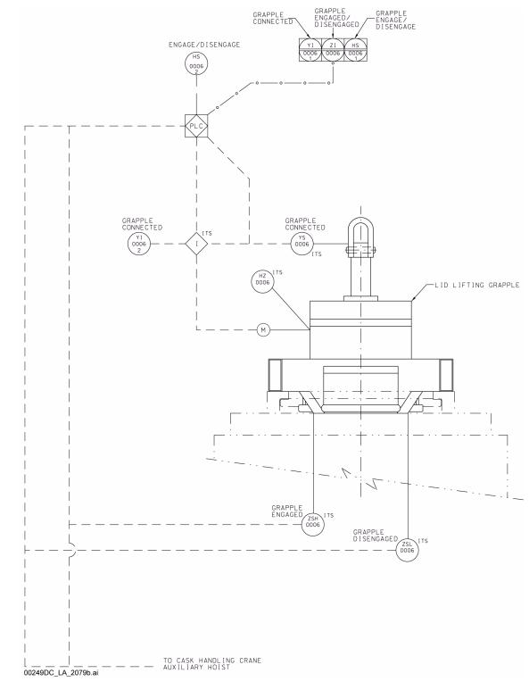
Equipment Number: 060-HMH0-HEQ-00012, CRCF cask lid-lifting grapple; 200-HMH0-HEQ-00008, RF cask lid-lifting grapple.
