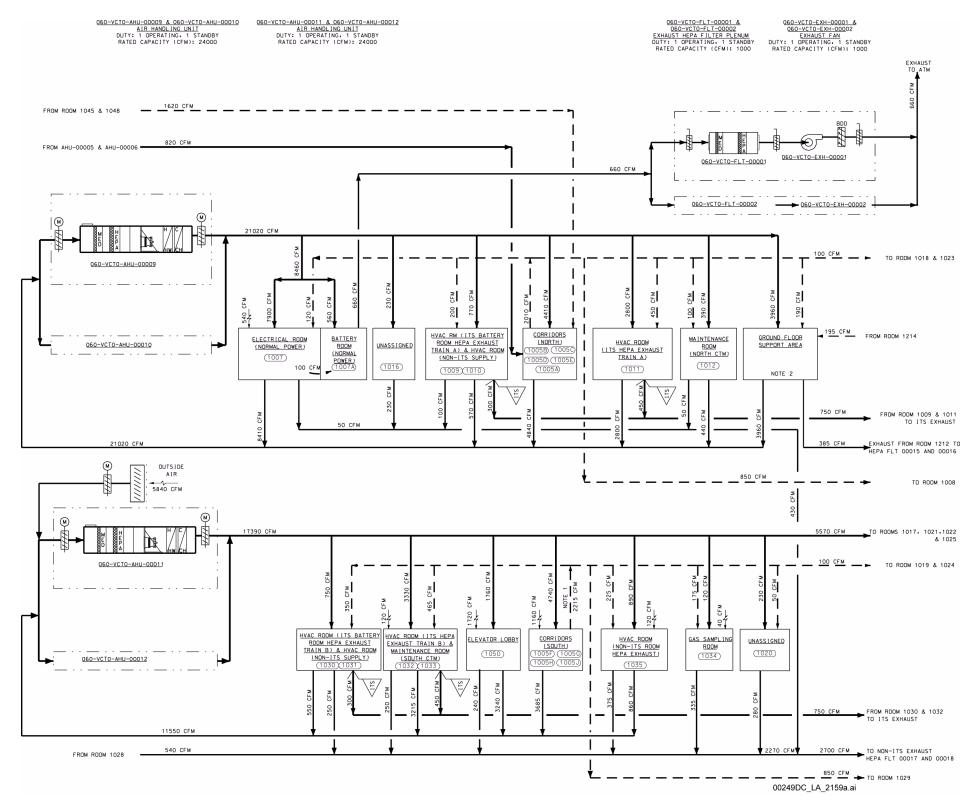
NOTE: Exhaust air is coming from the HEPA filter service gallery to the ITS exhaust system. The service gallery enclosure and the exhaust ductwork is ITS. Infiltration air to the corridor will be cascaded to adjacent rooms through doors and openings. It will be exhausted through the non-ITS HEPA filter. CTM = canister transfer machine.
