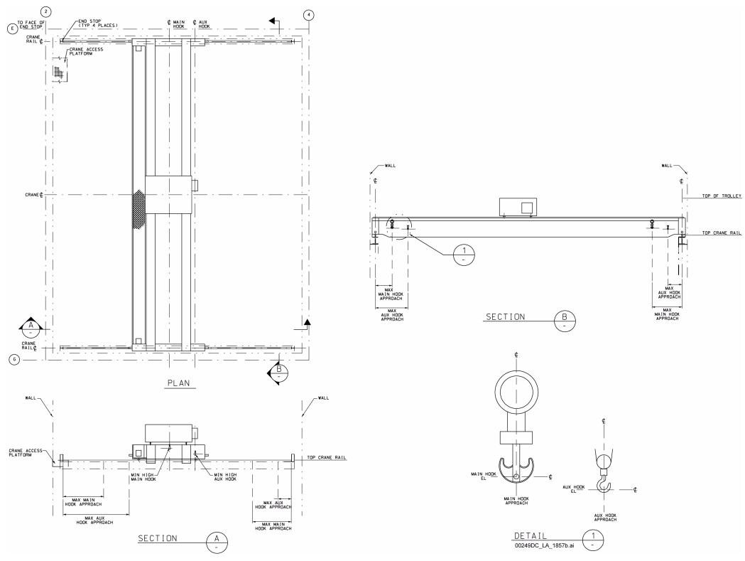
Equipment Number: 060-HMP0-CRN-00001, CRCF waste package handling crane.
