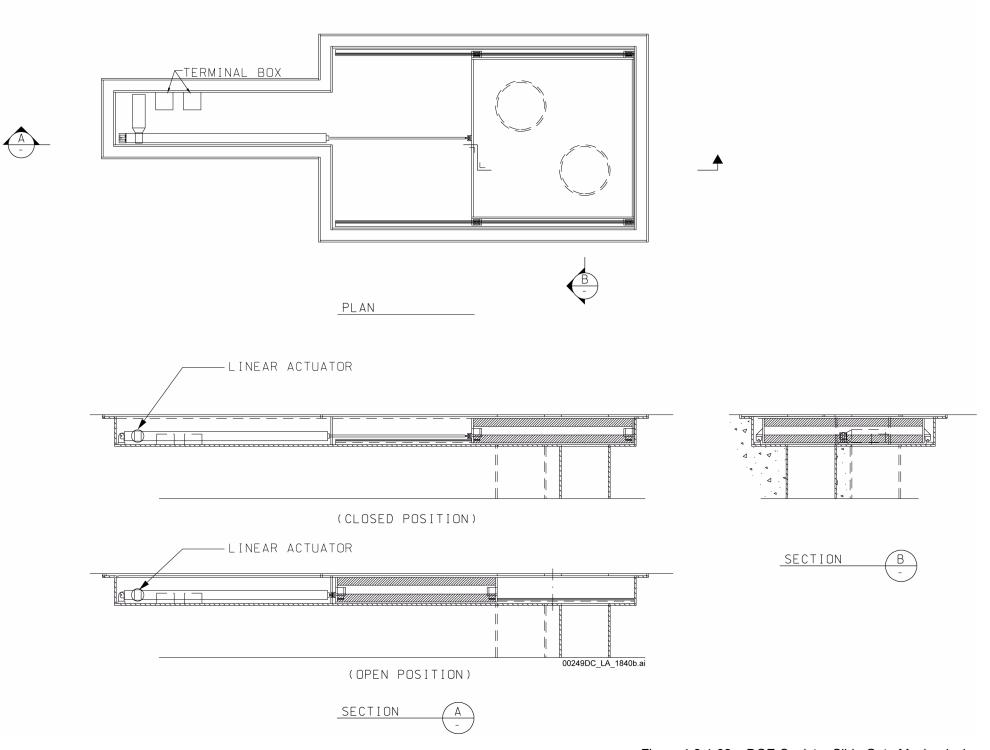
Equipment Number: 060-HTC0-HTCH-00005/00006/00007/00008/00009, CRCF DOE canister slide gates.
