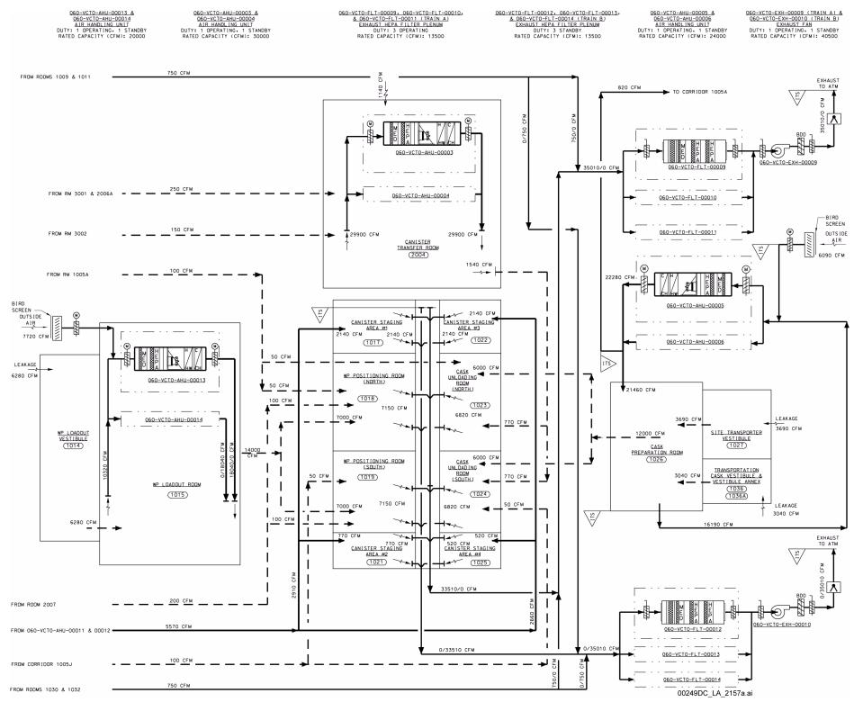
NOTE: The instrument and control devices shown on this drawing are non-ITS. The exhaust distribution ductwork is ITS, and the supply duct to the staging areas is non-ITS. WP = waste package.
