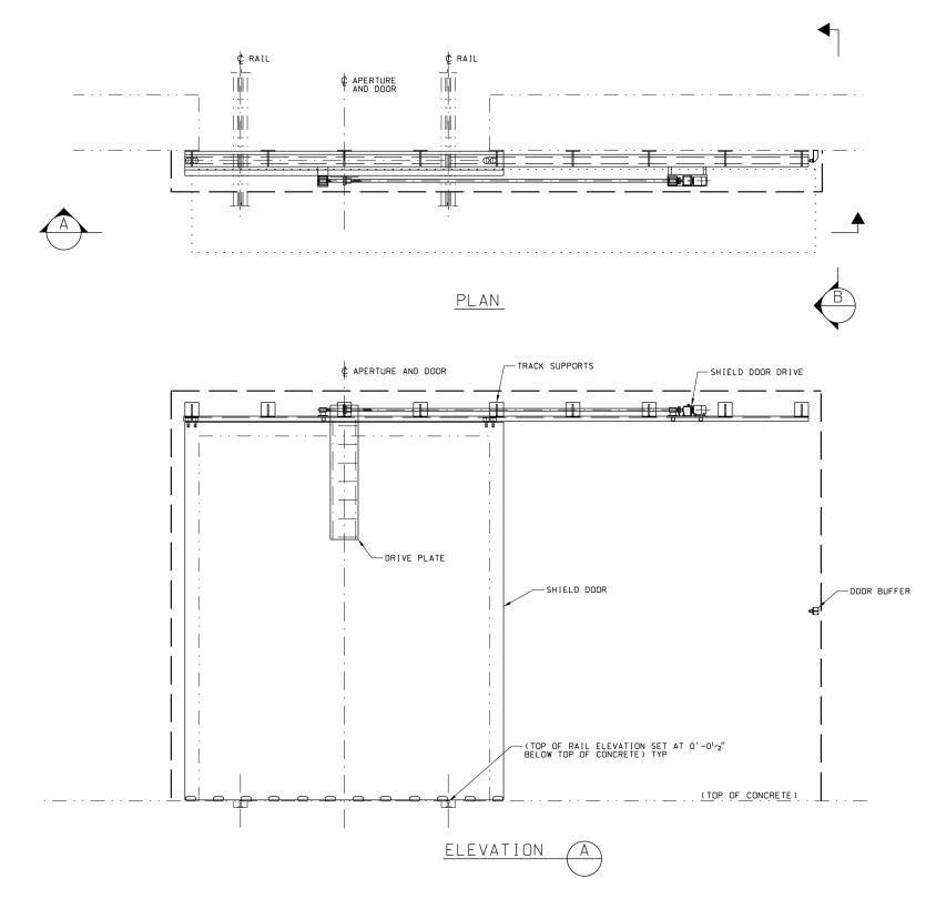
Equipment Number: 060-CR00-DR-00003/00004, CRCF waste package positioning room equipment shield door, north 1/south 2; 060-CR00-DR-00005/00006, CRCF waste package loadout room equipment shield door, door 1/door 2; 050-WH00-DR-00004, WHF site transporter vestibule equipment shield door.
