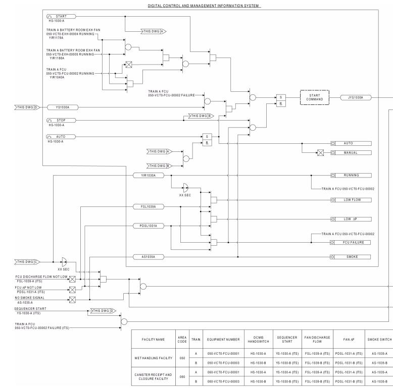
NOTE: This figure shows the logic diagram for the operating fan coil units in either Train A or Train B. ITS controls are identified by the letters "ITS" after the instrumentation tag number or control device identifier. The DCMIS is non-ITS and non-ITWI. Instrumentation tag numbers are prefixed by "XXX-VCT0-" and software tag numbers are prefixed by "XXXVCT0," where XXX is the area code.
