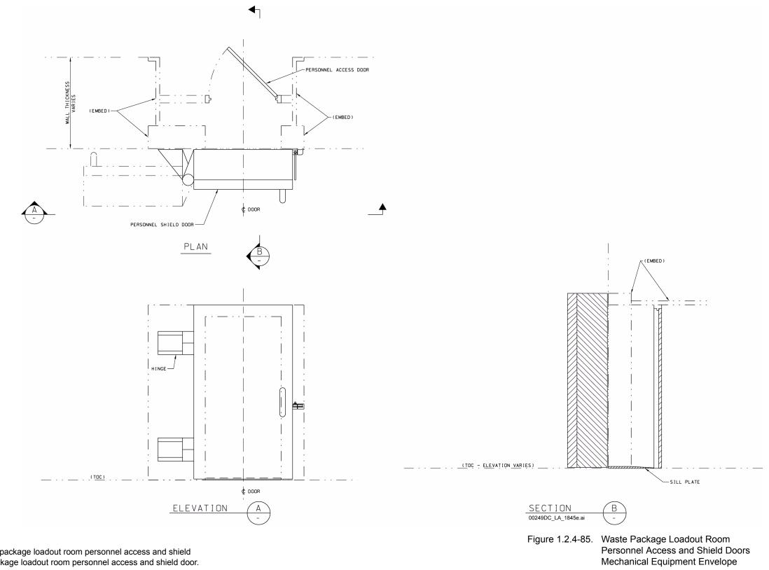
Equipment Number: 060-CR00-DR-00007/00008/00009, CRCF, waste package loadout room personnel access and shield doors; 51A-IH00-DR-00005/00006, IHF, waste package loadout room personnel access and shield door.
