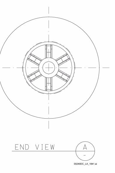
Figure 1.2.4-63. Hanford Multicanister Overpack Canister Grapple Mechanical Equipment Envelope
