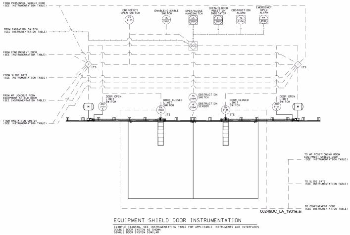
NOTE: Instrumentation tag numbers are prefixed by "XXX-YYYY-" where XXX is the area code and YYYY is the system code.
