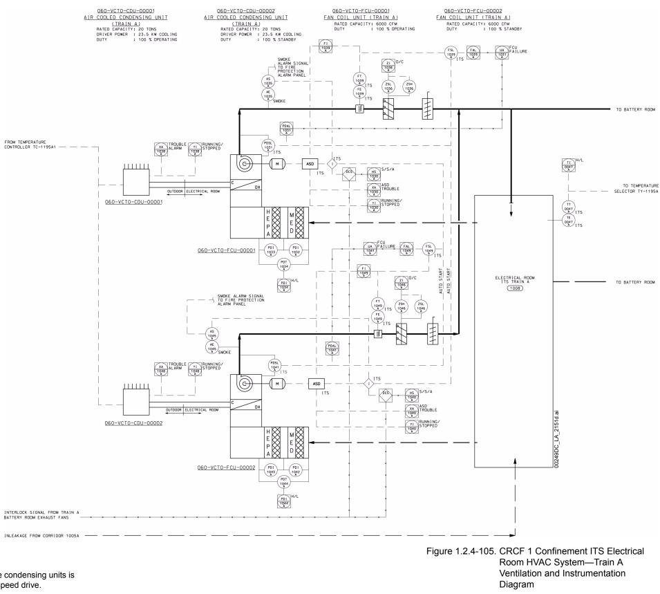
NOTE: All HVAC equipment, ductwork, and dampers are ITS. The compressor operation for the condensing units is controlled by either the battery room or electrical room temperature. ASD = adjustable speed drive.
