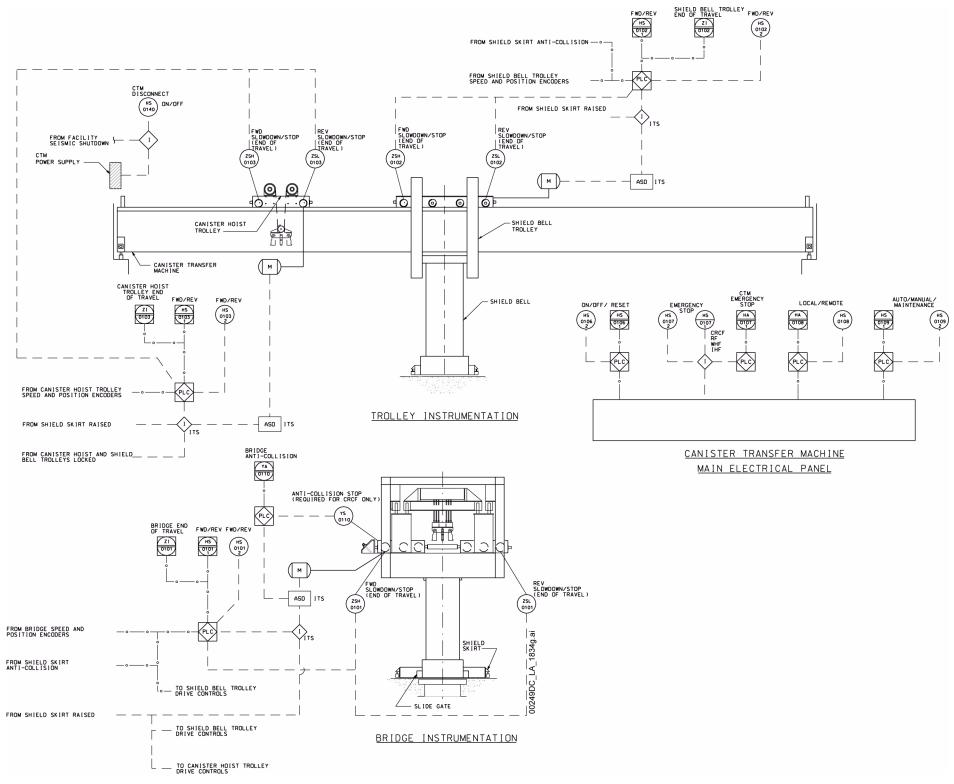
NOTE: The circuit breakers which provide power to the adjustable speed drives include instantaneous over-current protection. This feature is ITS. This equipment is used in the CRCF, RF, WHF, and IHF. CTM = canister transfer machine.
