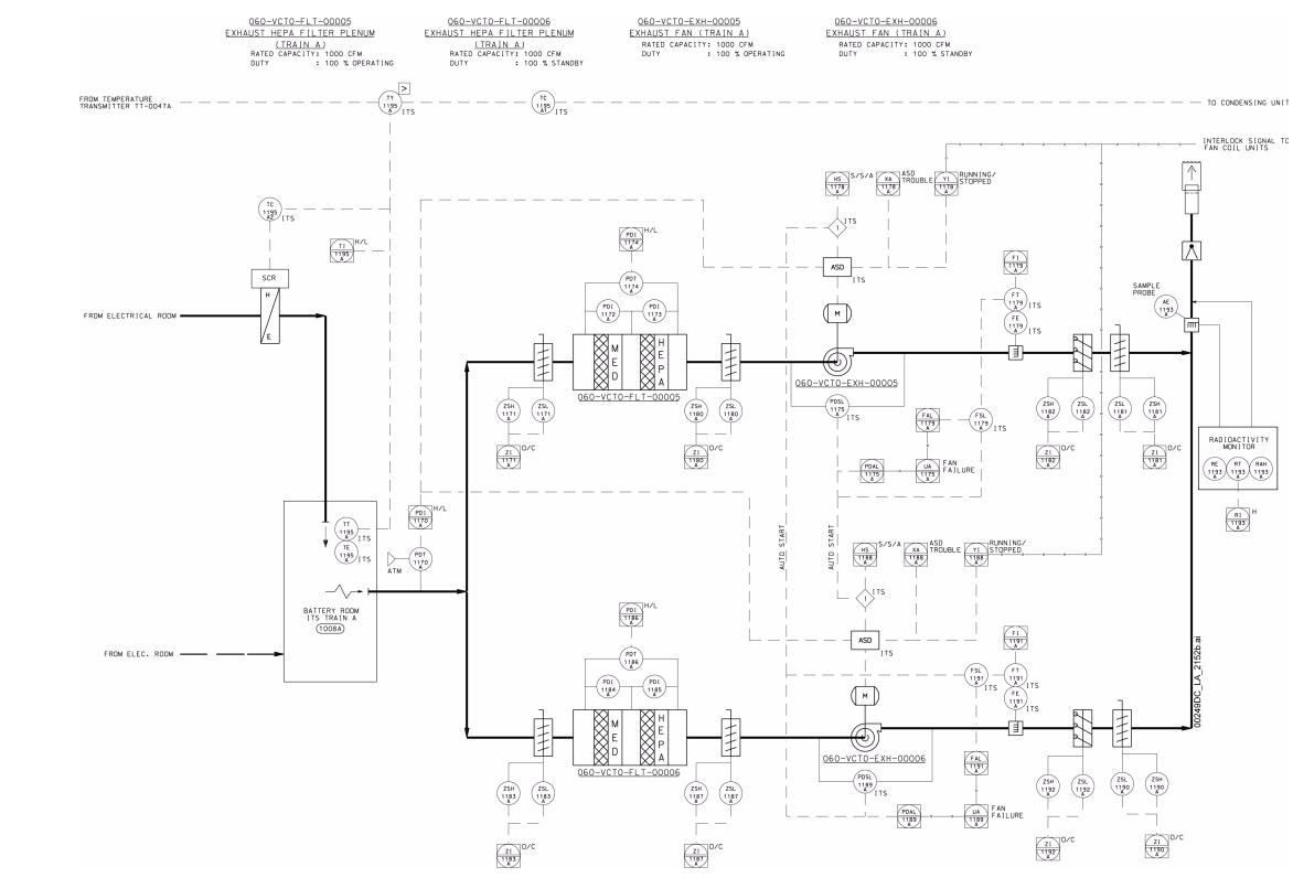
NOTE: HVAC equipment, ductwork, and all duct-mounted HVAC devices are ITS. The silicon controlled rectifier is integral to the electric heating coil and modulates heating in response to the temperature controller signal. ASD = adjustable speed drive. Figure 1.2.4-107. CRCF 1 Confinement ITS Battery Room Exhaust System—Train A Ventilation and Instrumentation Diagram
