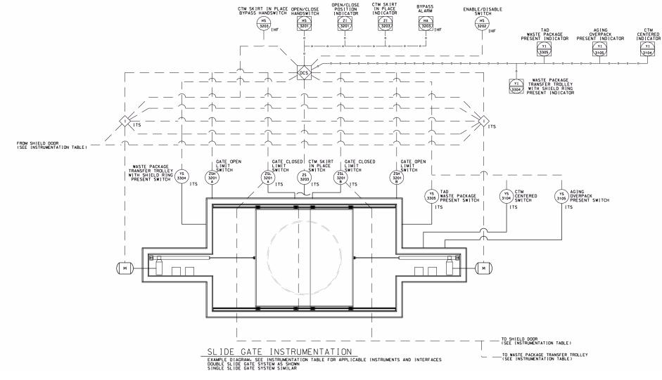
NOTE: The waste package transfer trolley with shield ring in place switch applies to the waste package port slide gates in the CRCF and IHF only. The canister transfer machine skirt in place bypass switch and alarm applies to the IHF waste package port slide gate only. This process and instrumentation diagram applies to the IHF, CRCF, WHF, and RF. CTM = canister transfer machine; WP = waste package.
