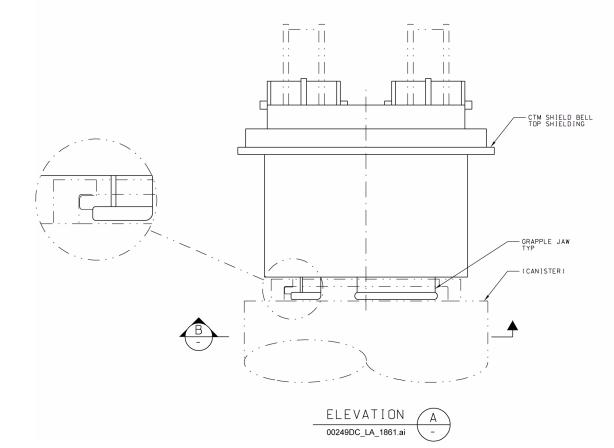
NOTE: This equipment is used in the CRCF, RF, WHF, and IHF. CTM = canister transfer machine.
