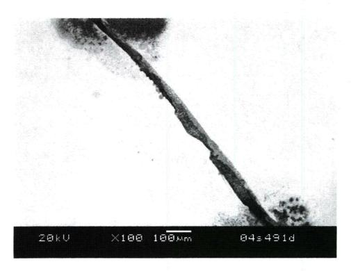
Figure B.8 Flaw C2CC on the End of Seam Repair C
