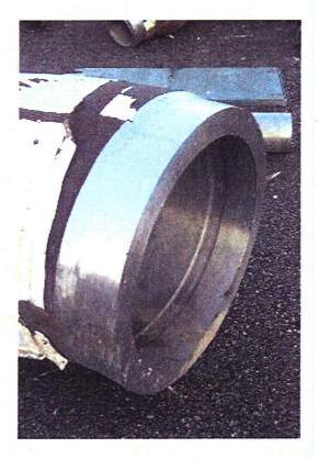
Figure 3.10 Dissimilar Metal Weld Specimen at PNNL – Safe End to 91-cm-Diameter Carbon Steel Elbow Weld
