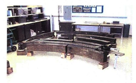
Figure 3.6 Shoreham Specimens in the PNNL NDE Laboratory, Prepared for Weld-Normal Inspection
