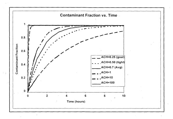
**Figure 5.2** - Plot of Equation 1 for a wider range of ACH values, where ACH=0.25 represents PS and ACH=0.7 represents SIP.
