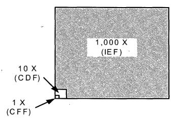
**Figure 3.6** - Relative magnitudes of Initiating Event Frequency (IEF), Core Damage Frequency (CDF), and Containment Failure Frequency (CFF) for LOSPs and LOCAs based on NUREG-1150 site risk analysis reports for the Surry, Sequoyah, Grand Gulf and Peach Bottom reactors.
