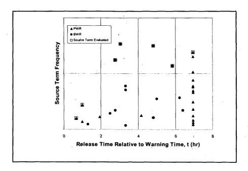
**Figure 3.2** - Higher frequency short time scale source terms for internally and externally initiated events at Surry, Sequoyah, Grand Gulf, Peach Bottom and LaSalle. Boxes indicate those source terms evaluated for potential use in the protective action recommendation study.
