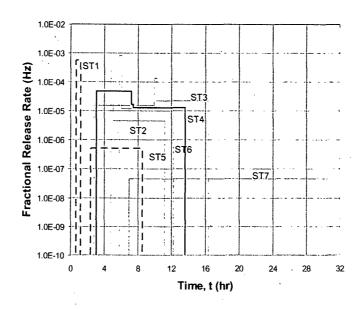
**Figure 3.3** - Noble gas releases associated with highest frequency and shortest time scale source terms at Surry, Sequoyah, and LaSalle.
