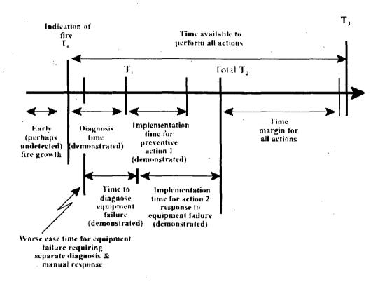
Figure A-2. Initial fire detection and multiple action (one action dependent on a separate diagnosis of an undesired equipment faulure) with a single overall time margin and T<sub>3</sub>
