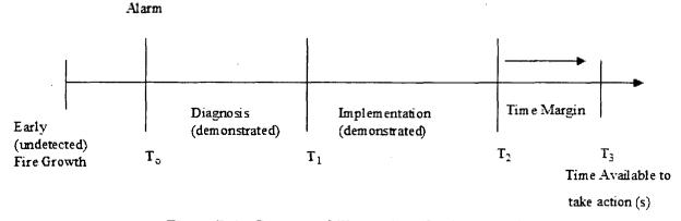
Figure B-1. Conceptual illustration of a time margin
