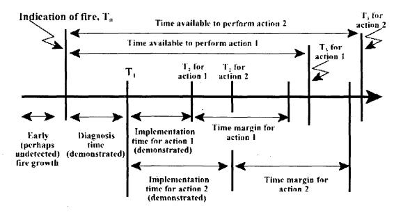
Figure A-4. Initial fire detection and multiple actions illustrating the application of multiple time margins and T<sub>3</sub>s
