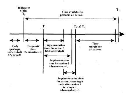
Figure A-3. Initial fire detection and multiple actions (one action dependent on completion of a prior action) with a single overall time margin and  ${\rm T}_3$
