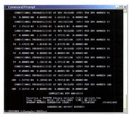
Fig. 15. Type in FAVPost at the MS DOS Prompt to execute the FAVPost module.
