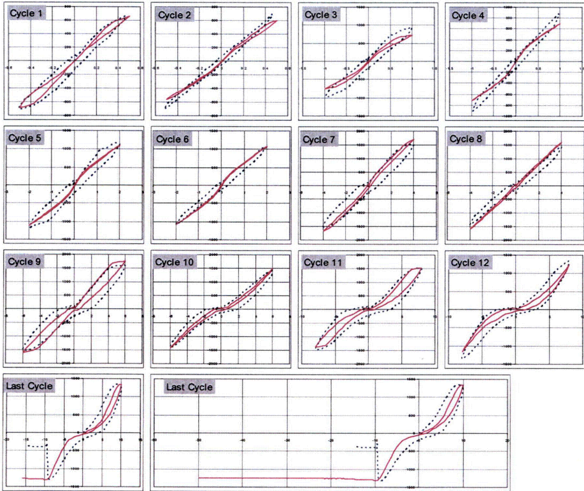
Figure 4-30 Cycle-By-Cycle Q_x - D_x Relation For Cross Loading
