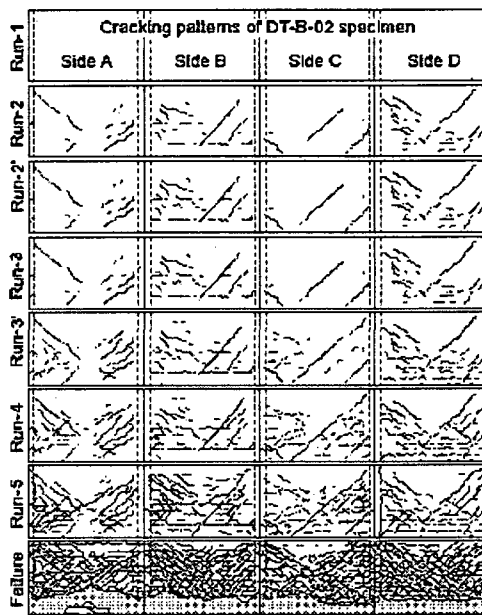
Figure 2-51 Progressive Development of Shear Wall Cracks for DT-B-02
