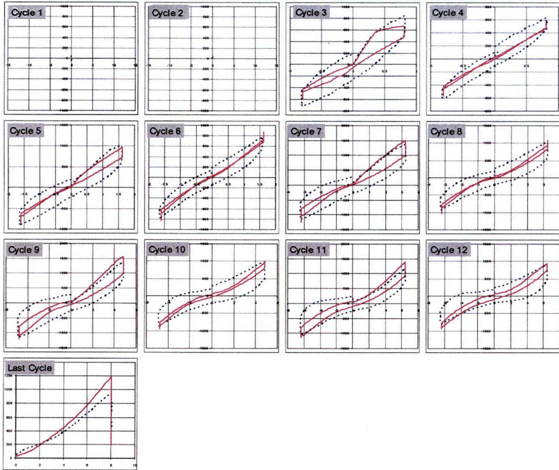
Figure 4-25 Cycle-By-Cycle Q_y - D_y Relation For Rectangular Loading
