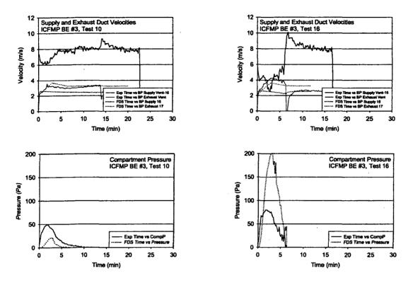
Figure 6-10: Ventilation Rates and Pressures for BE #3, Tests 10 and 16
