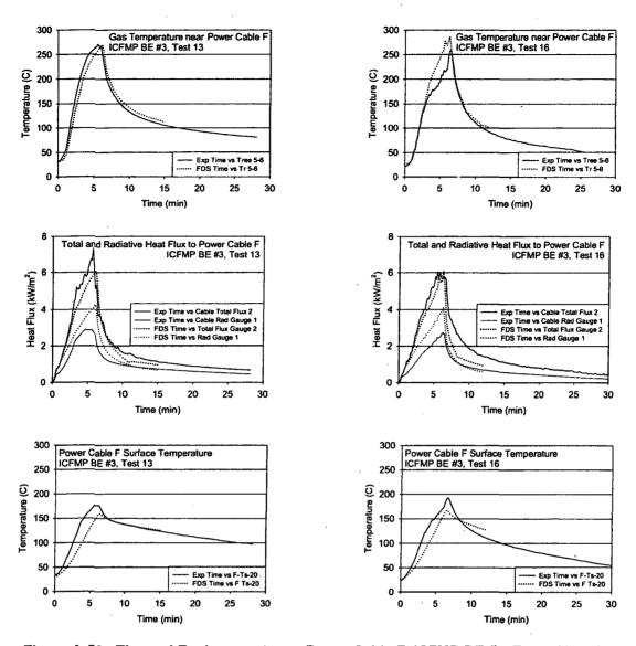
Figure A-50: Thermal Environment near Power Cable F, ICFMP BE #3, Tests 13 and 16
