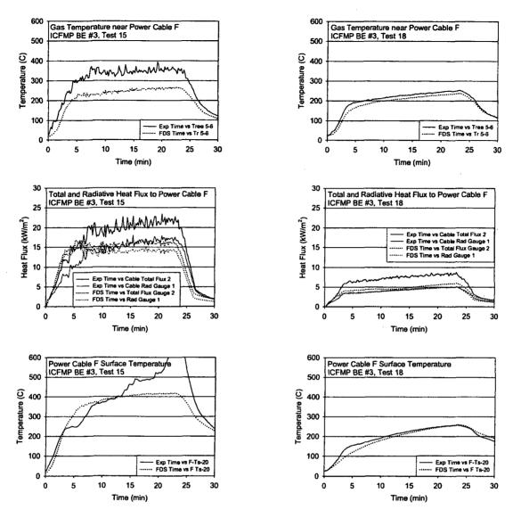
Figure A-53: Thermal Environment near Power Cable F, ICFMP BE #3, Tests 15 and 18
