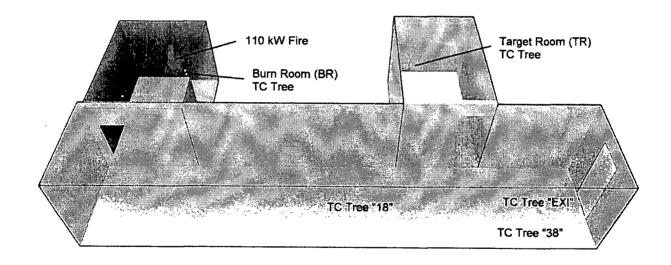
Figure A-14: Snapshot of the Simulation of NBS Multi-Room Test 100Z
