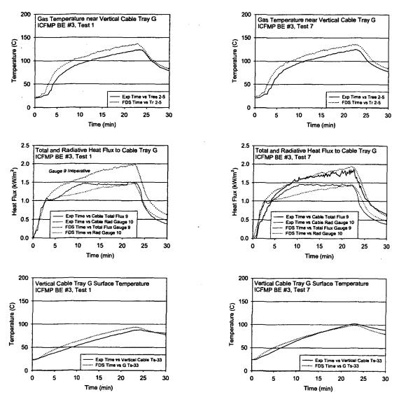
Figure A-54: Thermal Environment near Vertical Cable Tray G, ICFMP BE #3, Tests 1 and 7
