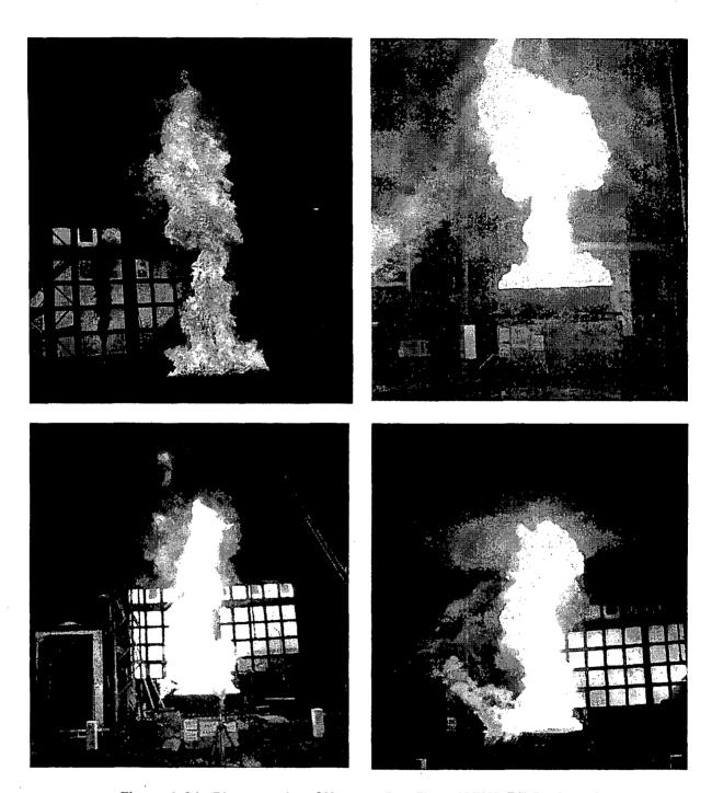
Figure A-24: Photographs of Heptane Pan Fires, ICFMP BE #2, Case 2 (Courtesy of Simo Hostikka, VTT Building and Transport, Espoo, Finland.)
