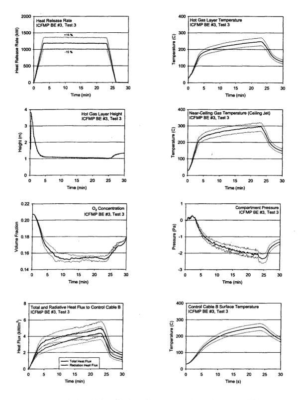
Figure 5-4: Sensitivity of Various Output Quantities to Changes in HRR
