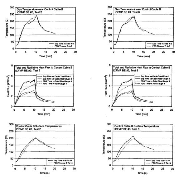
Figure A-34: Thermal Environment near Cable B, ICFMP BE #3, Tests 2 and 8
