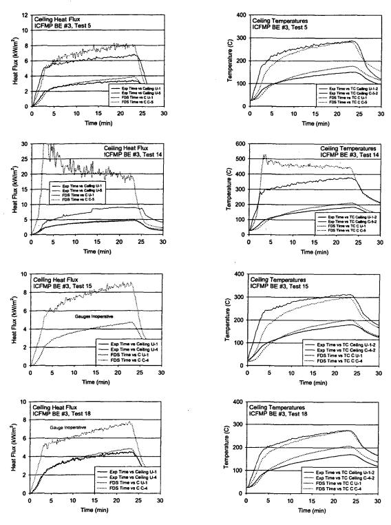
Figure A-77: Ceiling Heat Flux and Surface Temperature, ICFMP BE #3, Open-Door Tests
