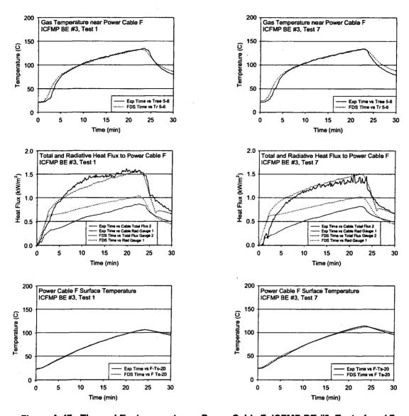
Figure A-47: Thermal Environment near Power Cable F, ICFMP BE #3, Tests 1 and 7
