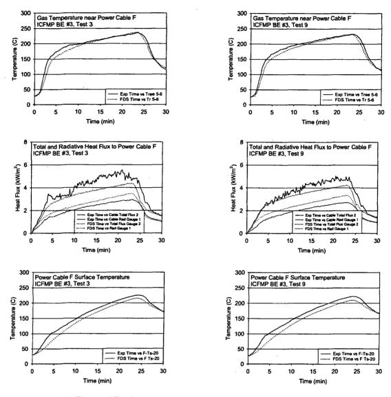
Figure A-51: Thermal Environment near Power Cable F, ICFMP BE #3, Tests 3 and 9
