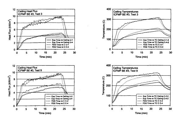
Figure A-76: Ceiling Heat Flux and Surface Temperature, ICFMP BE #3, Open-Door Tests
