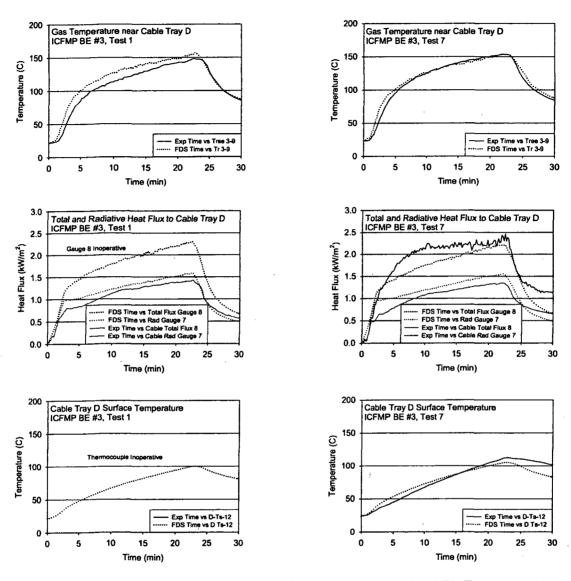
Figure A-40: Thermal Environment near Cable Tray D, ICFMP BE #3, Tests 1 and 7
