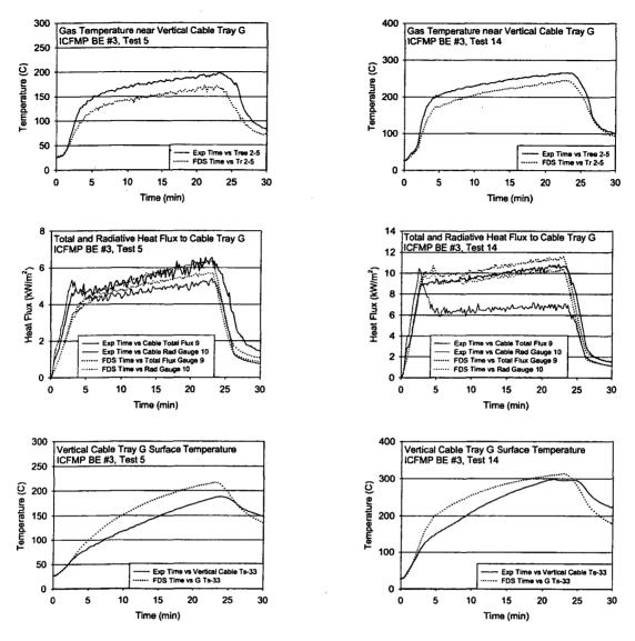
Figure A-59: Thermal Environment near Vertical Cable Tray G, ICFMP BE #3, Tests 5 and 14
