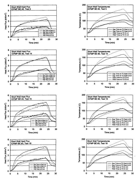
Figure A-73: Short-Wall Heat Flux and Surface Temperature, ICFMP BE #3, Open-Door Tests
