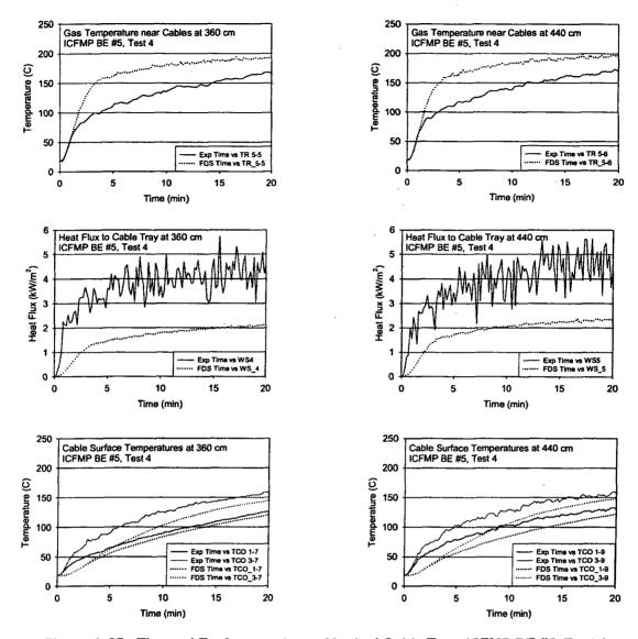
Figure A-65: Thermal Environment near Vertical Cable Tray, ICFMP BE #5, Test 4
