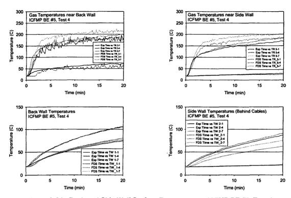
Figure A-84: Back and Side Wall Surface Temperatures, ICFMP BE #5, Test 4
