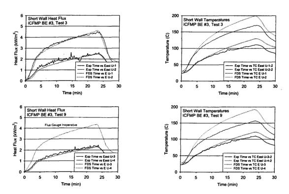
Figure A-72: Short-Wall Heat Flux and Surface Temperature, ICFMP BE #3, Open-Door Tests
