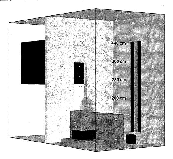
Figure A-63: Location of Targets, ICFMP BE #5, Test 4
