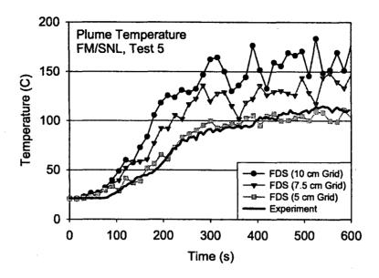
Figure 5-1: Grid Sensitivity Study for FM/SNL Test 5
