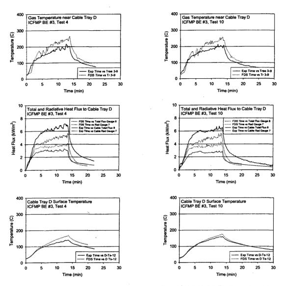
Figure A-42: Thermal Environment near Cable Tray D, ICFMP BE #3, Tests 4 and 10
