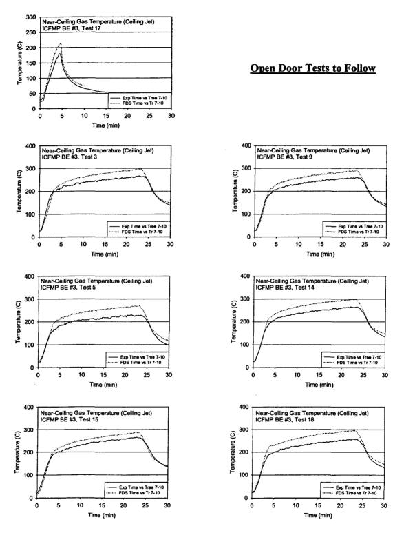
Figure A-19: Near-Ceiling Gas Temperatures, ICFMP BE #3, Closed-Door Tests
