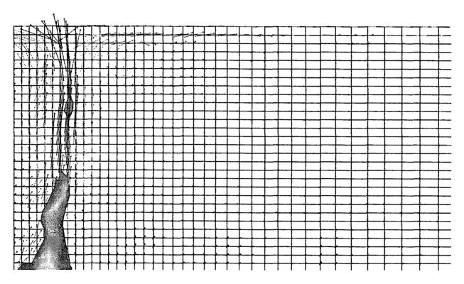
Figure 6-4: Snapshot of FDS Simulation of ICFMP BE #3, Test 3
