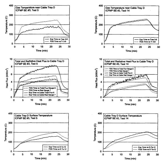
Figure A-45: Thermal Environment near Cable Tray D, ICFMP BE #3, Tests 5 and 14
