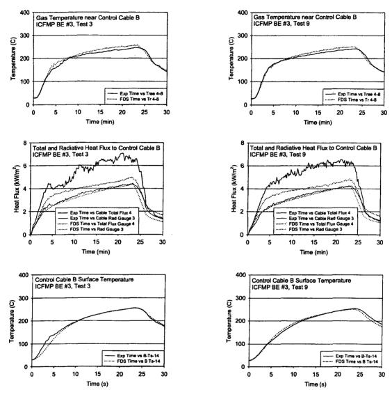
Figure A-37: Thermal Environment near Cable B, ICFMP BE #3, Tests 3 and 9
