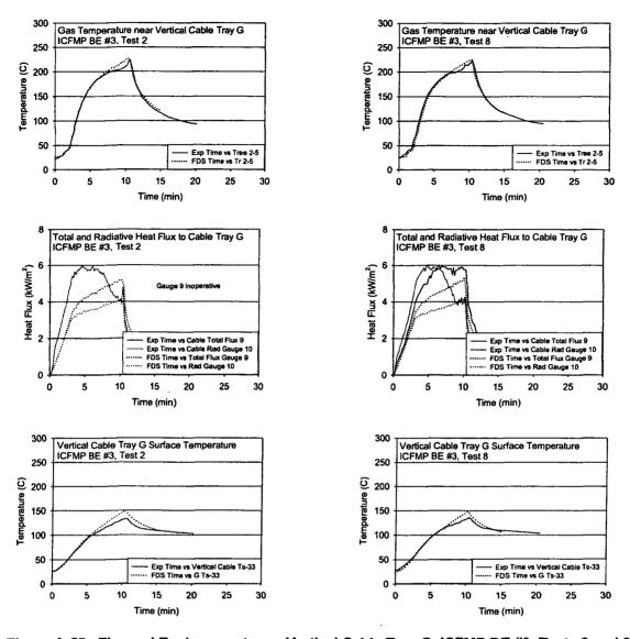
Figure A-55: Thermal Environment near Vertical Cable Tray G, ICFMP BE #3, Tests 2 and 8
