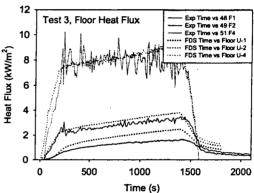
Figure 5-3: ICFMP BE #3 Test 3 Results Using 200 Radiation Angles (Left) and 100 (Right)
