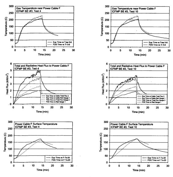
Figure A-49: Thermal Environment near Power Cable F, ICFMP BE #3, Tests 4 and 10
