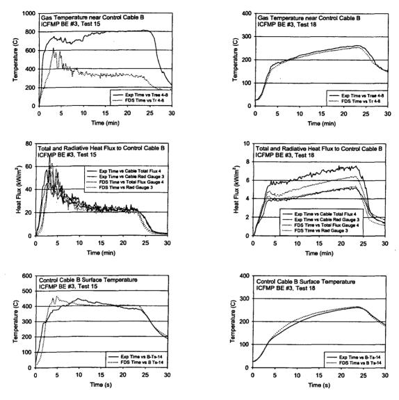
Figure A-39: Thermal Environment near Cable B, ICFMP BE #3, Tests 15 and 18 (Note that the cable was very close to the fire in Test 15.)
