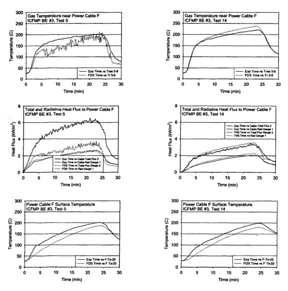
Figure A-52: Thermal Environment near Power Cable F, ICFMP BE #3, Tests 5 and 14
