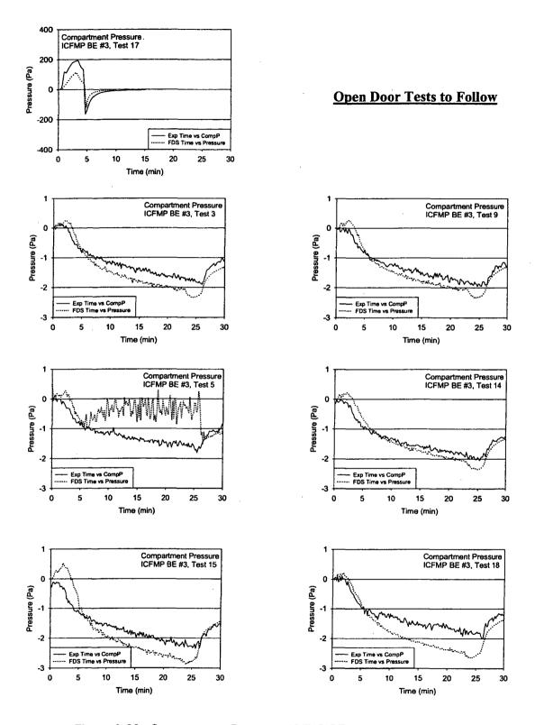
Figure A-32: Compartment Pressure, ICFMP BE #3, Open-Door Tests
