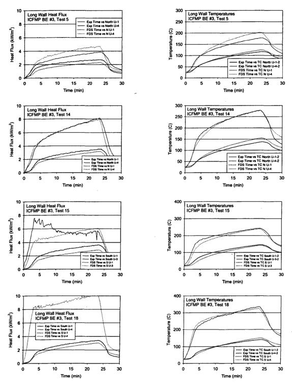
Figure A-69: Long-Wall Heat Flux and Surface Temperature, ICFMP BE #3, Open-Door Tests
