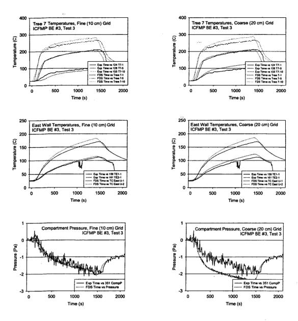
Figure 5-2: Fine (Left) and Coarse (Right) Simulations of ICFMP BE #3, Test 3
