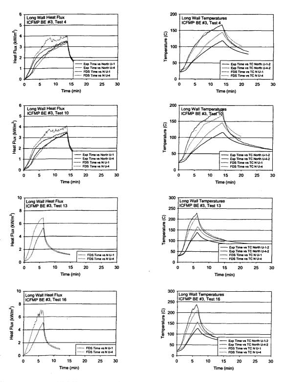
Figure A-67: Long-Wall Heat Flux and Surface Temperature, ICFMP BE #3, Closed-Door Tests
