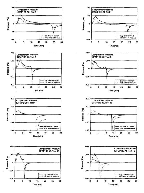
Figure A-31: Compartment Pressure, ICFMP BE #3, Closed-Door Tests
