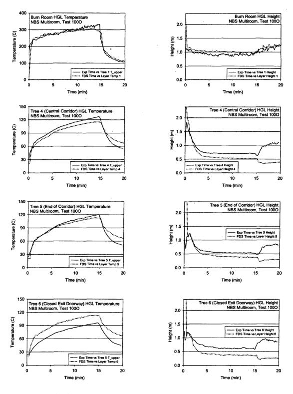
Figure A-16: Hot Gas Layer (HGL) Temperature and Height, NBS Multi-Room Test 100O
