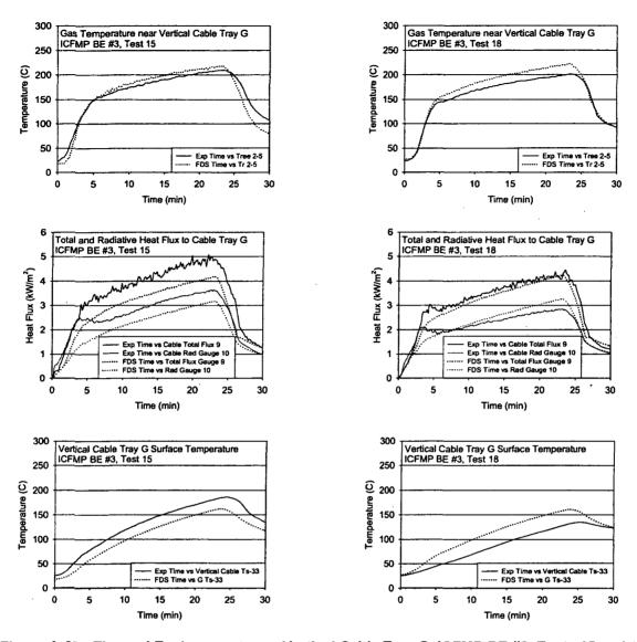
Figure A-60: Thermal Environment near Vertical Cable Tray G, ICFMP BE #3, Tests 15 and 18
