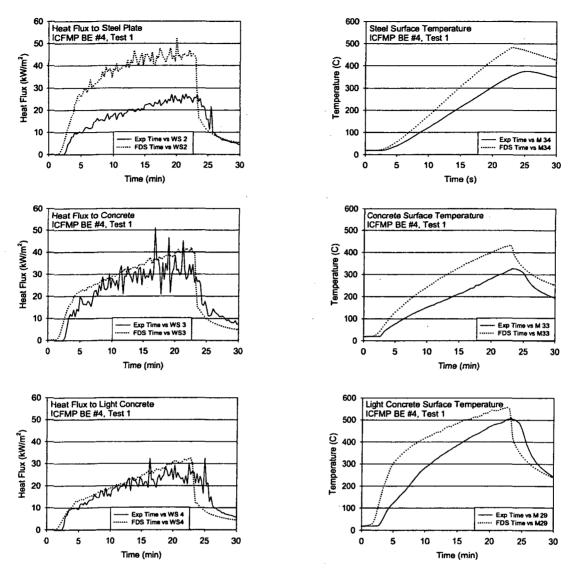
Figure A-62: Heat Flux and Surface Temperatures of Target Slabs, ICFMP BE #4, Test 1
