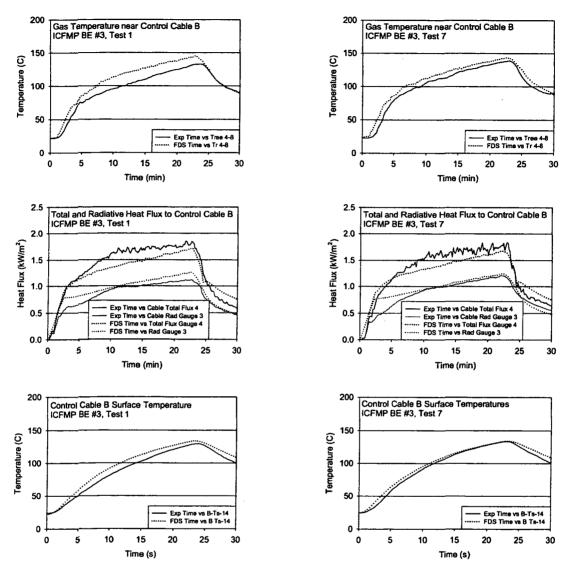
Figure A-33: Thermal Environment near Cable B, ICFMP BE #3, Tests 1 and 7
