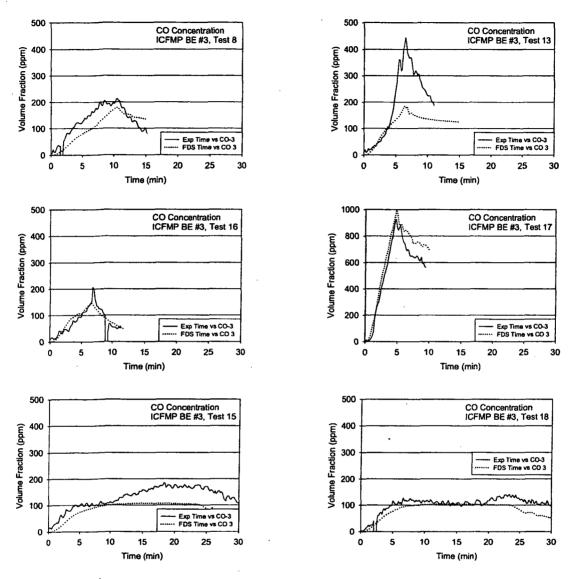
Figure A-30: CO Concentration, ICFMP BE #3, Closed Door (Top Four) and Open Door (Bottom Two) Tests
