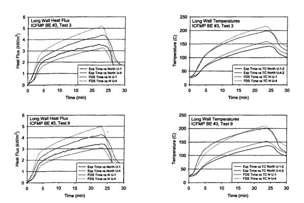
Figure A-68: Long-Wall Heat Flux and Surface Temperature, ICFMP BE #3, Closed-Door Tests
