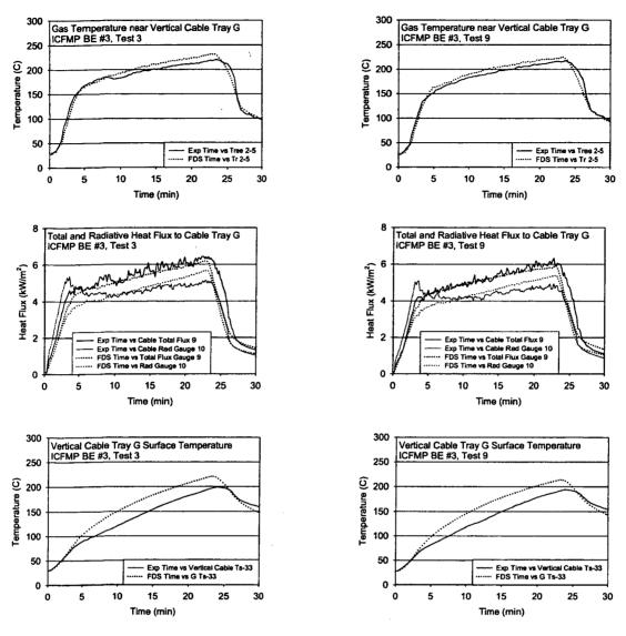
Figure A-58: Thermal Environment near Vertical Cable Tray G, ICFMP BE #3, Tests 3 and 9
