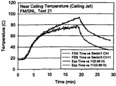
Figure A-20: Near-Ceiling Gas Temperatures, FM/SNL Series, Sectors 1 and 3
