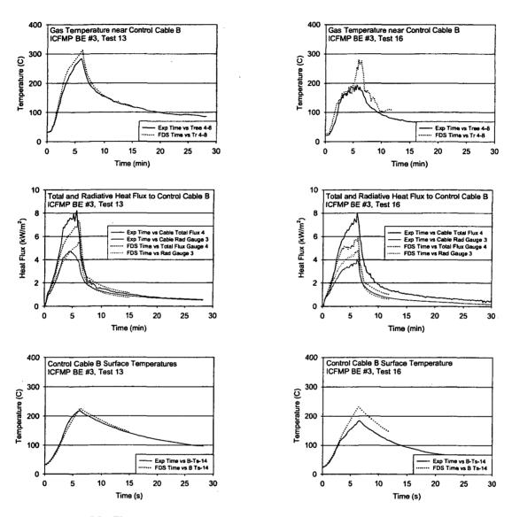
Figure A-36: Thermal Environment near Cable B, ICFMP BE #3, Tests 13 and 16 (Note the influence of the fan in Test 16.)
