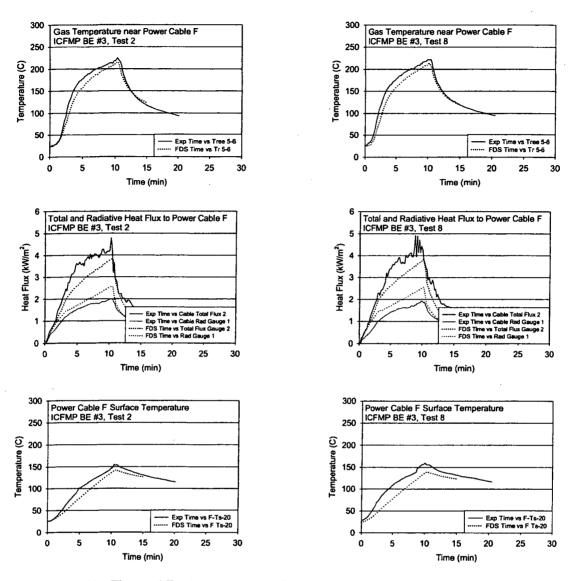
Figure A-48: Thermal Environment near Power Cable F, ICFMP BE #3, Tests 2 and 8
