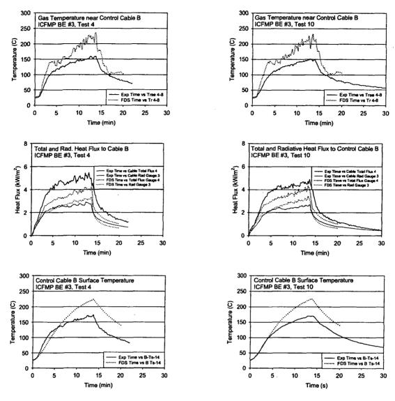
Figure A-35: Thermal Environment near Cable B, ICFMP BE #3, Tests 4 and 10 (Note the influence of the fan on the gas and surface temperatures.)
