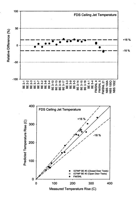
Figure 6-3: Summary of FDS Predictions of Ceiling Jet Temperature
