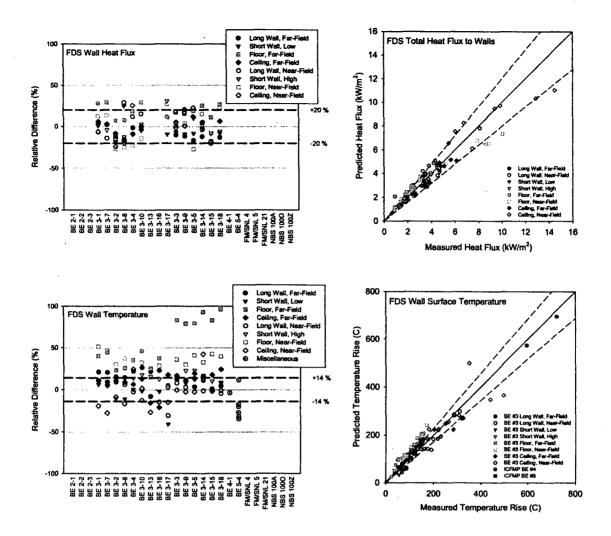
Figure 6-12: Summary of FDS Predictions of Wall Heat Flux and Temperature
