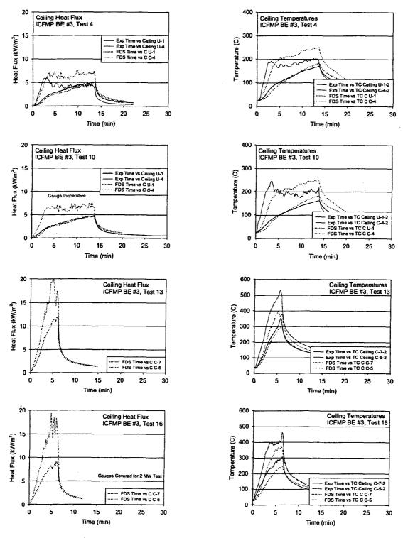
Figure A-75: Ceiling Heat Flux and Surface Temperature, ICFMP BE #3, Closed-Door Tests
