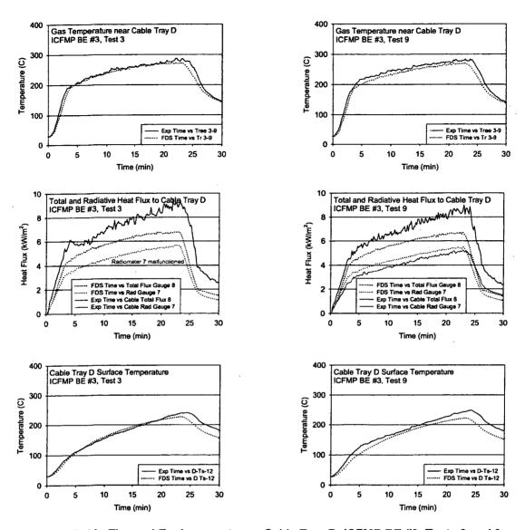
Figure A-44: Thermal Environment near Cable Tray D, ICFMP BE #3, Tests 3 and 9
