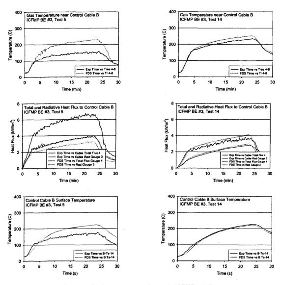
Figure A-38: Thermal Environment near Cable B, ICFMP BE #3, Tests 5 and 14 (Note the influence of the fan in Test 5.)
