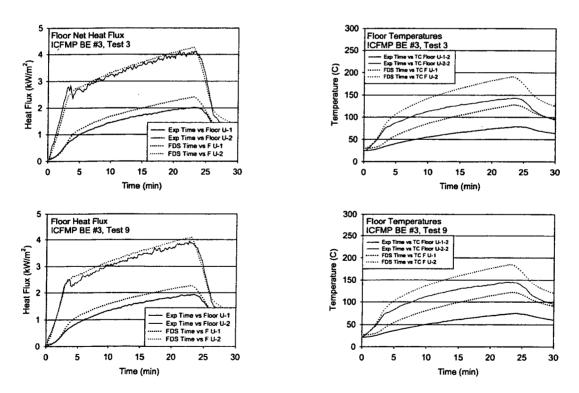
Figure A-80: Floor Heat Flux and Surface Temperature, ICFMP BE #3, Open-Door Tests
