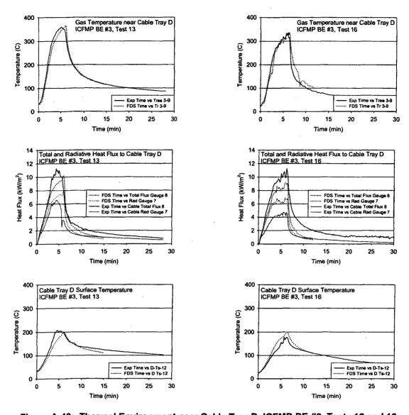
Figure A-43: Thermal Environment near Cable Tray D, ICFMP BE #3, Tests 13 and 16
