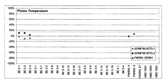
Figure 6-3: Scatter Plot of Relative Differences for Plume Temperatures in ICFMP BE #2, and the Selected FM/SNL Tests (Experimental uncertainty is 14%.)
