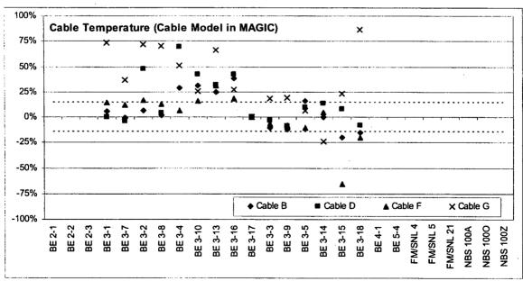
Figure 6-8: Scatter Plot of Relative Differences for Target Temperature in ICFMP BE #3 (Experimental uncertainty is 14%.)
