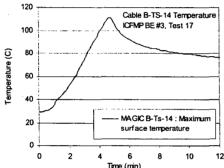
Figure A-40: Thermal Environment near Cable B, ICFMP BE #3, Test 17
