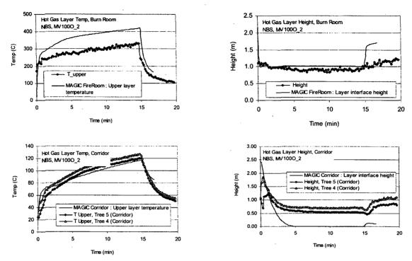
Figure A-16: Hot Gas Layer (HGL) Temperature and Height, NBS Multiroom Test 1000
