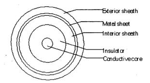
Figure 3-2: Simplified Inner Structure of an Armored Electrical Cable
