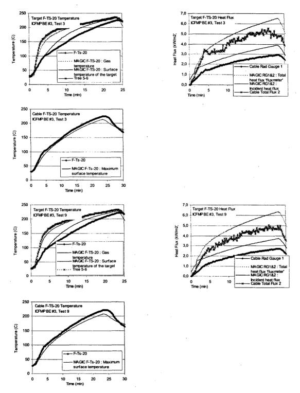
Figure A-57: Thermal Environment near Cable F, ICFMP BE #3, Tests 3 and 9
