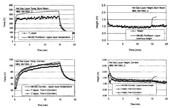
Figure A-15: Hot Gas Layer (HGL) Temperature and Height, NBS Multiroom Test 100A.
