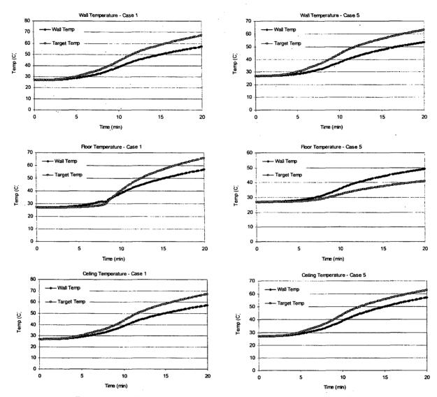
Figure 5-14: Target Temperature vs. Wall Temperature, 1-MW Fire
