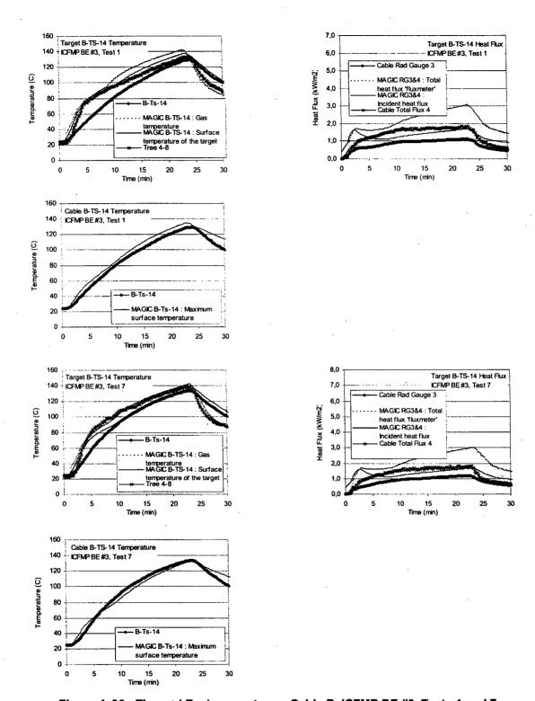
Figure A-36: Thermal Environment near Cable B, ICFMP BE #3, Tests 1 and 7
