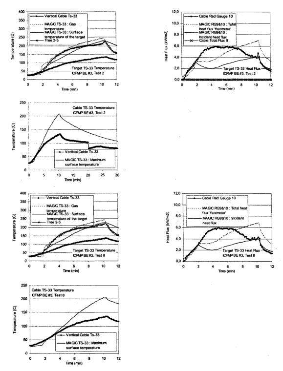
Figure A-61: Thermal Environment near Cable G, ICFMP BE #3, Tests 2 and 8
