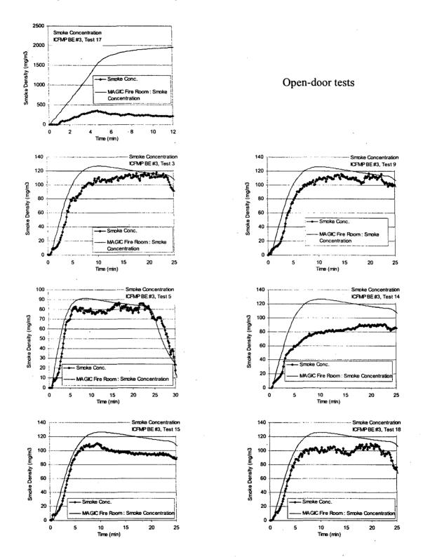
Figure A-33: Smoke Concentration in ICFMP BE #3, Open-Door Tests
