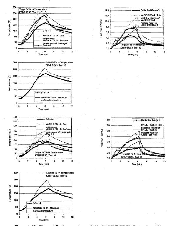
Figure A-39: Thermal Environment near Cable B, ICFMP BE #3, Tests 13 and 16
