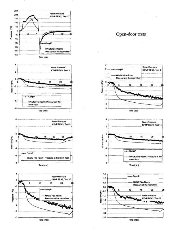
Figure A-35: Compartment Pressure in ICFMP BE #3, Open-Door Tests
