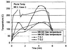
Figure A-22: Near-Ceiling Gas Temperatures, FM/SNL Series, Sectors 1 and 3
