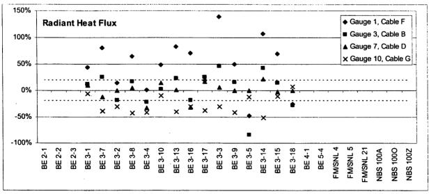
Figure 6-9: Scatter Plot of Relative Differences for Radiant Heat Flux in ICFMP BE #3 (Experimental uncertainty is 20%.)
