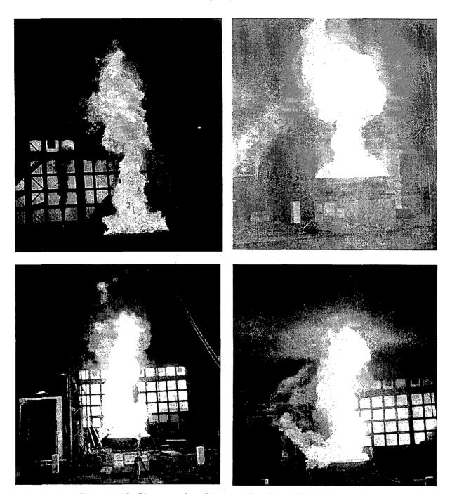
Figure A-25: Photographs of Heptane Pan Fires, ICFMP BE #2, Case 2 (Courtesy of Simo Hostikka, VTT Building and Transport, Espoo, Finland)
