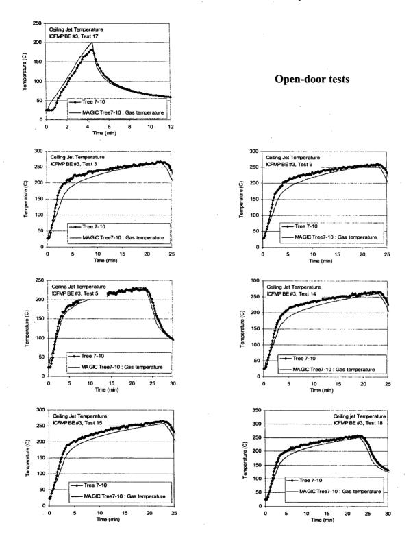
Figure A-19: Near-Ceiling Gas (Ceiling Jet) Temperatures, ICFMP BE #3, Open-Door Tests
