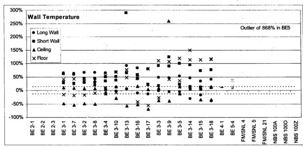
Figure 6-11: Scatter Plot of Relative Differences for Target Temperature in ICFMP BE #3, #4, and #5 (Experimental uncertainty is 14%.)
