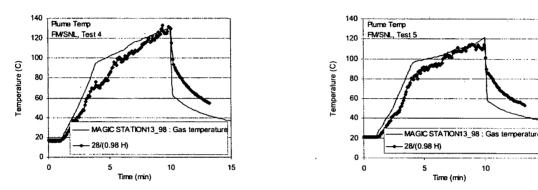
Figure A-23: Near-Plume Temperatures, FM/SNL Series, Sector 13
