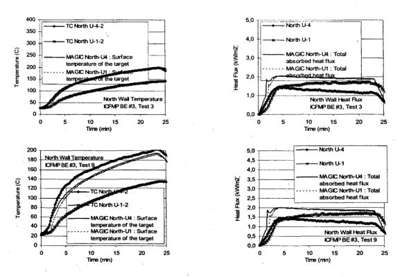
Figure A-72: Long-Wall Heat Flux and Surface Temperature, ICFMP BE #3, Closed- and Open-Door Tests
