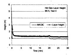
Figure A-11: Hot Gas Layer (HGL) Temperature and Height, ICFMP BE #5, Test 4
