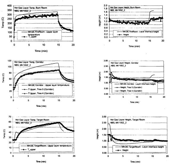
Figure A-17: Hot Gas Layer (HGL) Temperature and Height, NBS Multiroom Test 100Z
