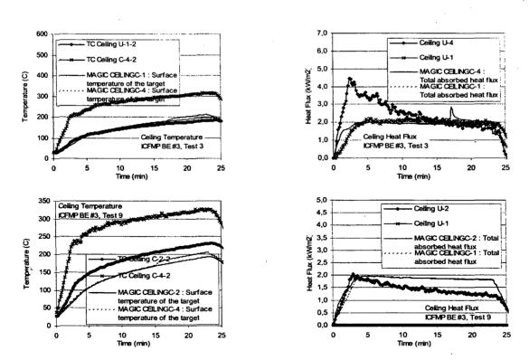
Figure A-80: Ceiling Heat Flux and Surface Temperature, ICFMP BE #3, Open-Door Tests
