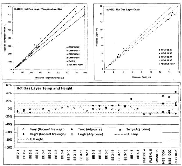
Figure 6-1: Scatter Plot of Relative Differences for Hot Gas Layer Temperature and Height in ICFMP BE #2, #3, #4, and #5, and the Selected FM/SNL and NBS Tests [Experimental uncertainties (EU) are 13% (HGL temp) and 9% (HGL height).]
