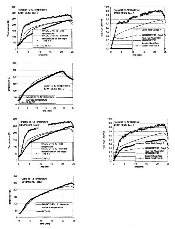
Figure A-49: Thermal Environment near Cable D, ICFMP BE #3, Tests 3 and 9
