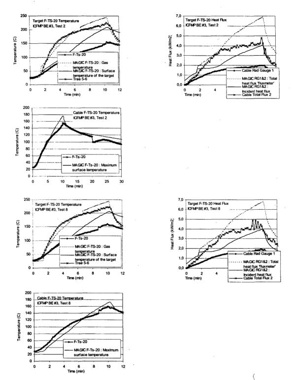
Figure A-53: Thermal Environment near Cable F, ICFMP BE #3, Tests 2 and 8
