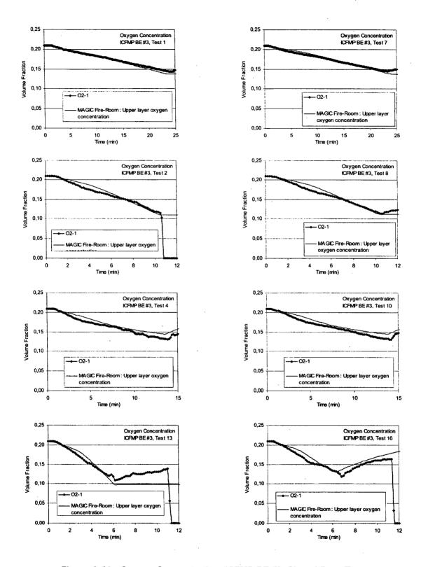
Figure A-29: Oxygen Concentration, ICFMP BE #3, Closed-Door Tests
