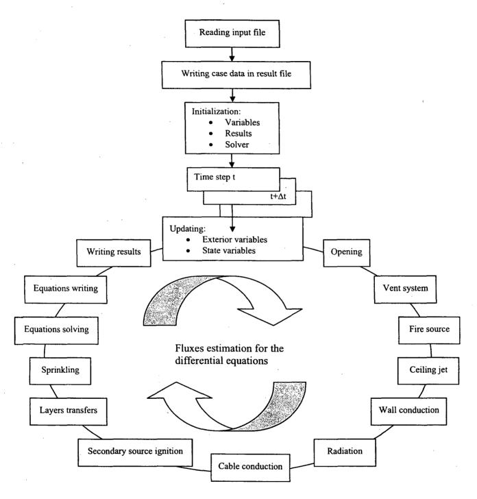
Figure 4-1: Simplified Functional Breakdown of the MAGIC Code
