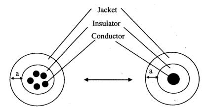
Figure 3-3: Modeling Multi-Conductor Cables in MAGIC
