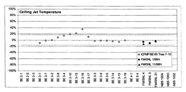
Figure 6-2: Scatter Plot of Relative Differences for Ceiling Jet Temperatures in ICFMP BE #3 and the Selected FM/SNL Tests (Experimental uncertainty is 16%.)
