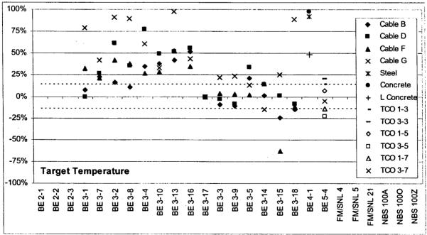
Figure 6-7: Scatter Plot of Relative Differences for Target Temperature in ICFMP BE #3 (Experimental uncertainty is 14%.)
