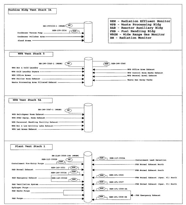
Figure 3.2 Schematic of Airborne Effluent Release Points
