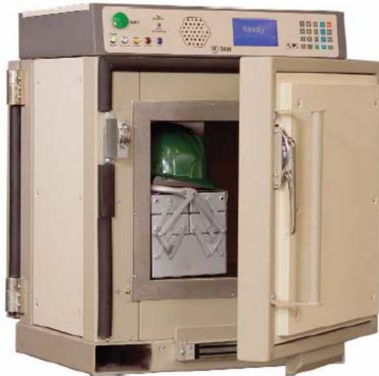
Figure D.1 Example Volumetric Counter (Thermo 2005)
