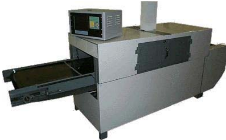
426 Figure D.2 Example Conveyorized Survey Monitoring System (Laurus 2001)
