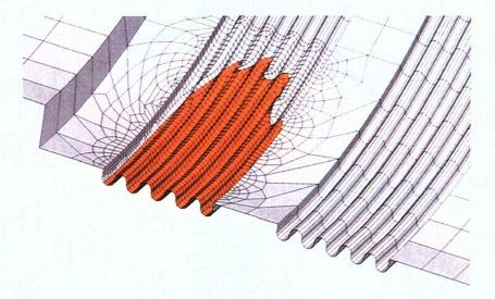
Figure 4.16: Mesh Detail of Corroded Bellows Area
