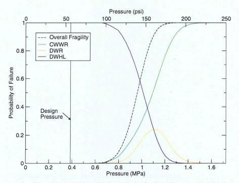
Figure 4.31: Conditional Probabilities of Failure Modes for Containment with 25% Corrosion at Wetwell Water Line
