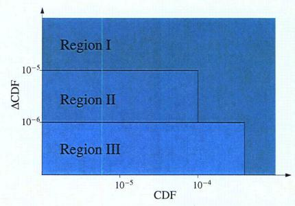
Figure 2.1: Acceptance Guidelines for Core Damage Frequency
