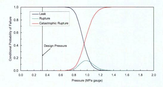
Figure 6.14: Conditional Probability of Failure for Original Containment (No Corrosion)
