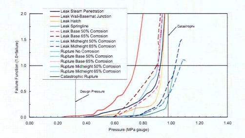
Figure 6.5: Failure Potential at Liner Corrosion and Discontinuity Locations
