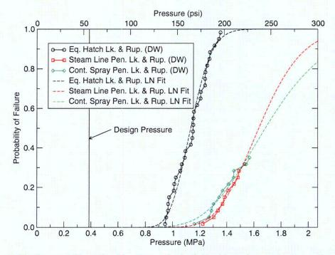
Figure 4.20: Raw and Fitted Fragility Curves for Individual Locations in the Drywell Region (Note: No Observed Failures at Floor Drain Penetration)
