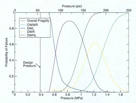
Figure 4.29: Conditional Probabilities of Failure Modes for Containment with 25% Corrosion at Drywell Sand Pocket
