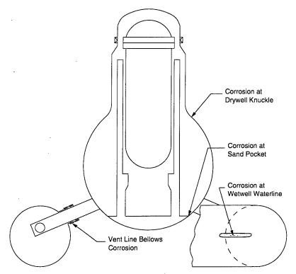
Figure 4.1: Postulated Corrosion in Liner of Steel Mark I Containment
