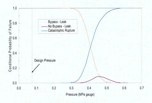
Figure 5.19: Conditional Probabilities for 50% Corrosion at the Basemat
