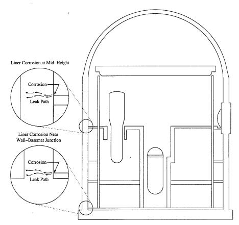
Figure 3.1: Postulated Corrosion in Liner of RC Containment
