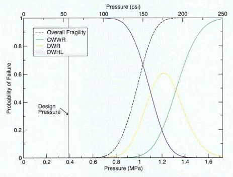
Figure 4.26: Conditional Probabilities of Failure Modes for Original Containment
