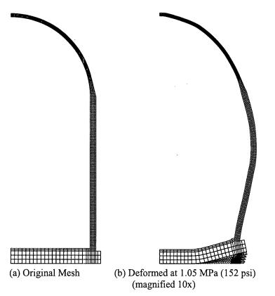
Figure 3.2: Axisymmetric Finite Element Model of RC Containment
