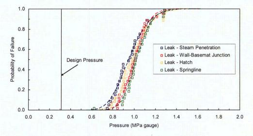
Figure 3.6: Fragility Curves for Leak at Discontinuity Locations
