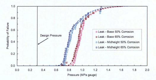
Figure 3.7: Fragility Curves for Leak at Corroded Locations
