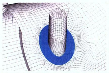
Figure 4.7: Mesh Detail of Wetwell Access Hatch Area
