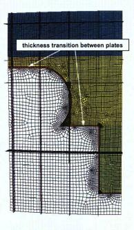
Figure 5.8: Detailed View of the Upper Containment Region Submodel
