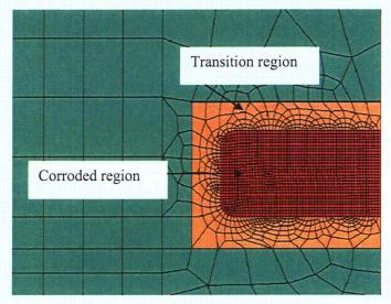
Figure 6.4: Corroded Region in Submodel Finite Element Mesh
