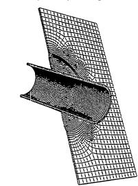
Figure 4.10: Containment Spray Line Penetration Submodel
