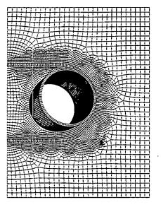
Figure 4.8: Steam Line Penetration Submodel
