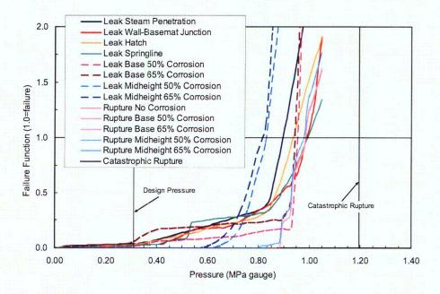
Figure 3.5: Failure Potential at Corrosion and Discontinuity Locations
