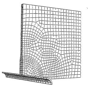
Figure 4.11: Wetwell Instrumentation Line Penetration Submodel
