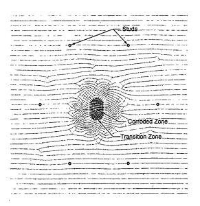
Figure 3.3: Finite Element Mesh of Corrosion at Midheight
