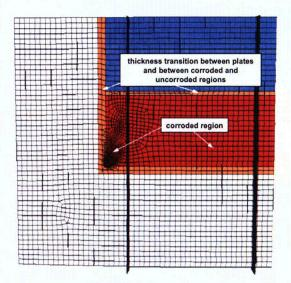
Figure 5.12: Detailed View of the Corroded Upper Floor Region Submodel
