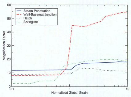
Figure 2.9: Strain Magnification Factors for Typical Discontinuities in RC Containments (Tang et al., 1995). Permission to use this copyrighted material is granted by Elsevier.
