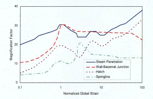
Figure 2.10: Strain Magnification Factors for Typical Discontinuities in Prestressed Containments (Tang et al., 1995). Permission to use this copyrighted material is granted by Elsevier.
