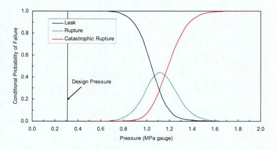
Figure 3.13: Conditional Probability of Failure for 65% Corrosion at Basemat
