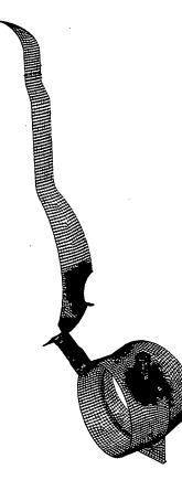
Figure 4.5: Finite Element Mesh of Containment with Large Penetrations
