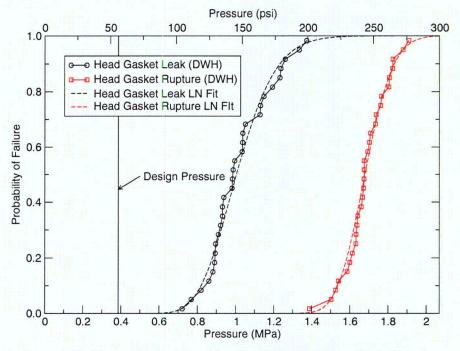
Figure 4.19: Raw and Fitted Fragility Curves for the Drywell Head Region
