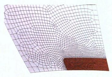
Figure 4.14: Mesh Detail of Corroded Area at Sand Pocket
