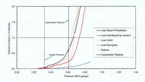
Figure 6.6: Failure Potential at Discontinuity Locations for 50% Area Degradation in the Midheight Tendons
