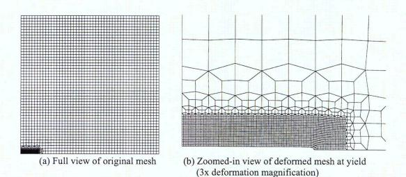
Figure 2.4: Finite Element Mesh of Plate with 5.08 m (200 in) Crack
