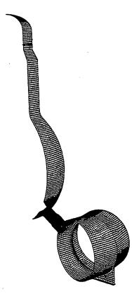
Figure 4.2: Finite Element Mesh of Drywell, Vent Line, and Wetwell
