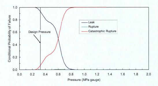
Figure 6.19: Conditional Probability of Failure for 50% Area Reduction of the Midheight Tendons
