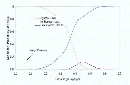
Figure 5.20: Conditional Probabilities for 25% Corrosion at the Basemat
