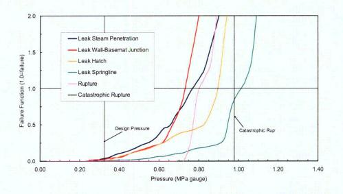
Figure 6.7: Failure Potential at Discontinuity Locations for 50% Loss of Prestressing of the Midheight Tendons
