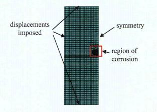
Figure 6.3: Submodel Finite Element Mesh
