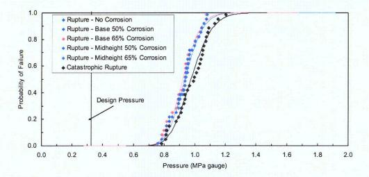
Figure 6.10: Fragility Curves for Rupture and Catastrophic Rupture
