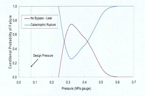
Figure 5.25: Conditional Probabilities for Bellows Corrosion
