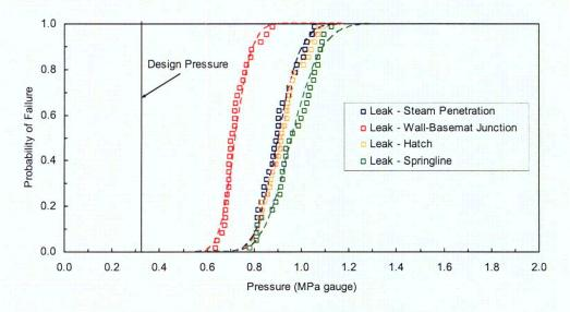
Figure 6.8: Fragility Curves for Leak at Discontinuity Locations
