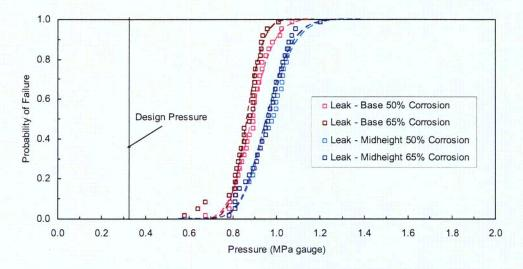
Figure 6.9: Fragility Curves for Leak at Corroded Locations
