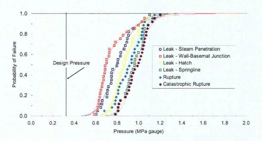
Figure 6.12: Fragility Curves for 50% Prestressing Loss for the Midheight Tendons
