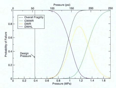
Figure 4.27: Conditional Probabilities of Failure Modes for Containment with 25% Corrosion at Drywell Knuckle
