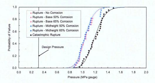
Figure 3.8: Fragility Curves for Rupture and Catastrophic Rupture
