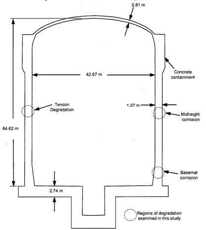
Figure 6.1: Postulated Degradation in Prestressed Concrete Containment
