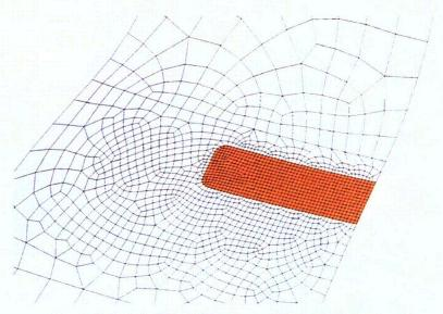
Figure 4.13: Mesh Detail of Drywell Knuckle Corrosion Area
