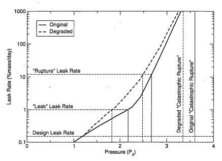
Figure 2.3: Hypothesized Effect of Degradation on Containment Performance
