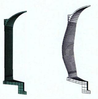
(a) Original Mesh(b) Deformed at 1.08 MPa (157 psi)Figure 6.2: 3-D Wedge Finite Element Model of Prestressed Containment
