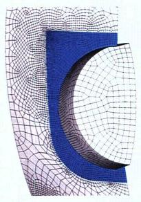
Figure 4.6: Mesh Detail of Equipment Hatch Area
