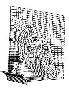
Figure 4.12: Wetwell HPCI Test Line Penetration Submodel
