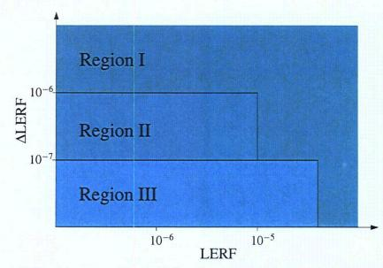
Figure 2.2: Acceptance Guidelines for Large Early Release Frequency
