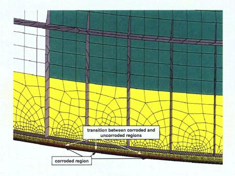
Figure 5.10: Detailed View of the Corroded Basemat Region
