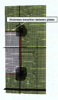
Figure 5.6: Detailed View of the Ice Basket Region Submodel
