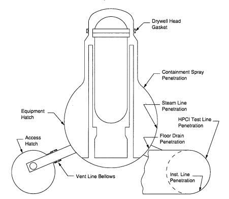
Figure 4.4: Approximate Locations of Local Details Analyzed in Steel Mark I Containment
