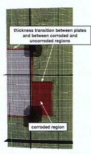
Figure 5.11: Detailed View of the Corroded Ice Basket Region Submodel
