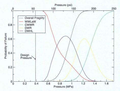
Figure 4.33: Conditional Probabilities of Failure Modes for Containment with Corrosion in One of Vent Line Bellows Plies
