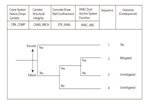
Figure B-1 Seismically Initiated Event Sequences.
