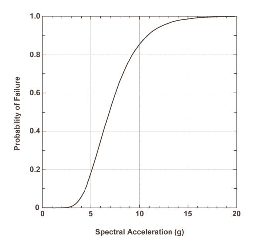
Figure A-2 Hypothetical Seismic Fragility Curve for Spectral Acceleration at 10-Hz.
