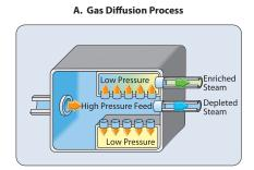
The gaseous diffusion method uses molecular diffusion to effect separation. The isotopic separation is accomplished by diffusing uranium, which has been combined with fluorine to form UF<sub>6</sub> gas, through a porous membrane (barrier) and utilizing the different molecular velocities of the two isotopes to achieve separation.
