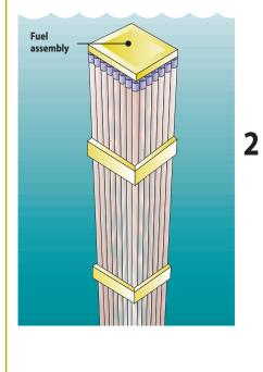
After about 6 years, spent fuel assemblies typically 14 feet long and containing nearly 200 fuel rods — are removed from the reactor and allowed to cool in storage pools for a few years. At this point, the 900-pound assemblies contain only about one-fifth the original amount of U<sup>235</sup>.
