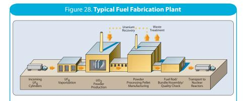
Fabrication is the final step in the process used to produce uranium fuel. It begins with the conversion of enriched uranium hexafluoride (UF<sub>6</sub>) gas to a uranium dioxide solid. Nuclear fuel must maintain both its chemical and physical properties under the extreme conditions of heat and radiation present inside an operating reactor vessel. Fabrication of commercial light-water reactor fuel consists of three basic steps:
