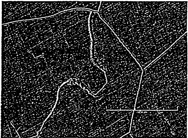
Figure 1. Typical microstructures observed by SEM, showing degree of sensitization for alloys used in this study: (a), (c), (e), low magnification; (b), (d), (f), high magnification.
