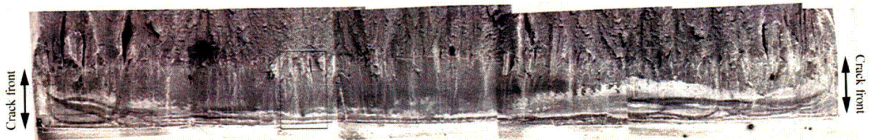
Figure 86. Photomicrograph of the fracture surface of specimen CT31-W01.
