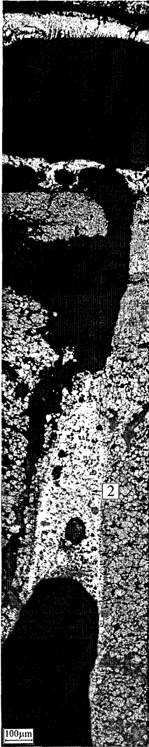
Fig. G-11.3. Fuel Microstructure for Fragment of Fuel Rod #B11T at 50 mm Elevation
