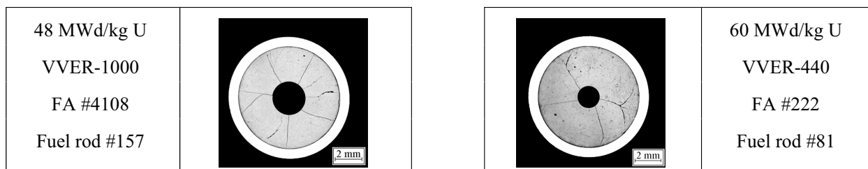
Fig. 5.14. The cross-sections of two VVER-1000 and VVER-440 high burnup fuel elements after the base irradiation
