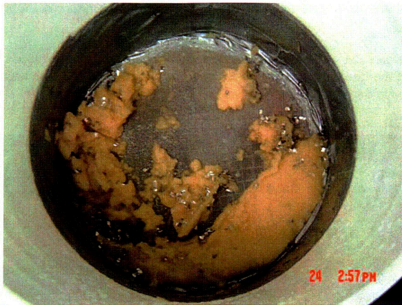
Figure 2-20. Debris Recovery Bucket after a Test Involving a Mixture of RMI and NUKON
