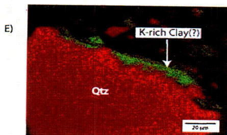
Combined X-ray map of Al (green) and Si (red) to better depict the relative location of clay(?) and quartz. This phase distribution is typical for the Naturita soil.
