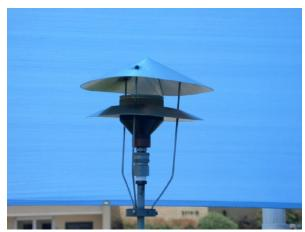
Device for monitoring airborne radiation
