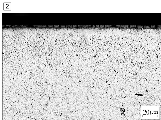
Fig.E-9.3. Cladding microstructure at 69 mm elevation (from low cap) and longitudinal metallographic specimen image of fuel rod # RT9
