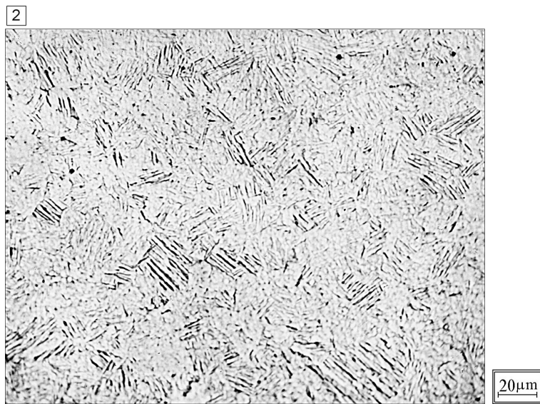
Fig.E-8.4. Cladding microstructure of fuel rod # RT8 at 97 mm elevation (from low cap)
