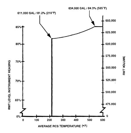
FIGURE 3.5.5-1 Minimum Required RWT Volume
