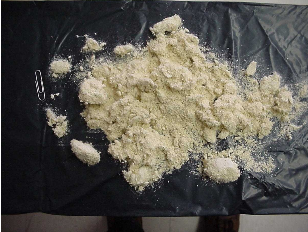
Figure 3-3. Prototypical crushed CalSil debris.
