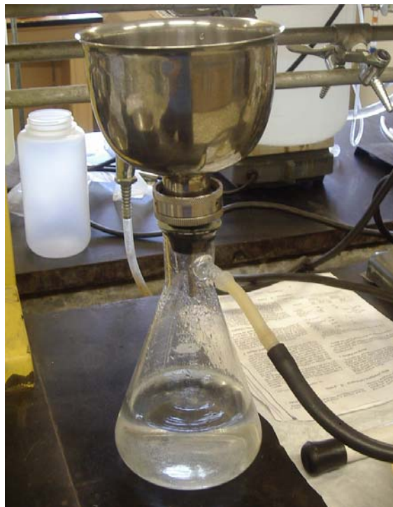
Figure 4-1. Filtration of NUKON™ to remove water.
