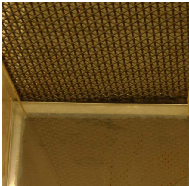
Figure 2-5b. Close-up of the 0.64-cm (0.25-in.)-opening screen and tray on the floor.
