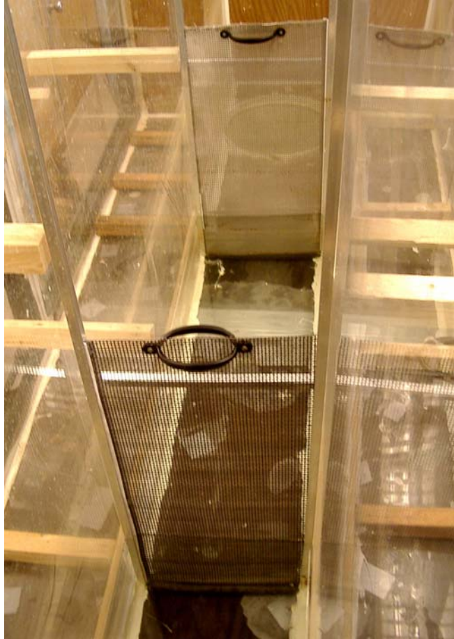
Figure 2-5a. Test screen and fine screen in the test section.
