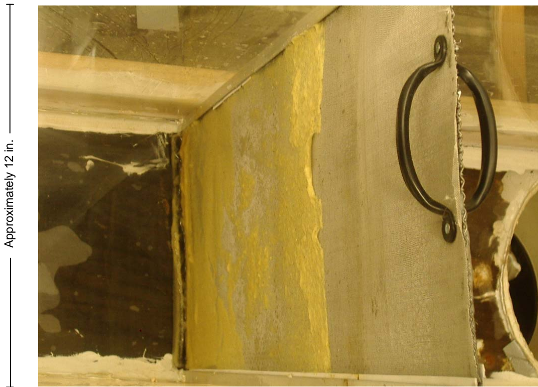
Figure 5-3. Finer-sized BP NUKON™ collected on the fine screen located downstream.
