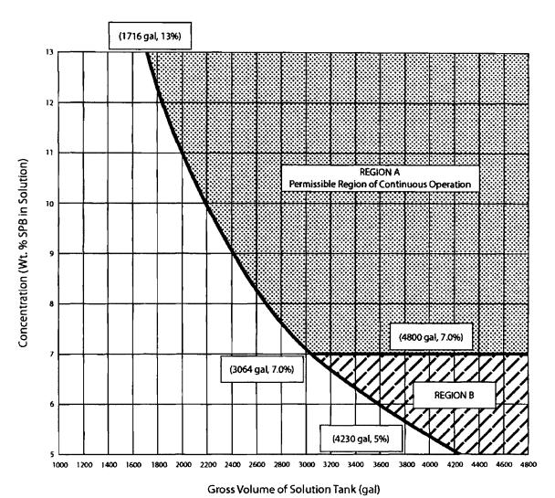
Figure 3.1.7-1 (page 1 of 1) Sodium Pentaborate Solution Volume Versus Concentration Requirements
