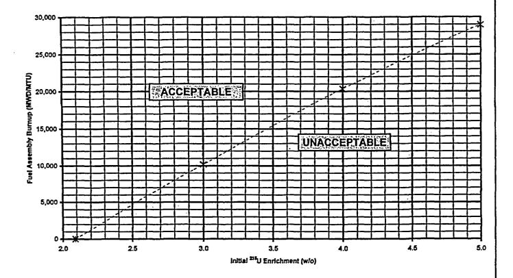
Figure 3.7.18-1 Fuel Assembly Burnup Limit Requirements For Cask Storage
