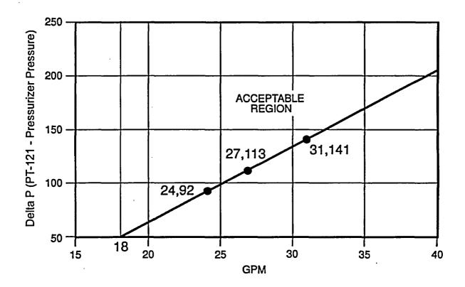
Figure 3.5.5-1 Seal Injection Flow Limits
