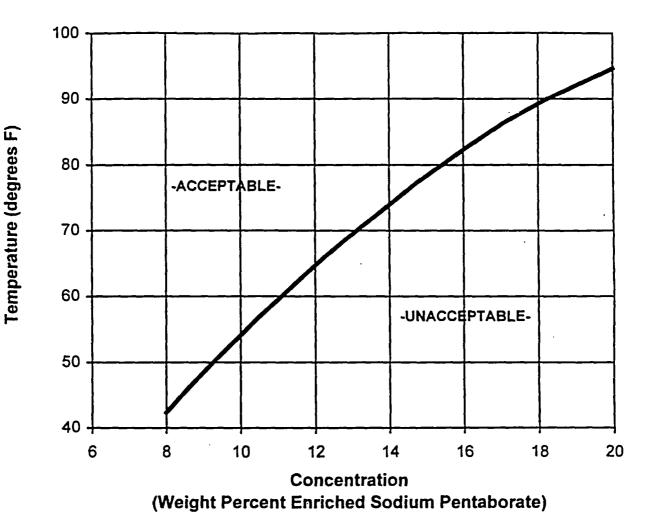
Figure 3.1.7-2 (page 1 of 1) Sodium Pentaborate Solution Temperature Versus Concentration Requirements
