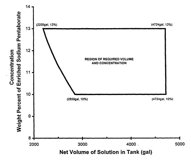
Figure 3.1.7-1 (page 1 of 1) Sodium Pentaborate Solution Volume Versus Concentration Requirements
