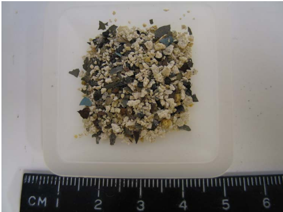
Fig. 16. Particulate 500 \mu m to 2 mm (Plant C).
