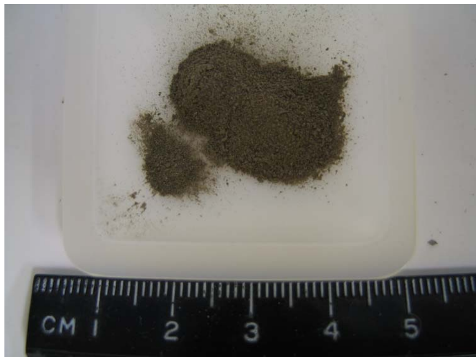
Fig. 8. Particulate <75 \mu\text{m} (Plant A).
