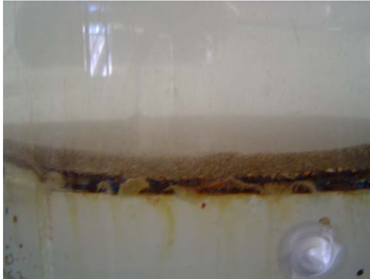
Fig. 51. Test 16 debris bed of common sand.
