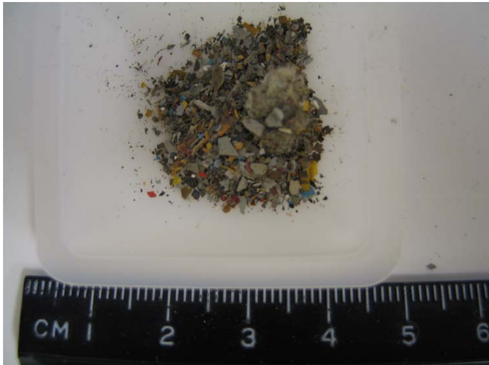
Fig. 6. Particulate 500 \mu m to 2 mm (Plant A).
