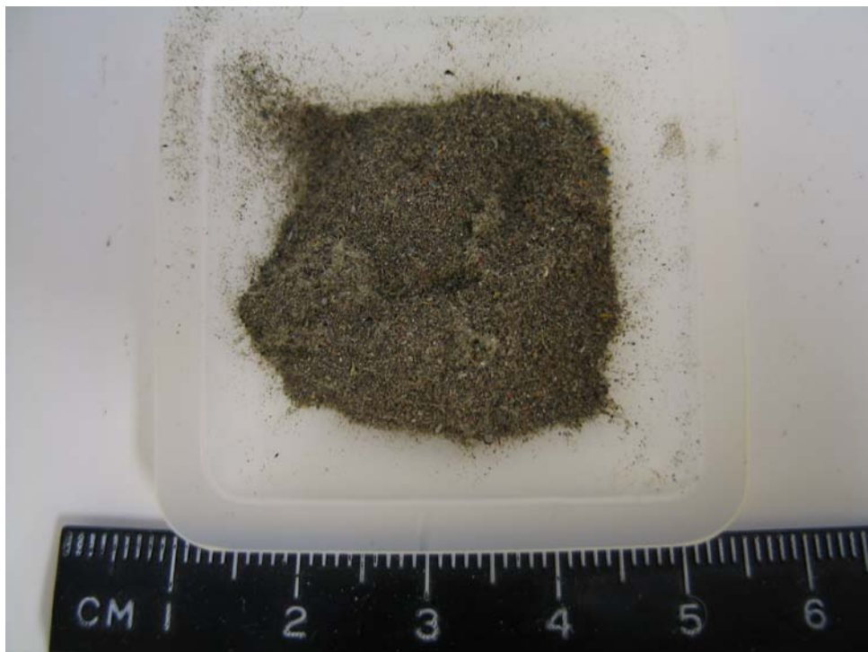
Fig. 7. Particulate 75 \mu\text{m} to 500 \mu\text{m} (Plant A).
