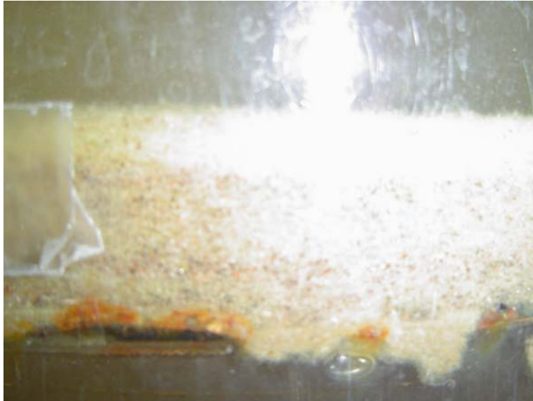
Fig. 53. Test 20 debris bed of NUKON™ mixed with common sand.
