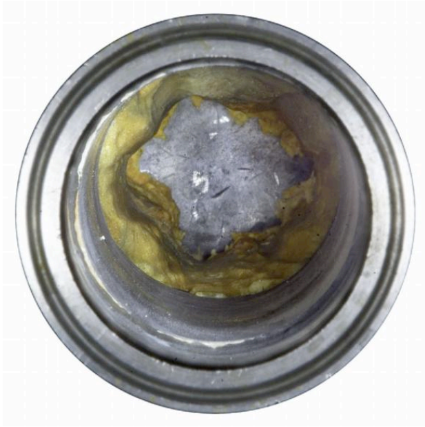
Figure 25. Photograph of the solid boric acid crust left at the bottom of the test chamber after the corrosion test with water addition.
