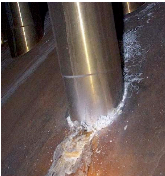
Figure 4. Deposits of boric acid crystals on reactor pressure vessel head from leaking CRDM nozzles.
