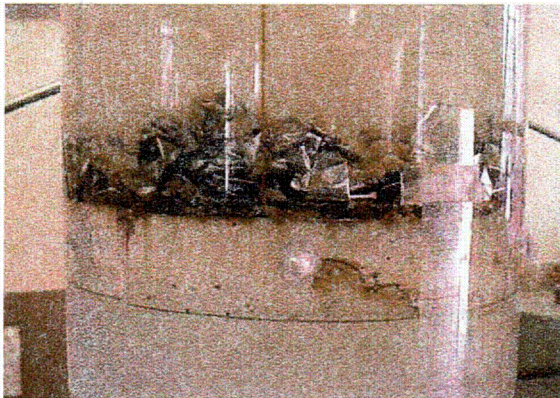
Figure 3.24. CalSil/RMI debris mixture in a typical 1-in. debris bed.
