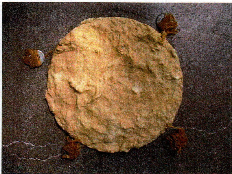
Figure 4.7. Photo of Test 31 debris bed.
