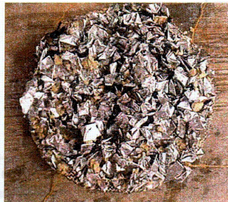
Figure 3.24. CalSil/RMI debris mixture in a typical 1-in. debris bed.
