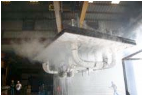
#111: Immediately after hose stream test.
