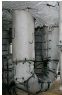
#124: Item 3J after hose stream test.
