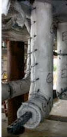
#121: Item 3G after hose stream test.
