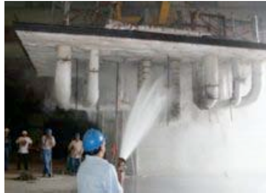
#110: Hose stream test.
