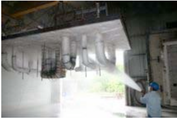
#109: Hose stream test.
