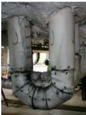
#125: Item 3J after hose stream test.
