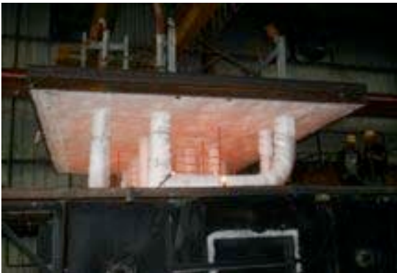
#95: Removing assembly from furnace.
