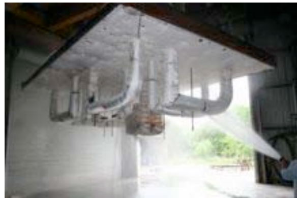
#108: Hose stream test @ 15°, 75 psi from 10 feet.
