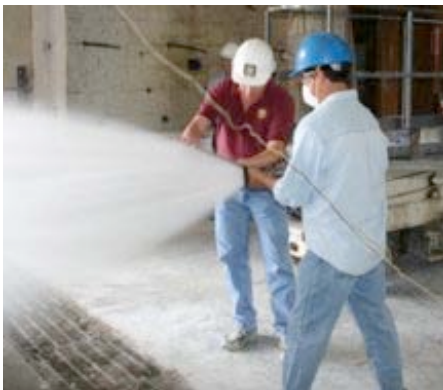
#107: Setting water pressure and discharge angle.
