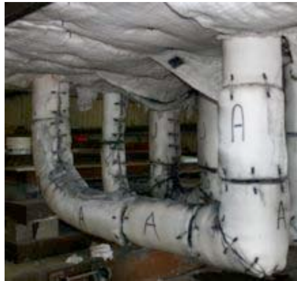
#114: Item 3A after hose stream test.
